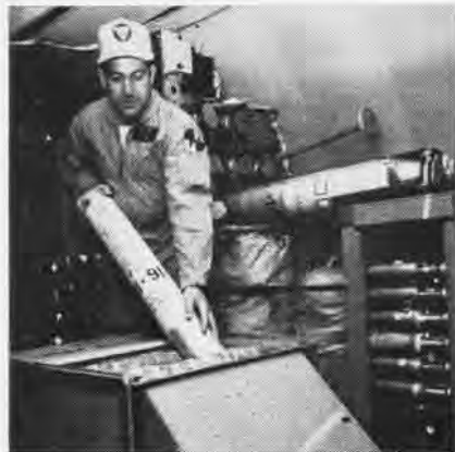
L. G. HONSINGER, AO2, loads smoke marker into retro-launcher aboard the P-3 Orion.
