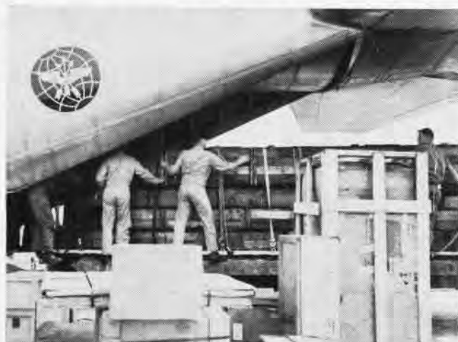
OFFLOADING CARGO sometimes is an all-crew job. Some 1400 pounds of cargo are strapped to three pallets tied together and rolled off.
