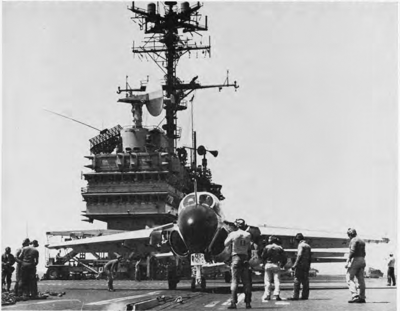
A GRUMMAN A-6A INTRUDER FLOWN BY VA-75 PILOT PREPARES TO LAUNCH FROM THE SARATOGA. NOSE TOW SHUTTLE IN FOREGROUND
