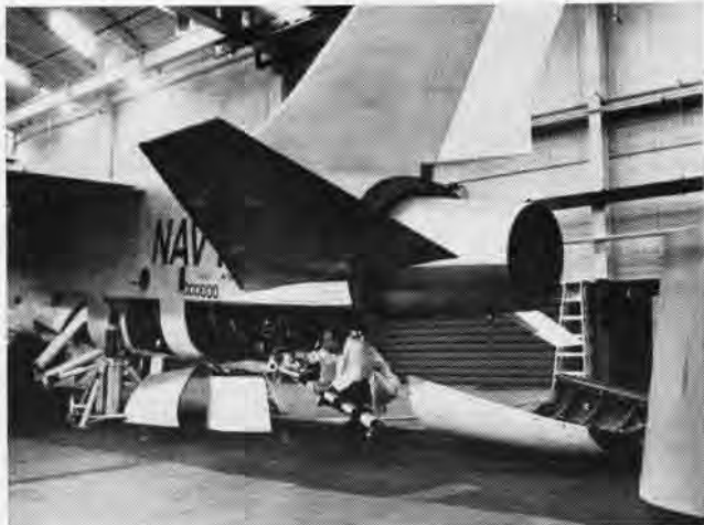
EASE OF REMOVAL of the jet engine without removing the plane's tail section is demonstrated in this photo of the full-scale A-7A mockup.
