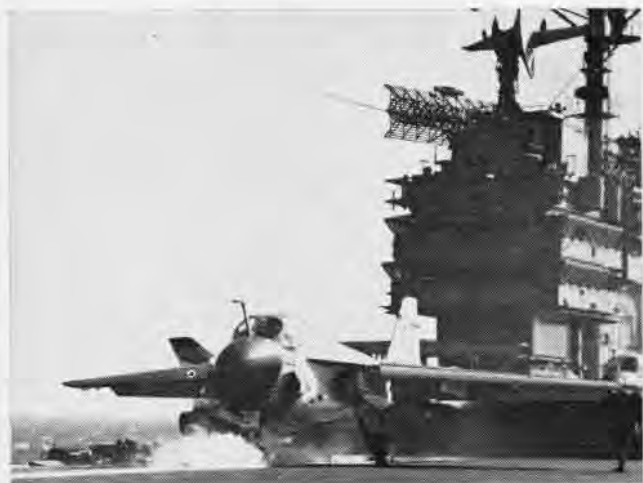
STEAM HIDES THE MECHANICAL HOOK-UP OF CATAPULT TO PLANE
