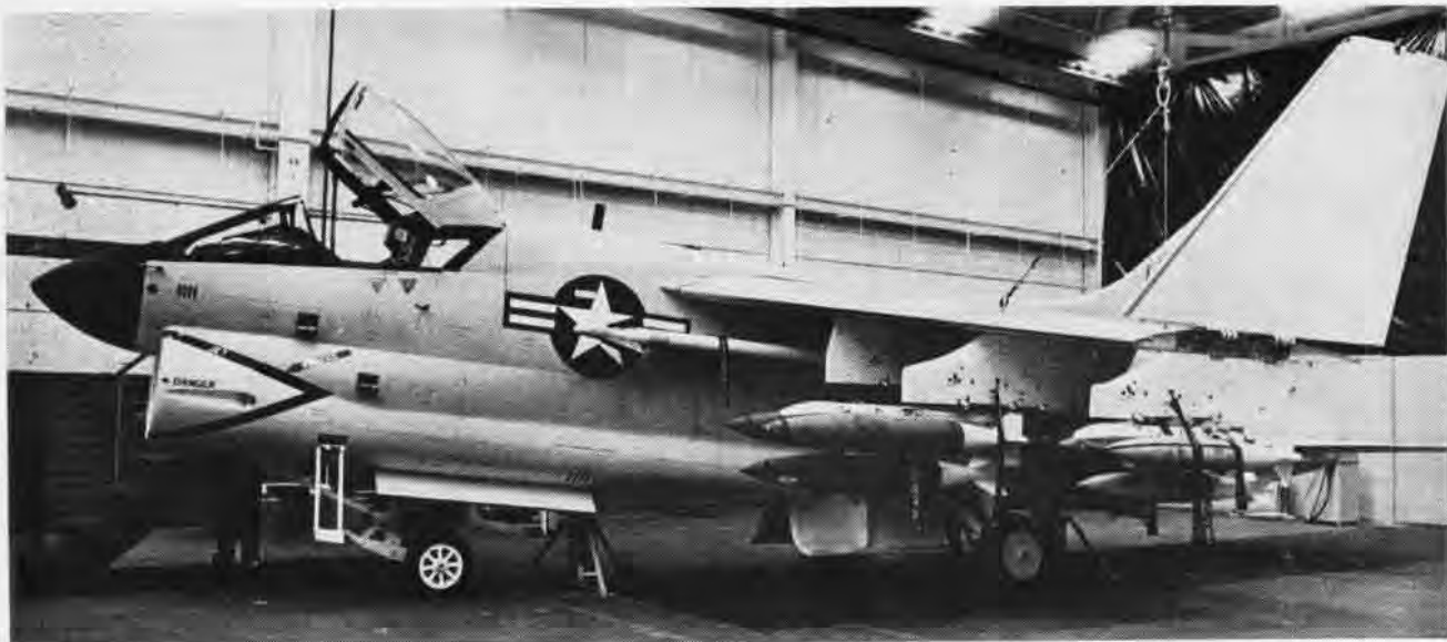
SIDE VIEW of full-scale mockup of the A-7A attack bomber Ling-Temco-Vought is building for the Navy shows the aircraft carrying a variety of bombs on two of its wing pylons and a Sidewinder missile on the fuselage. The aircraft, formerly called VAL, has 20 mm cannon.
