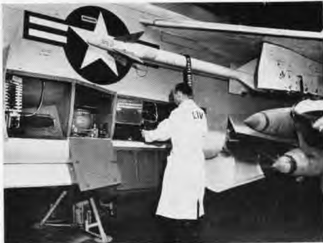
MAINTENANCE technicians have easy access to numerous areas in the forward section of the A-7A. The gun bay, opened, appears at the left.
