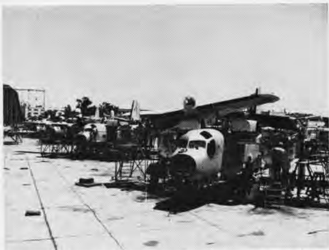
TRACKERS undergo PAR at North Island's O&R open-air production line. Twenty to 24 planes are being processed at all times in Area H.
