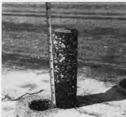
THIS CORE SAMPLE, drilled from a runway at Beaufort, is nine and a half inches long.
