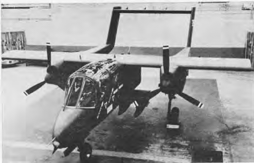
TWIN-TURBOPROPS , twin booms, horizontal tail high between vertical tails mark OV-10A. Under-wing fuselage gives pilot and observer in tandem, ahead of props, an unobstructed view.
