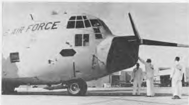
NICKNAMED the "Humanitarian Dragonfly" this HC-130H Hercules and many others will operate on a global basis in mid-1965. The USAF's Air Rescue Service will use the new version for distress missions. Probes on nose extend in flight to snare balloon-lifted lines for personnel and material pickup. Radome houses tracking gear.
