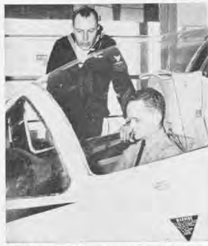
PILOT IS checked out in an aircraft by means of a Cockpit Orientation Trainer (COT).
