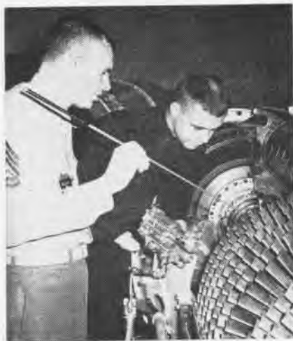
INSTRUCTOR POINTS out workings of J-57 engine to University of Wisconsin midshipman.
