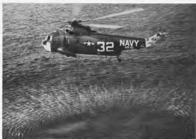
THE ULTIMATE in aerial maneuverability belongs to the SH-3A Sea King as its crew pinpoints "enemy submarine" with dipping sonar.
