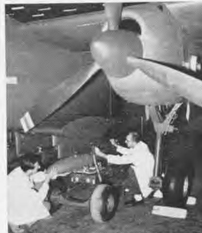
LOCATION of store stations permits loading of weapons without special hoist equipment.
