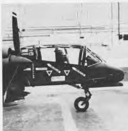
SIDE VIEW of the OV-10A illustrates the unobstructed visibility available to crewmen.
