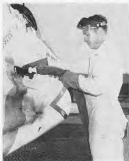
LOX IN JETS changes to gas, goes through 14 feet of tubing, is then warmed for pilot.
