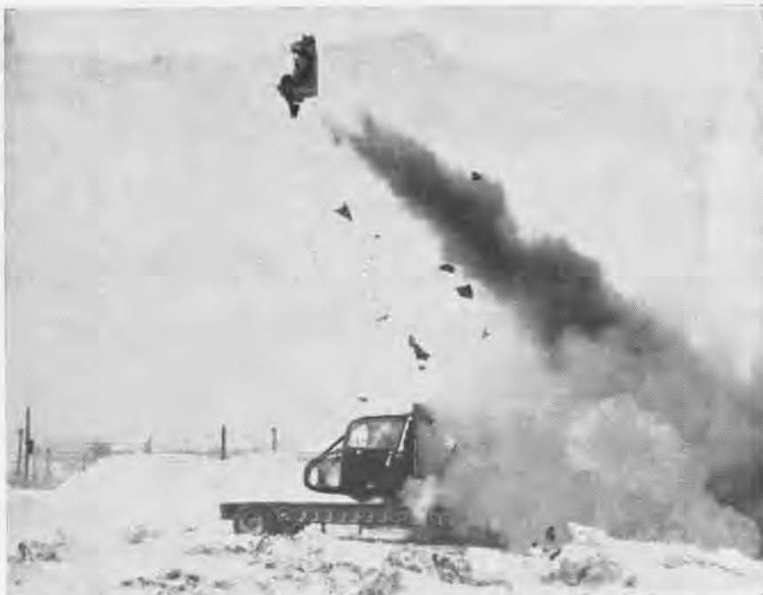
SMOKE AND PIECES OF PLASTIC from a shattered canopy fill the air as a dummy rides a rocket-propelled seat in a successful test of the X-22A vertical/short takeoff and landing (V/STOL) aircraft's emergency ejection system. Two dummies of varying weight were separately ejected up through the aircraft's plastic canopy by a 1250-pound thrust rocket attached to the seat. They reached altitudes of 200 and 500 feet before their parachutes opened up.
