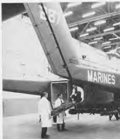
REAR SEAT removed, OV-10A can accommodate a medical attendant and two litter cases.
