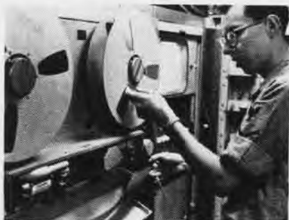
A NEW ROLL of magnetic tape is threaded on video tape recorder by Phillip Cano, IC3.
