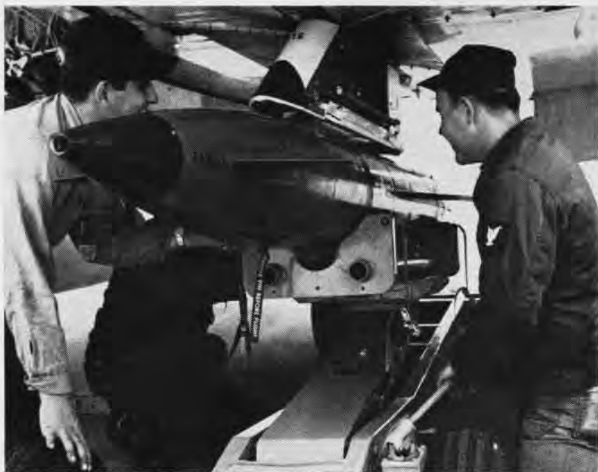
MISSILE TECHNICIANS of Guided Missile Unit 55 at Naval Missile Center, Point Mugu, California, load an AQM-37 target missile aboard a Skyhawk for airborne test and evaluation.
