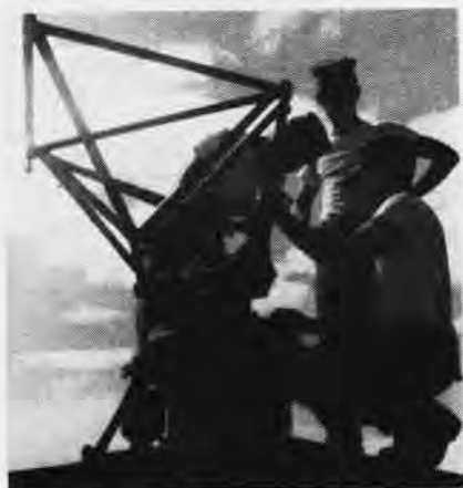
BASE for a search antenna is mounted atop radar van. It will scan for enemy aircraft.
