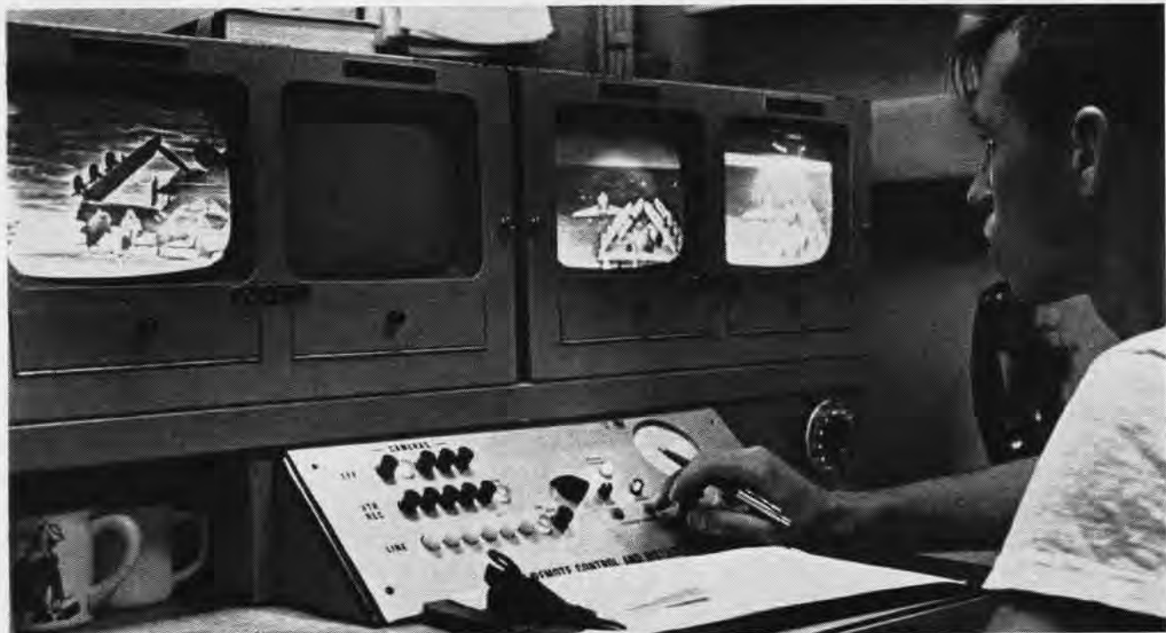
AT THE REMOTE control console, Gerald D. Clark, ICFN, selects camera positions to be relayed to the closed-circuit TV receivers placed in squadron ready rooms, on the bridge, and on the LSO platform aboard Bon Homme Richard . The system is known as PLAT.
