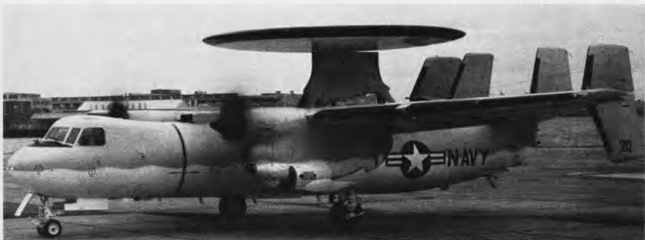
MAKING ITS FIRST appearance with VAW-11 on the West Coast, the Grumman E-2A Hawkeye is designed to revolutionize airborne early warning with its completely computerized data-link system. The Hawkeye is capable of operating at 30,000 feet.
