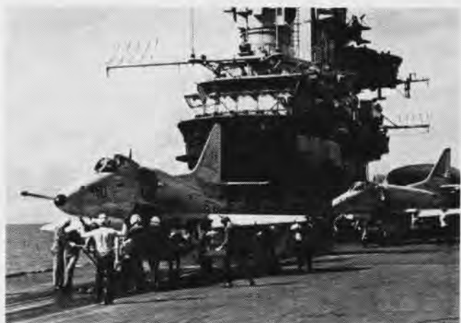
CATAPULT CREW lines up VA-164 A-4 Skyhawk for launch from Oriskany's flight deck. Squadron underwent first combat in May.
