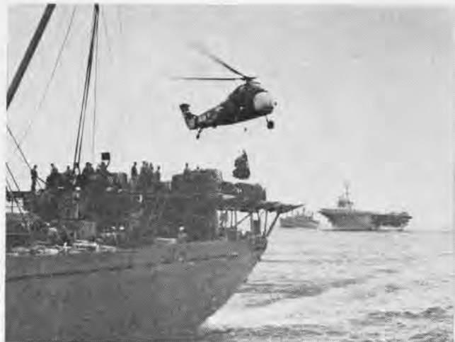
HELO MAKES a pick-up of cargo for delivery to CVA in background. Under ideal conditions, a round trip is accomplished in 30 seconds.
