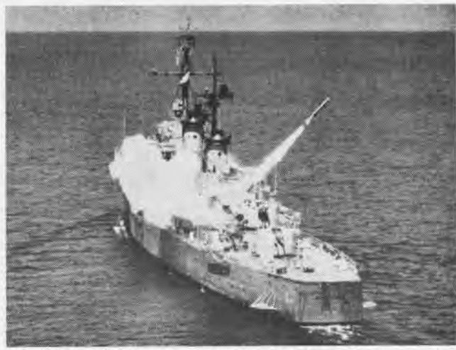
ASROC , with a Mark 46 payload, is launched from a destroyer in test. Once in water, the torpedo pursues its target using search patterns.
