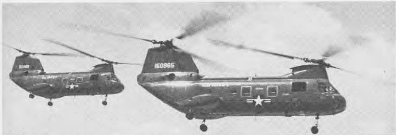
BOEING VERTOL UH-46A Sea Knight was assigned to new supply ships for use in vertical replenishment of combatant ships while under-
