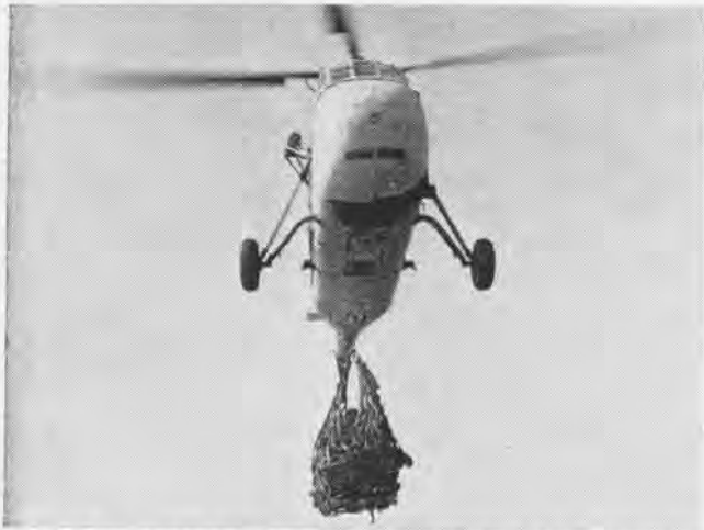
ALTAIR HELICOPTER brings empty nets and pallets to the supply ship. All nets and pallets are returned every five to ten round trips.
