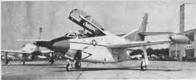
TWIN-ENGINE version of the Buckeye, T-2B, was under evaluation by VT-4 at Pensacola prior to introduction in basic flight training.
