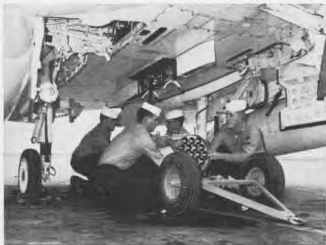
ORDNANCEMEN Peter Dickinson, Donald Hopkins, David Smith and Marlowe Gunderson, prepare to lift Aero 7D rocket pack into its place.
