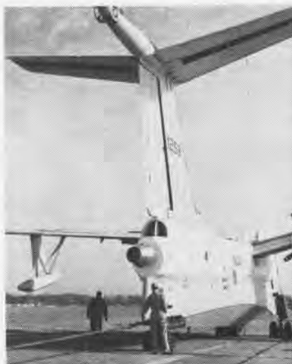
JET ENGINE in the tail, designed to give the SP-5B Marlin greater performance on takeoff as well as increased rate of climb, is being tested by Navy at Patuxent. The J-60 engine, which produces 3000 pounds of thrust, was installed in the tail observer's compartment by the Martin Company of Baltimore.
