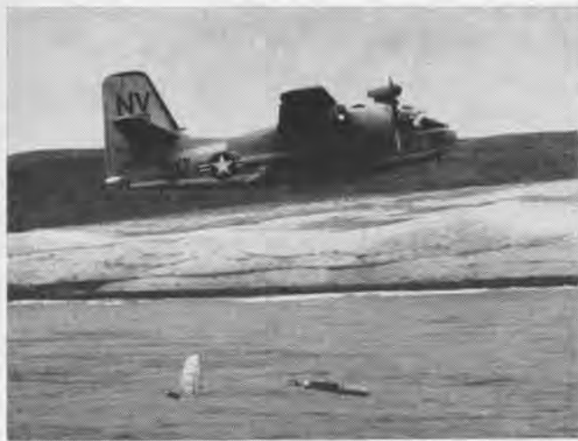
S-2 LAUNCHES Mark 46, the Navy's first solid-rocket-propellant-driven torpedo during operational test of weapon's capabilities.
