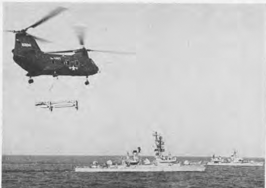
UH-46 TYPE HELOS , like this one toting a missile, will increase the lift capability of Vertrep and along with larger flight deck platforms, will further expedite supply replenishment.
