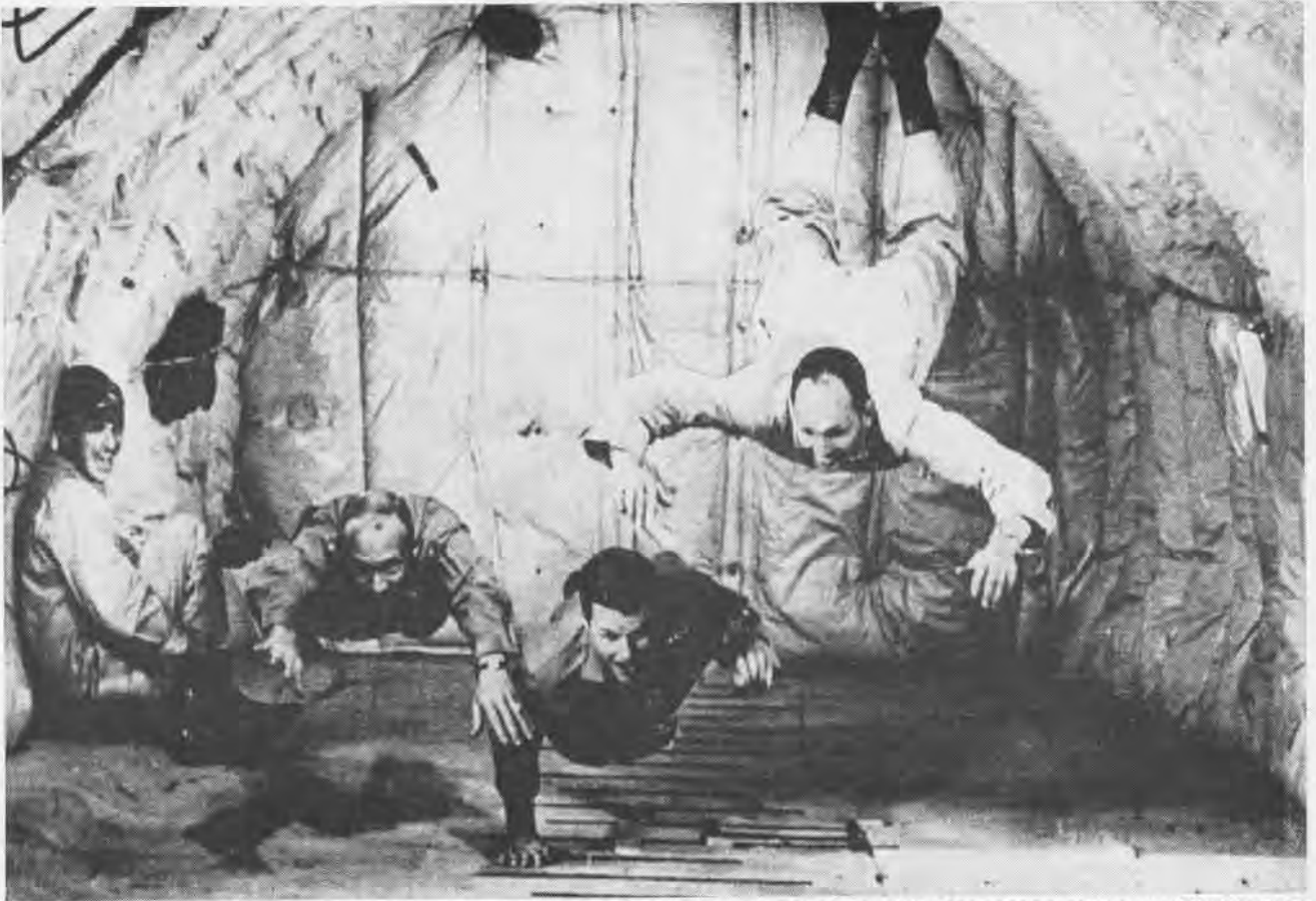
C-135 AIRCRAFT FOLLOWS PARABOLIC CURVE TO SIMULATE WEIGHTLESSNESS IN ORDER TO GIVE ASTRONAUTS SPECIAL INDOCTRINATION
