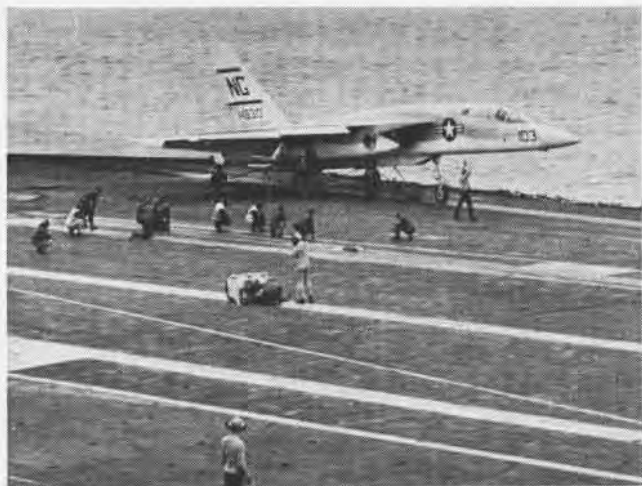
FLIGHT DECK CREWMEN on a waist catapult have booked up the bridle to "103" and crouch in readiness before pilot adds takeoff power.
