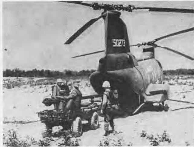
THE MEDIUM ASSAULT transport helicopter can carry a great deal of equipment; for example, a 106 recoilless rifle on an M-274 Mule.
