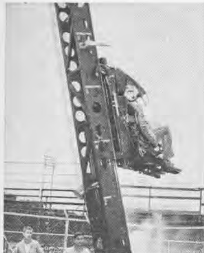
NAVY MEN get realistic sensations of ejection in this trainer designed at NTDC.
