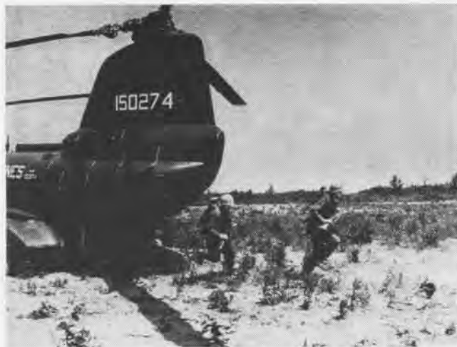
MARINES CHARGE out of the Sea Knight which carries 17 fully equipped troops on a 100-mile radius mission. It can carry up to 25 troops.
