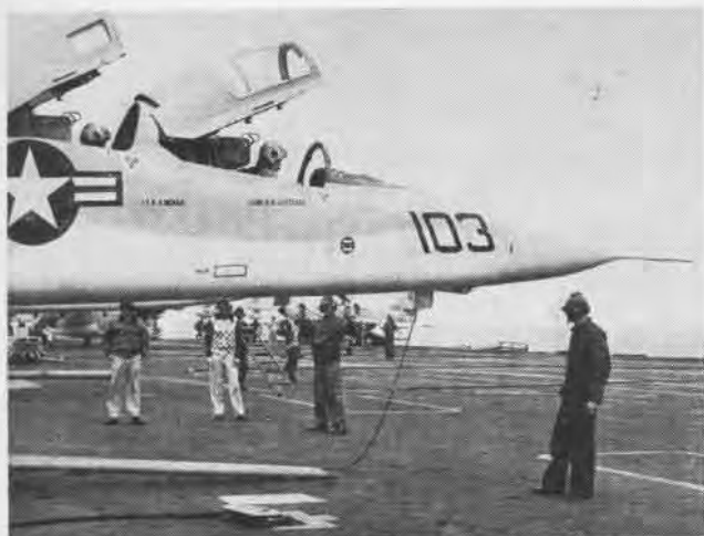
WITH EVERYTHING ready, it is time for the final steps to be taken; Vigilante 103 is "turned up" prior to position on the steam catapult.
