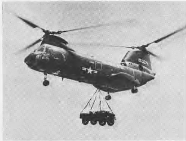
USING ITS EXTERNAL cargo hook, the CH-46A helicopter finds it no trick at all to lift and transport a 1700-pound Mighty Mite vehicle.
