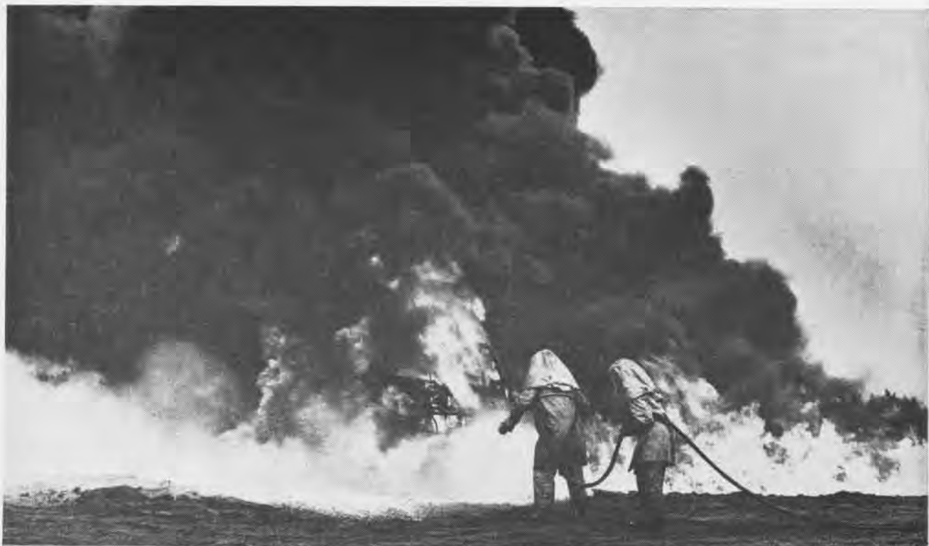
A BLAZING AIRCRAFT IS PUT OUT BY USING LIGHT WATER AND PURPLE K DEVELOPED BY THE NAVAL RESEARCH LABORATORY
