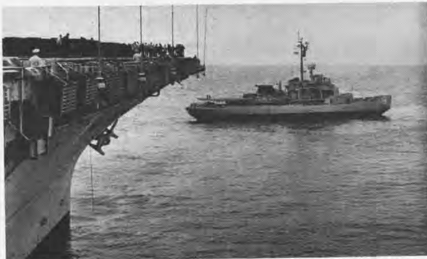
SEATTLE-BASED icebreaker USS Staten Island (AGB-5) displayed muscle power last fall off Oregon coast when she towed 71,000-ton Kitty Hawk for three hours, reaching a sustained speed of eight knots. Objective of exercise was to determine the ability of 6000-ton AGB-5
