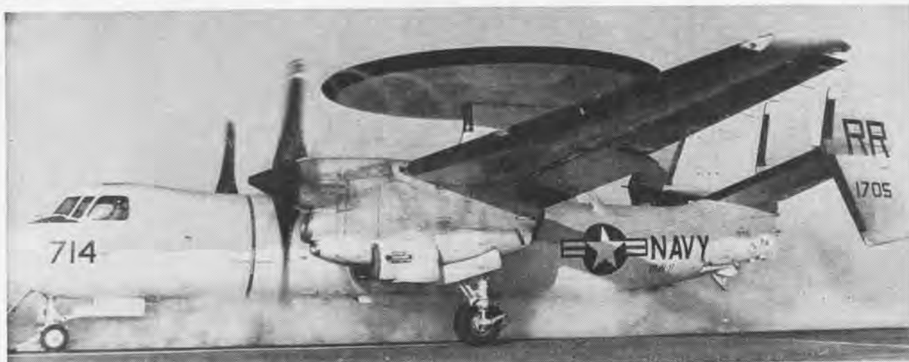
A GRUMMAN HAWKEYE is being launched from the flight deck of the USS Oriskany. The E-2A is 56 feet, 4 inches, in length and has a wing span of 80 feet, 7 inches. The two Allison turboprop power plants, which whirl reversible pitch propellers, generate 4600 horsepower each.
