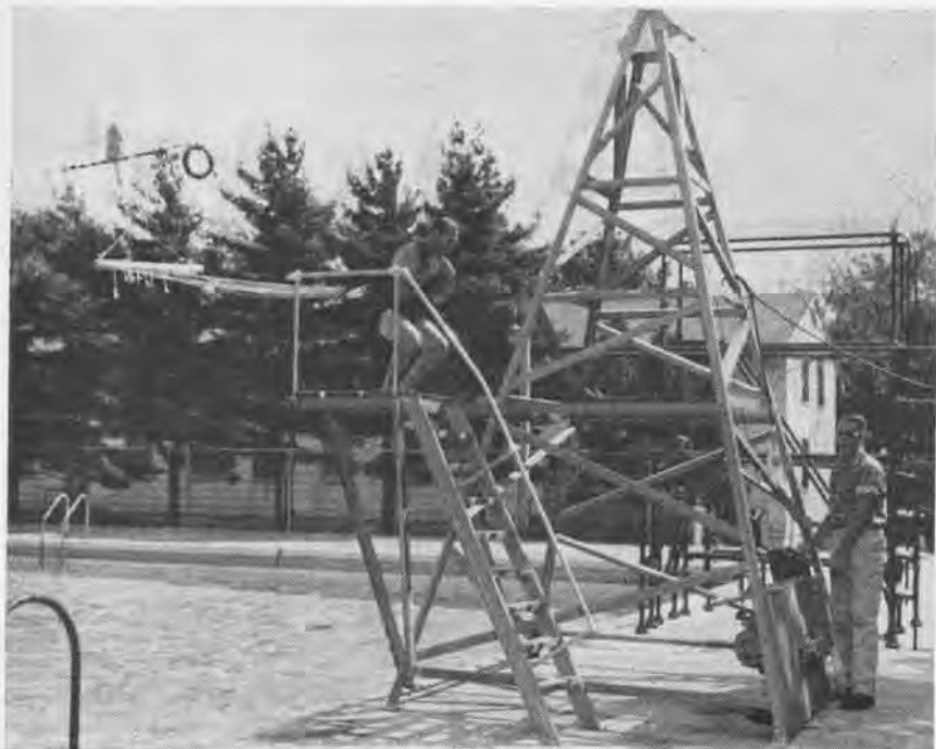
THIS TRAINING DEVICE yanks the student into the water and by means of a pulley drags him through a pool to simulate effects of a downed airman being hauled through ocean by a chute.
