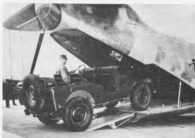
1966, reduce the pipeline time for delivery of cargo and personnel to carriers. Maximum loads are 15,000 lbs. of cargo or 40 passengers. Cruising speed is 300 mph; range, 1300 miles with five-ton payload. It has nose-tow launch feature and turboprop engines similar to Hawk-eye. Large rear-loading doors makes for easy loading of bulky cargo.
