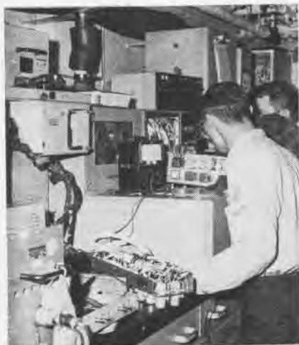
IN AVIONICS SHOP, the Program Bench tests all avionics components of the Vigilante.
