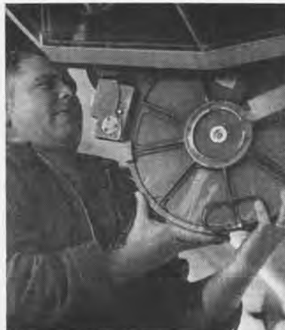
WHEN THE RA-5C is tied down, personnel open the "canoe" and take out the exposed film.
