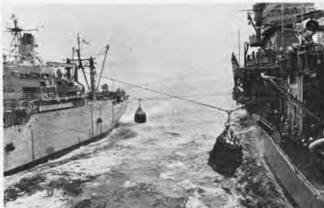
UNDERWAY REPLENISHMENT is one way of keeping an aircraft carrier supplied with items ranging from fresh vegetables to spare parts.
