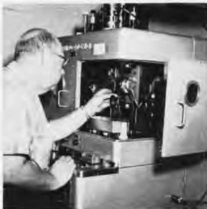
CHEMIST James Jennings places a vial containing oil in spectrometer for analysis.
