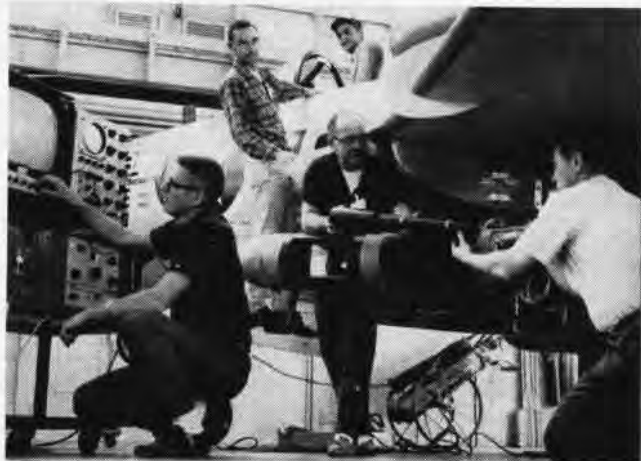
TELEVISION CAMERA and transmitter, mounted under the left wing of the QF-9G drone, receive special attention prior to the takeoff.
