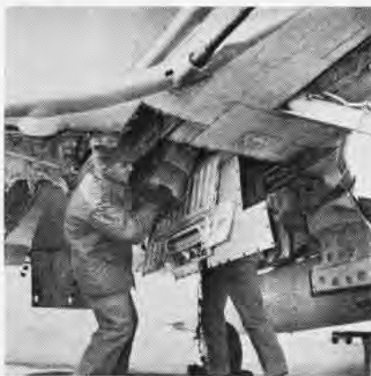
MARINES JOCKEY ammo cans into waiting A-4. Skyhawk fires through 20mm cannon.
