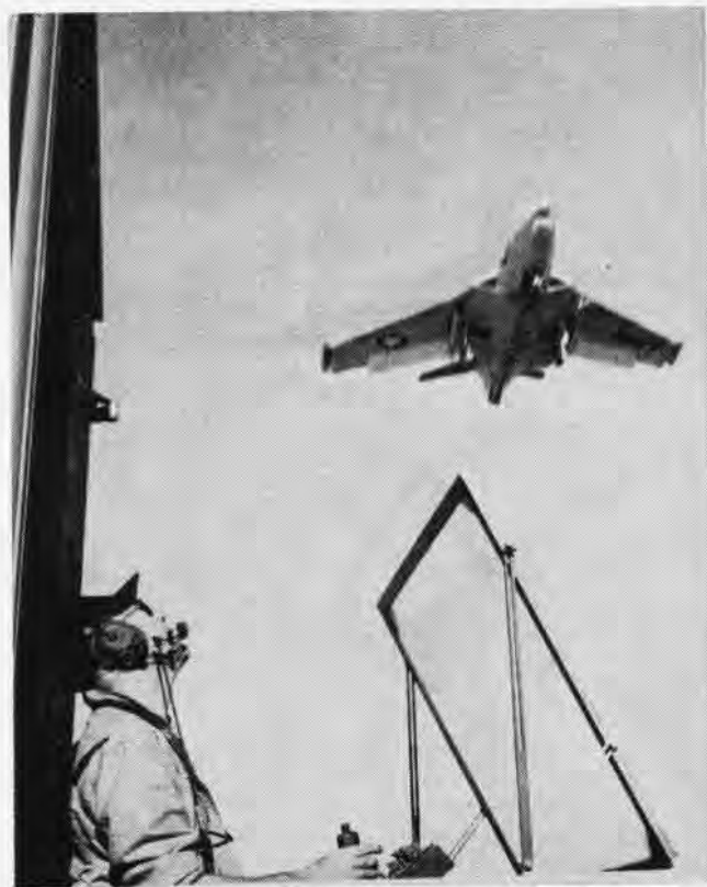
LAUNCH CONTROL officer, Lt. Todd Crombie, guides QF-9G on takeoff. After drone reaches proper altitude, chase planes take over.
