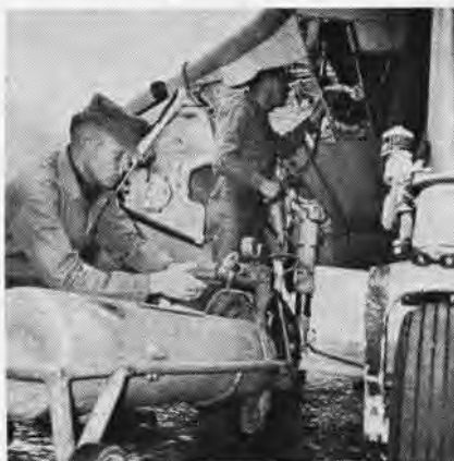
TWO MEMBERS of VMA-225's gun crew fill an A-4's pneumatic system with compressed air.
