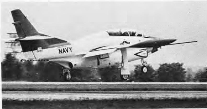
THE T-2B BUCKEYE jet trainer, scheduled for the Naval Air Basic Training Command, is shown returning from its first test flight at Columbus, Ohio. This is the first production model of 46 Buckeyes ordered by the Navy. The North American T-2B will replace the T-2A now in use. The new version has two 1-60 Pratt and Whitney jet engines which will substantially increase the power of the trainer to more than 6,000 pounds of available thrust.
