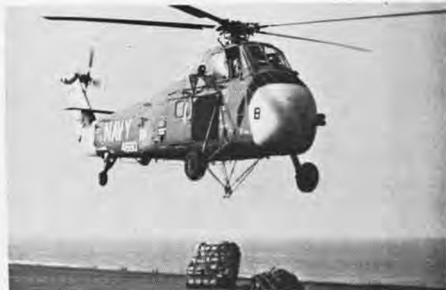
VERTICAL REPLENISHMENT speeds the transfer of supplies at sea. The belo remains airborne during operation, hovering to unload or load.
