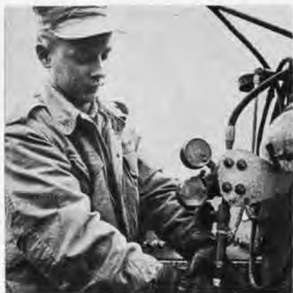
AIR BOTTLES used to pressurize A-4 pneumatic systems are filled by LCpl. Meister.
