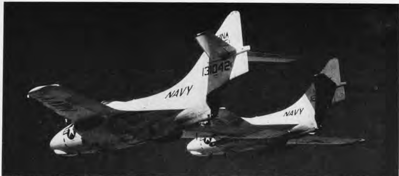
FIRST PHOTO of dual target presentation shows unmanned QF-9G drone aircraft in tight formation. Plane (right) with TV camera and transmitter under left wing relays relative position picture of "slave" to ground control station. Drones are controlled up to 75 miles.
