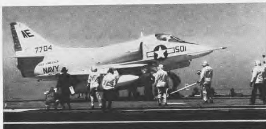
FLIGHT DECK CREWMEN aboard USS America hook up an A-4C Skyhawk to the catapult as the ship's Exec., Cdr. K. B. Austin, prepares to pilot the aircraft for first "cat" launch.
