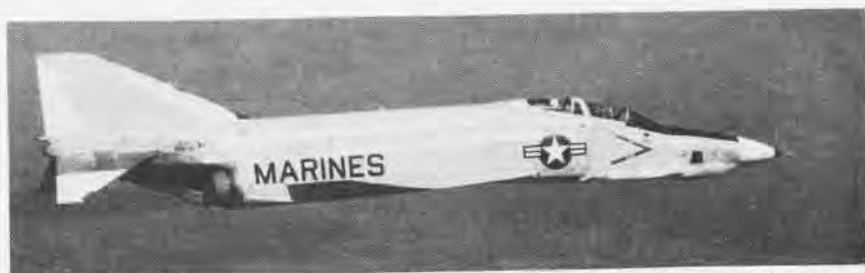
NEW PHOTO VERSION of the Phantom II, developed by the McDonnell Aircraft Corporation, is the RF-4B, now coming off production line for service with the Marines. Its first military test flight took place in April. The shore-based F-4C was developed for the USAF from the standard Navy/Marine F-4B, followed by the USAF RF-4C recon version. A minimum program combined the F-4B and RF-4C features into the RF-4B to meet Marine Corps needs.
