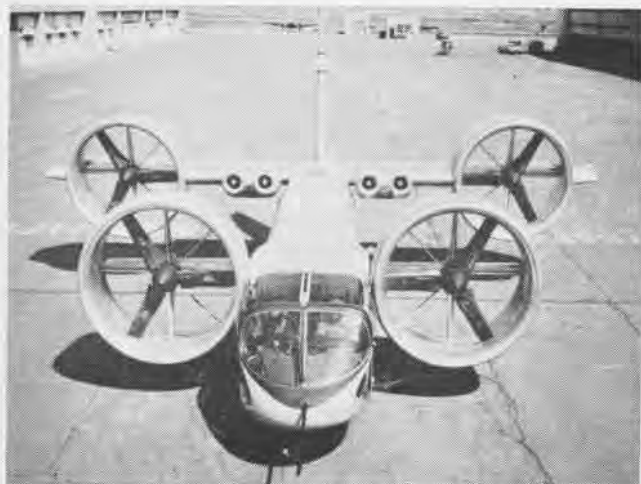
T-58 ENGINES DRIVE ALL PROPS THROUGH COMMON SHAFTING
