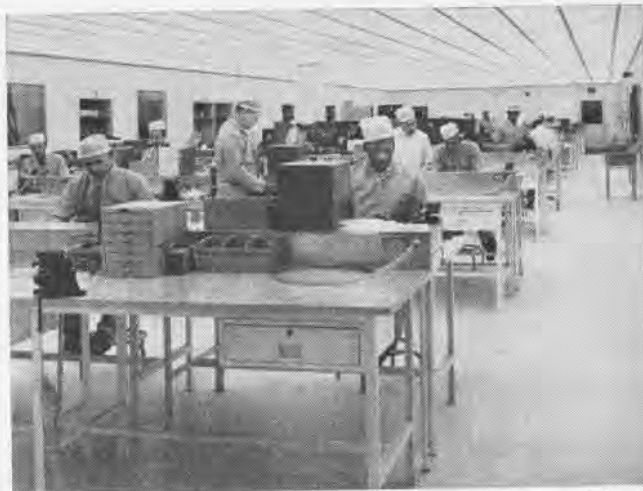
NEW ASSEMBLY AREA is largest contamination-free section of facility. Glass cabinets (left) are air-locked to protect transfer of parts.
