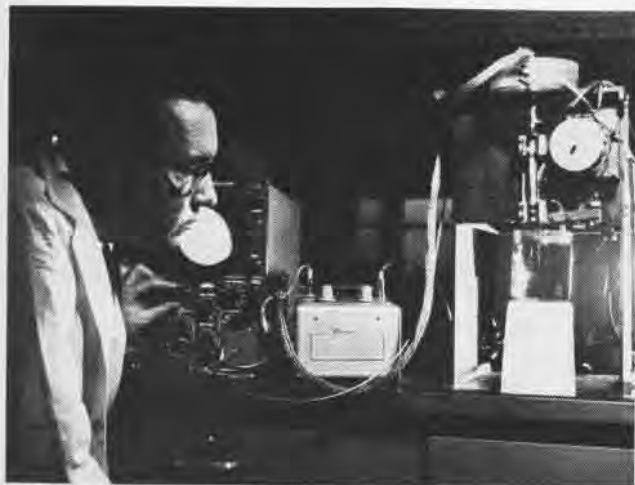
ROTOGENERATIVE MAPPING apparatus aids Illinois Institute of Technology in study of kinetics of inhibitive action of aircraft primer.
