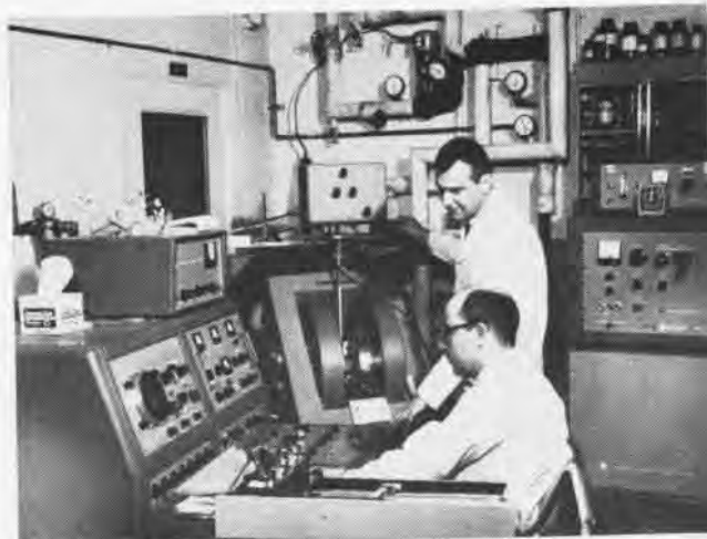
AT NAVAL RESEARCH Laboratory, Washington, scientists use electron spin resonance techniques to study magnesium alloy corrosion factors.
