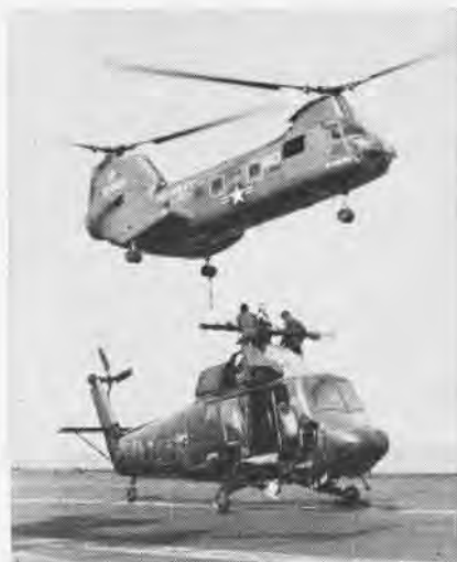
HELO-TO-HELO airlift removes downed craft from USS Ranger for needed repairs ashore.
