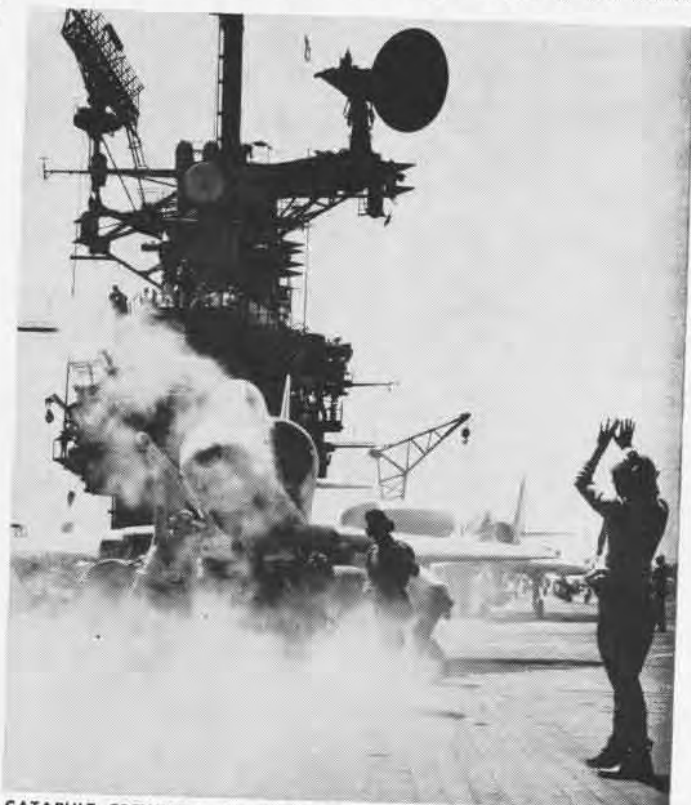
CATAPULT CREWMEN aboard USS Hancock attach a bridle to A-4 Skyhawk while steam pressure builds up for launch against North Vietnam.
