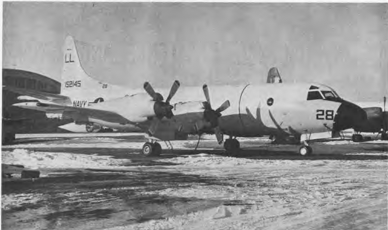
RECENT ADDITION to flight line of VP-38's Detachment Alfa at NAS Patuxent River is the Deltic P-3A. The aircraft's new Deltic system includes latest ASW detection devices which are more sensitive than earlier types and include improved tactical display equipment.
