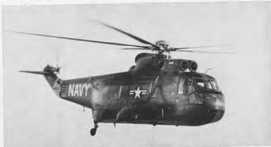
FOR ABOUT 9½ HOURS of the flight, the SH-3A was on single engine. The #2 engine was secured shortly after passing Guadalupe Pass, Tex., and started again 5,000 feet over Jacksonville.
