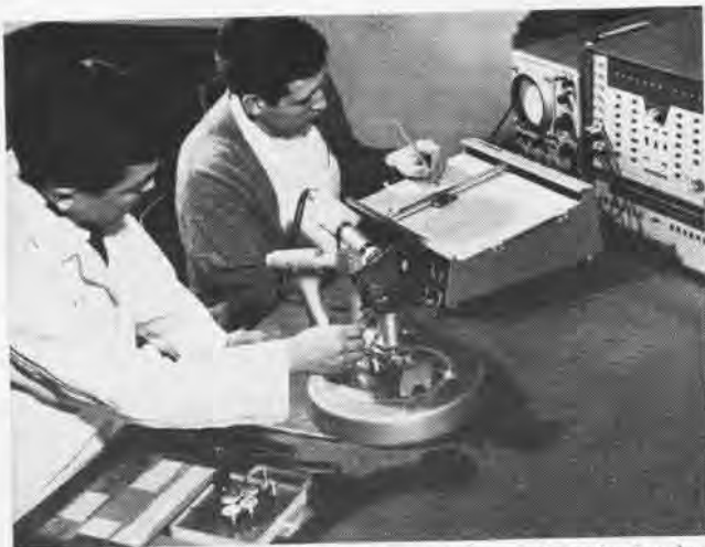
INDUSTRIAL NUCLEONICS Corporation engineers work to develop beta radiation equipment for the detection of corrosion under paint.
