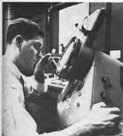
ALCOA TECHNICIAN inspects chemical conversion surface coating with electron microscope.
