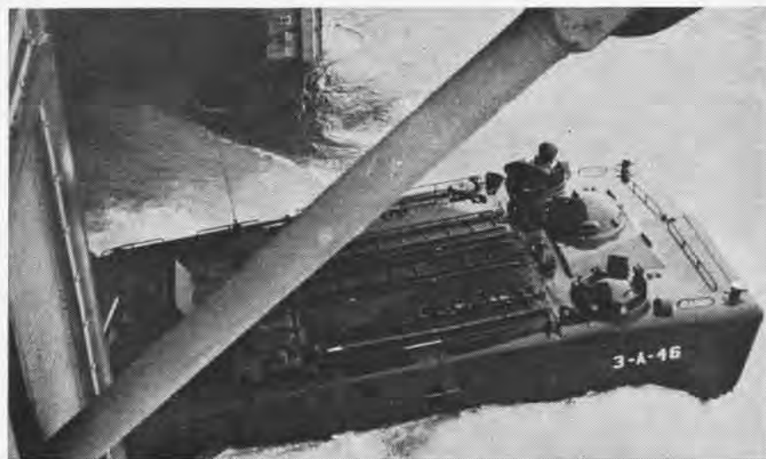
A MARINE LVTP-5 churns out of the tank deck of an LST before forming up in an assault wave. Part of a self-sustaining landing force, the vehicle has a capacity of 34 troops.
