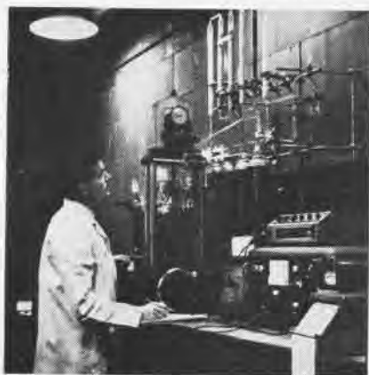
UNIVERSITY of Pennsylvania scientist studying the effect of stress on the permeation of electrolytic hydrogen in high strength steel.
