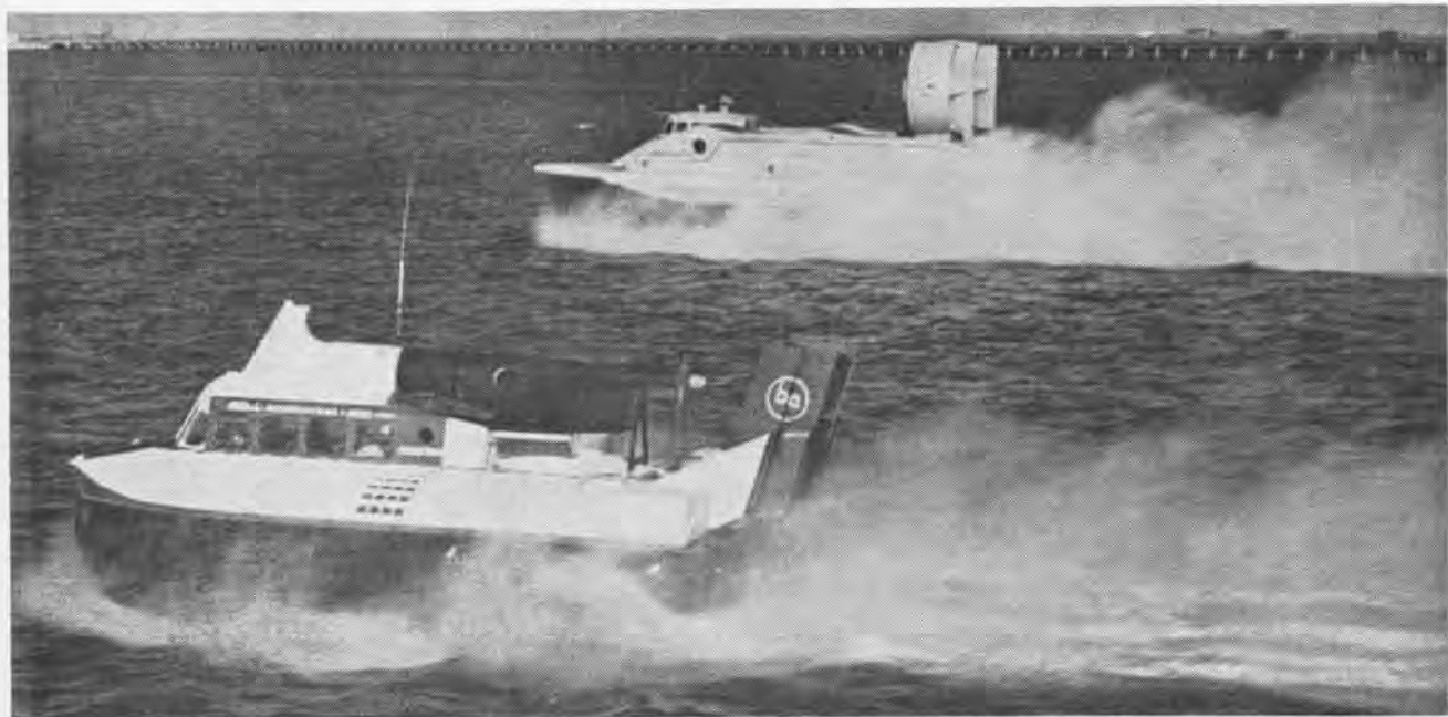
RIDING THEIR OWN CUSHIONS OF AIR, THE SR.N5 (FOREGROUND) AND THE SKMR-1 UNDERGO SALT WATER TESTS AT NAS NORFOLK
