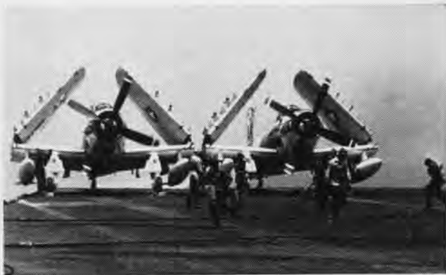
WHIRLING PROPS, ARRESTING GEAR CABLES ARE HAZARDS HOOKMAN'S JOB IS TO CLEAR CABLE AFTER PLANE LANDS
