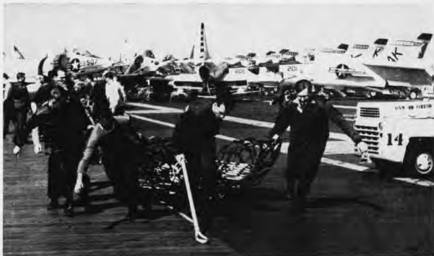
EMPTY NETS are re-spotted by Shangri La crew members for pickup by helo and return to the supply ship. In vertical unrep, some 310 tons of supplies were transferred.
