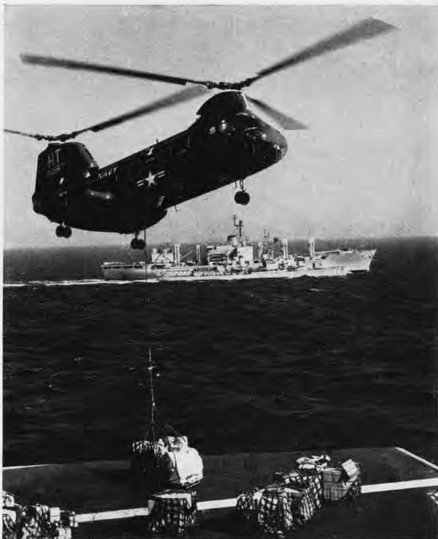
A SEA KNIGHT helicopter deposits net loaded with stores on Shangri La 's deck-edge elevator while supply ship, USS Sylvania , and a destroyer steam on parallel course.
