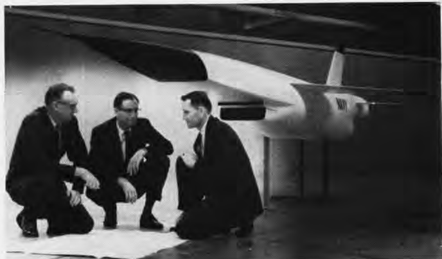
AERONAUTICAL ENGINEERS Ron Reasoner, Sam Sevelson and Carroll Berner discuss the sleek mockup of the new XBQM-34E Firebee at the Ryan plant in San Diego. The high-performance, remote-controlled target drone will be designed and initial fabrication will begin under a $5 million contract signed by the Bureau of Naval Weapons. The drone model will fly at speeds in excess of Mach 1.5 (about 1000 mph) and at altitudes exceeding 60,000 feet.
