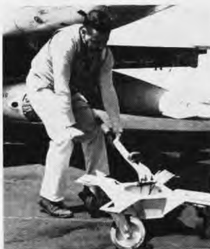
INVENTOR Ens. R. L. Allison demonstrates tail hook dolly now used aboard Roosevelt .
