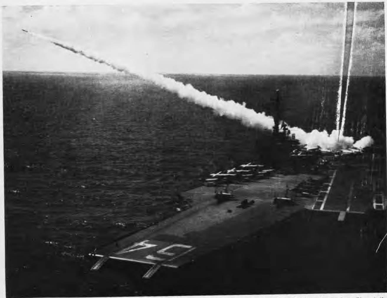
A TERRIER MISSILE streaks from USS Constellation (CVA-64) in the Pacific during exercises. This armament distinguishes the attack aircraft carrier as a member of the Kitty Hawk class. The missile is handled by the GM Division of the Weapons Division in carriers.
