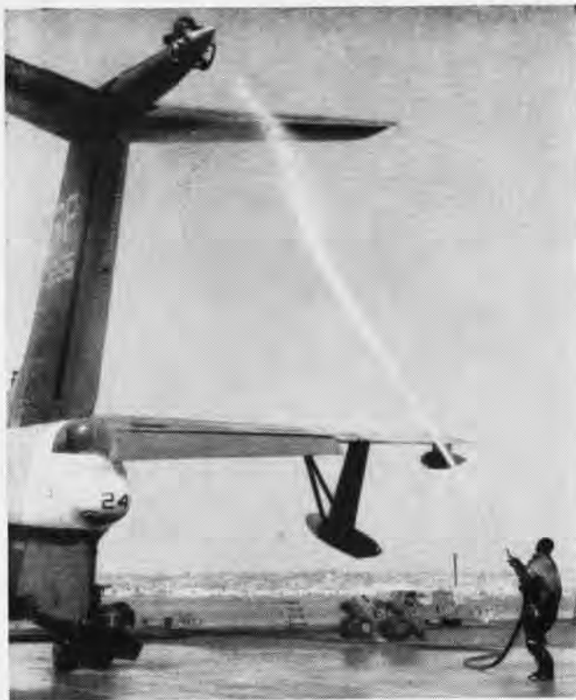
CORROSION CONTROL BEGINS WITH WATER WASHDOWN
