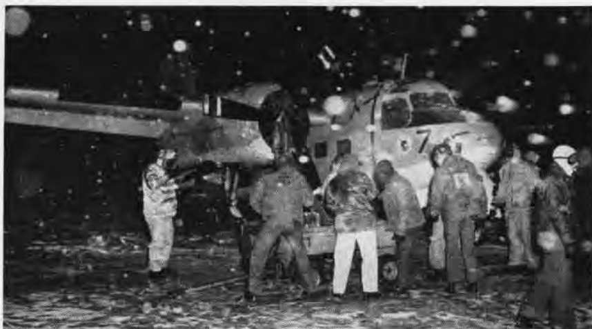
HYDRAULIC LEAK caused an emergency for USS Hornet's mail plane while the ship operated in the snow-swept Sea of Japan; barrier landing caused minor damage, no injuries.
