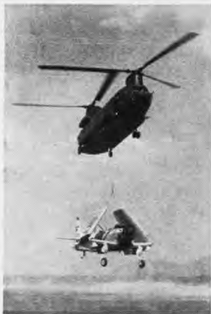
CH-47 AIRLIFTS A DAMAGED A-1
