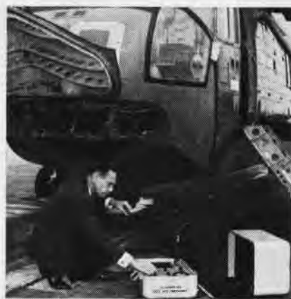
A DEVICE used to pre-flight the AN APN-130A navigation system in the SH-3A has been developed by Ryan Aeronautical Company. The one-man test set is an improved version of the Doppler Radar Test Set in use.
