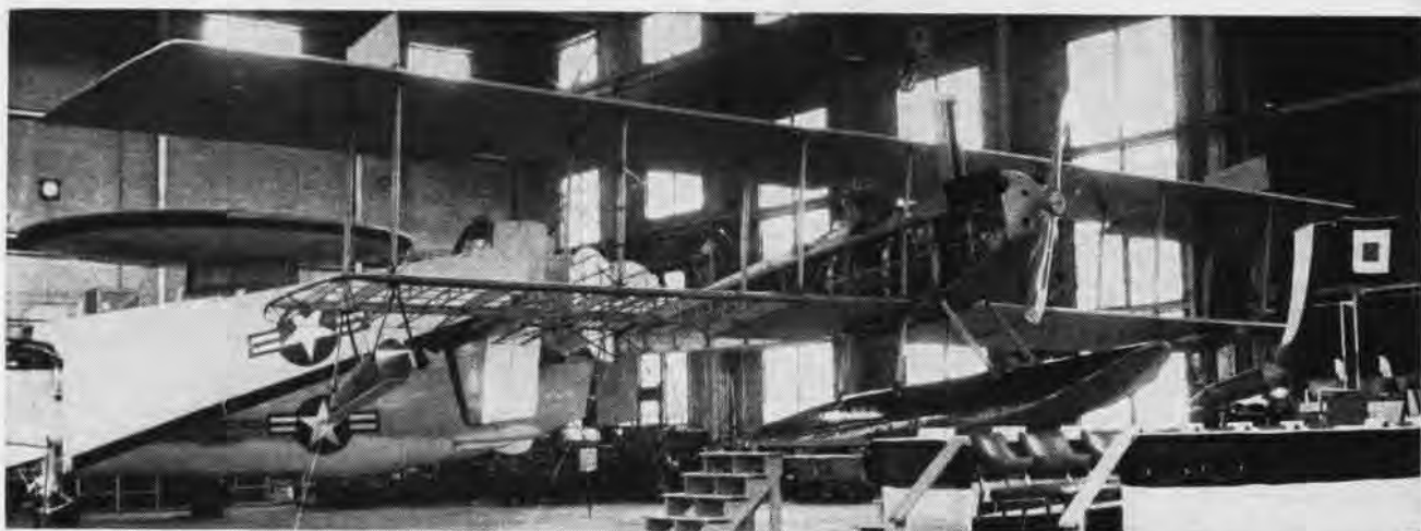
THE N-9 awaits ceremony at Naval Air Engineering Center, Philadelphia. Designed in 1915 as a trainer type seaplane, it is a two-seat aircraft with one float and dual controls. It has a wing span of 53 feet. It was originally equipped with a Curtiss OXX 100-hp engine.
