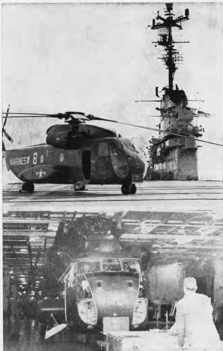
CH-53A HELICOPTER undergoes compatibility evaluation aboard USS Lake Champlain at NAS Quonset Point. The helo is a twin-turbine assault aircraft for cargo or troops.
