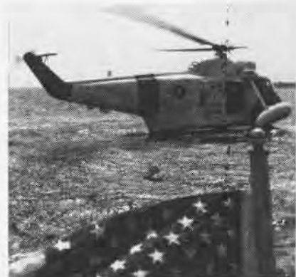
BOAT HULL on helicopter allows a practice water pickup of an airman (foreground).
