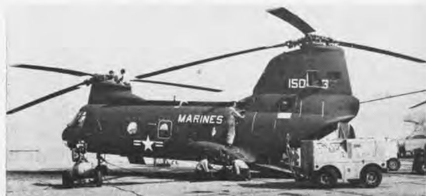
A PILOT REWORK of the Boeing Vertol H-46 Sea Knight has recently been completed at NAS North Island, and the Overhaul and Repair Department is now in full rework production of the new tandem rotor helicopter. The H-46 is powered by General Electric twin T-58-8 turbine engines which also are overhauled at North Island. The H-46 is being used in Vietnam where its rapid loading and unloading capability is vitally important.
