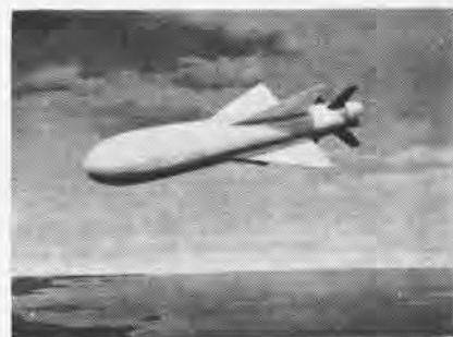
CONDOR, a new air-to-surface missile being developed by North American Aviation for the Navy, is shown in an artist's drawing. The missile relies on television for guidance and is adaptable to armament systems of current and future aircraft.
