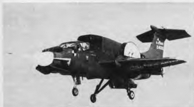
LIFT FANS in wings and pitch control fan in nose characterize Ryan/GE XV-5A V/STOL test aircraft. Exhaust of two GE J-85's is diverted to drive fans, and louvers and doors opened for VTOL operation.
