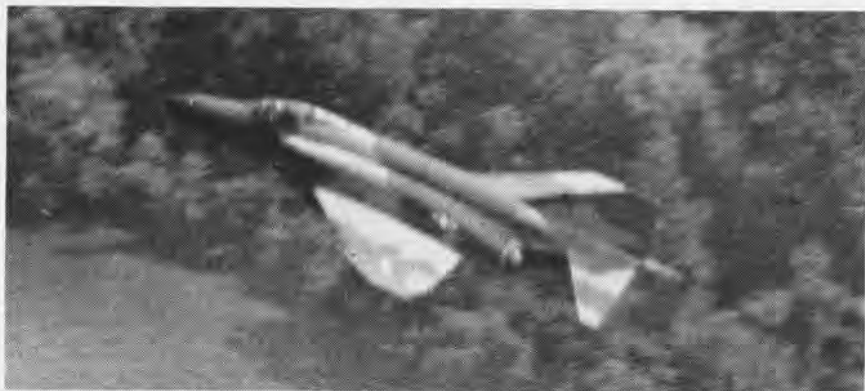
IN ITS NEW GREEN and brown camouflage, an Air Force RF-4C Phantom II hides against a wooded riverside. United States Air Force aircraft to be used in combat zones now feature the new color scheme designed to make them difficult to detect from above.
