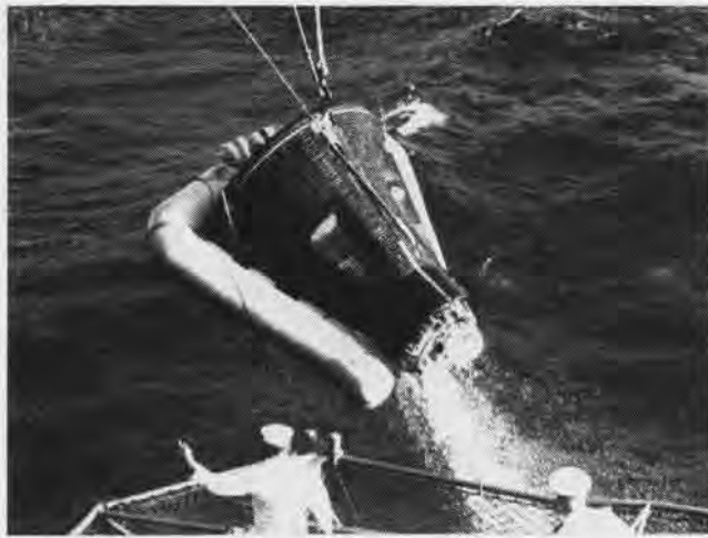
GEMINI III spacecraft of Grissom and Young comes aboard Intrepid in March, the first of five recovered by Navy carriers this year.
