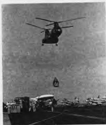
UH-46C HELICOPTERS from supply ships lift cargo to other ships operating at sea.
