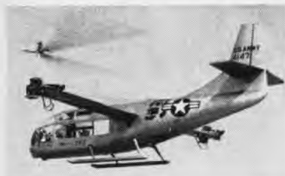
OLD TIMER in the DOD V series is Bell's XV-3A tilt propeller carried over from the earlier Army/AF convertiplane series.
