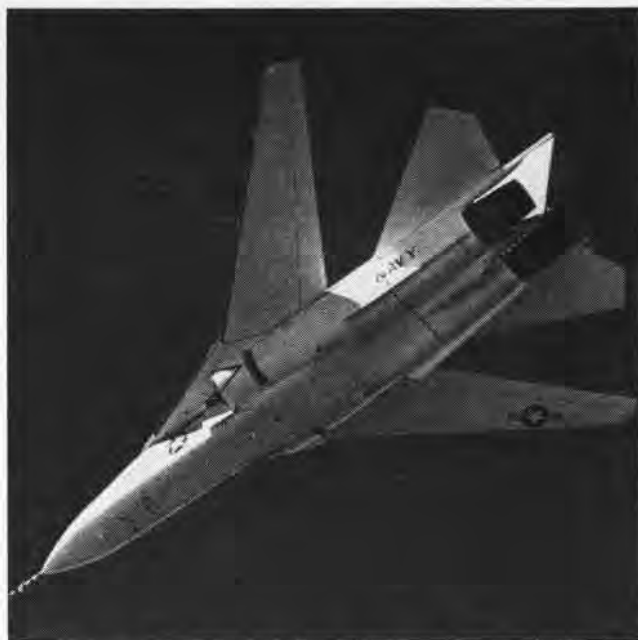
GRUMMAN F-111B , Navy version of jointly developed tactical fighter, TFX, demonstrated variable wing sweep on first flight in May.
