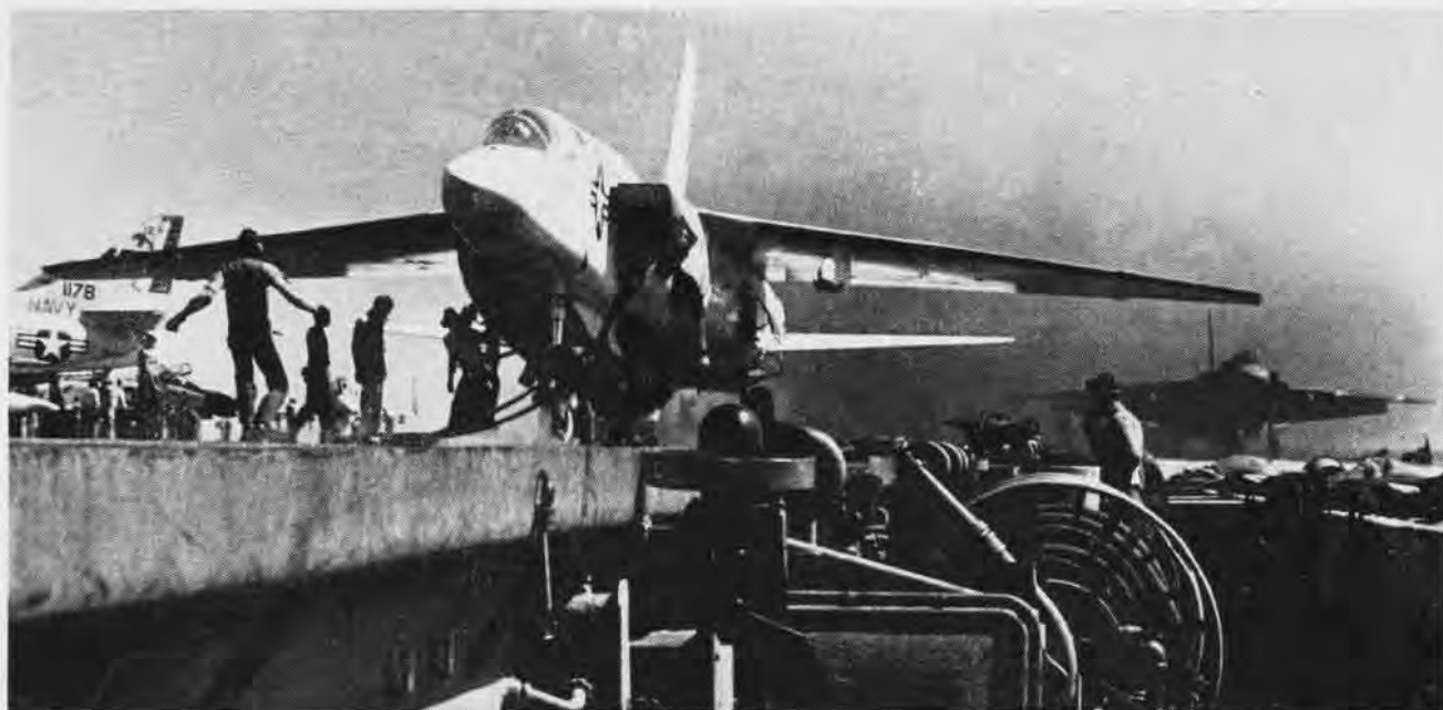
SECONDS BEFORE the launch of an RA-5C, a catapult crew attaches the bridle to another Vigilante to be launched off the waist catapult. Feverish action depicted above was typical of the daily activities aboard Independence as she steamed in seas off Vietnam.
