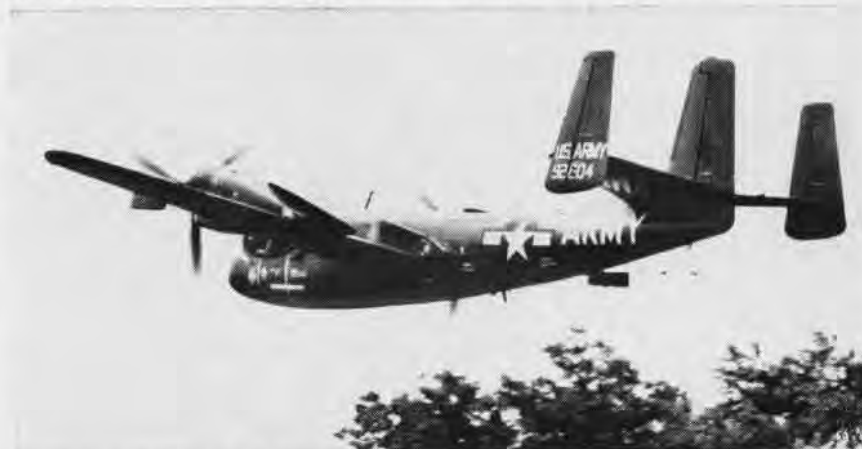
INITIAL MODEL in the V/STOL series is the Grumman OV-1 Mohawk, formerly the OA-1, a high performance propeller type reconnaissance aircraft powered by two 1150 hp Lycoming T-53 engines. The various versions carry different camera and electronics installations.
