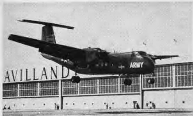
CV-7A CARIBOU , an STOL transport developed by de Havilland/Canada for U.S. and Canadian Army is undergoing operational evaluation in Vietnam. It is powered by two 2850 hp. G. E. T-64's.
