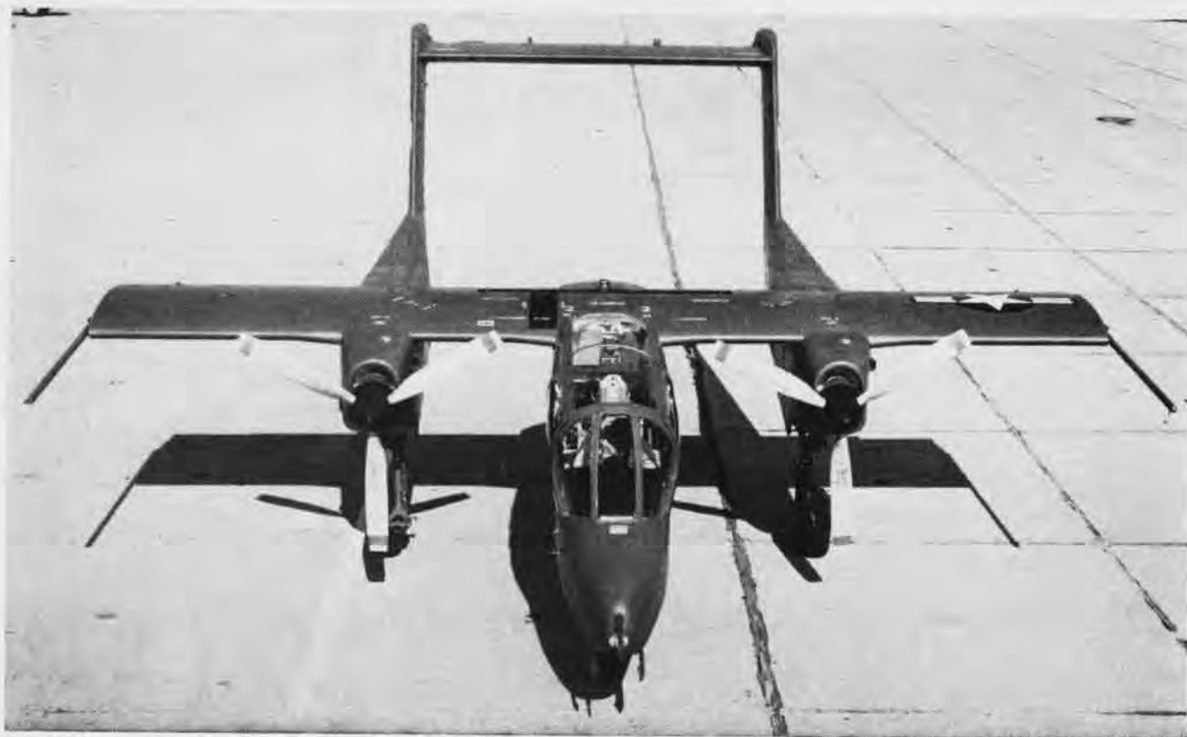
NEWEST in the V/STOL series is North American's OV-10A, which is being developed under a BuWeps contract. The two-place STOL is powered by a pair of 660 hp. AiResearch T-76 turboprops. The OV-10A is being developed to meet the needs of all three services in advanced area operations for reconnaissance, attack and utility. Use by other nations as a counter-insurgency aircraft is also envisioned.
