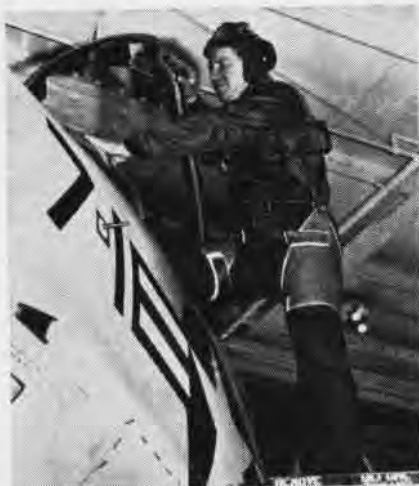
THIGH-TYPE harness allows plane captain greater ease in strapping into the cockpit.
