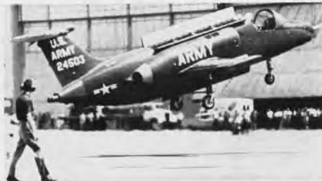
LOCKHEED XV-4A Hummingbird VTOL was designed, built to evaluate jet augmentation lift system. Augmentation with airflow entering through doors in top of fuselage did not measure up to predictions.
