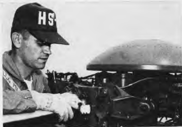
BIM INDICATES THIS BLADE IS SUSTAINING PRESSURE WHEN PRESSURE IS LOST, BLACK STRIPES SHOW ON BIM
