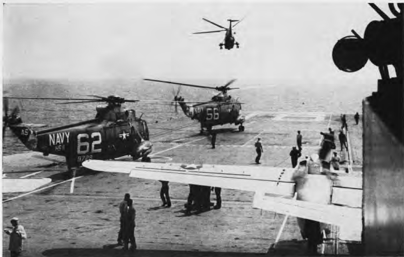
SEA KING helicopters are launched from the ASW carrier USS Wasp in the Atlantic. The helicopters are bound for an early-morning ASW practice mission. At right, an S-2E Tracker moves up for a catapult launch. Helos double as plane guards for fixed-wing planes.
