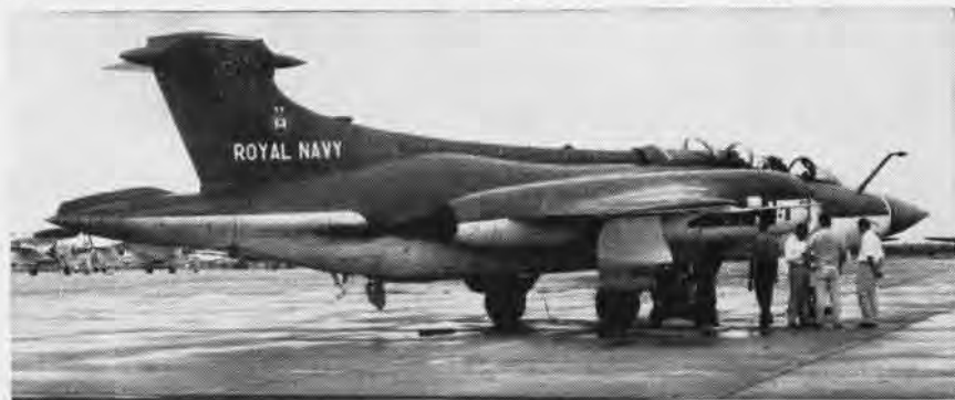
THE ROYAL NAVY'S Buccaneer II has completed two and one half months of flight tests in hot and humid weather conditions at NAS Pensacola. Trials were held to determine the aircraft's performance under low-level flight conditions. The majority of the flights were made at sub-sonic speeds at an altitude of 200 feet. The Buccaneer , which has a nuclear and a conventional capability, is comparable in weight to the U. S. Navy's A-6 Intruder .
