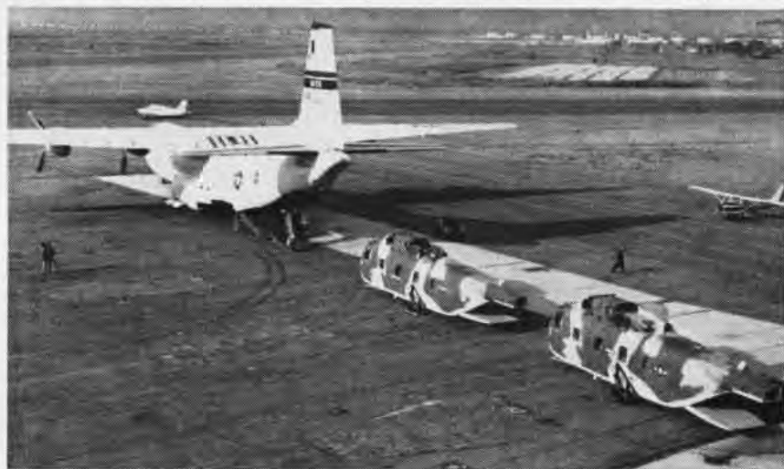
TWO SIKORSKY HH-3C helicopters of the USAF's Air Rescue Service are loaded aboard a giant C-133 transport at Bridgeport, Conn., for speedy delivery to South Vietnam. The camouflaged helicopters, fitted with armor plating, jettisonable fuel tanks, new rescue hoists and other improvements, are designed to improve the Air Force's ability to locate and pick up airmen who have been shot down in the jungle or behind enemy lines.
