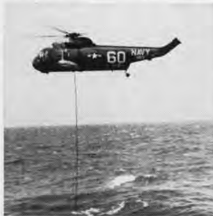
HOVERING 40 feet above the water, SH-3A dips sonar dome to listen for submarine.
