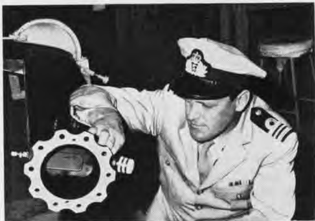
BIM INDICATES THIS BLADE IS SUSTAINING PRESSURE WHEN PRESSURE IS LOST, BLACK STRIPES SHOW ON BIM
