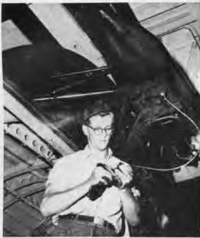
DUANE R. POMEROY, AX2, works on helo sonar rig; SH-3A uses cable to dip sonar.
