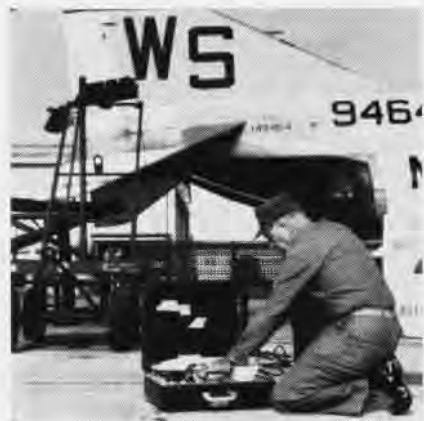
ADAMS X-RAYS TAIL FIN OF AN F-4
