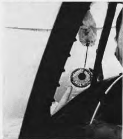
AN A-3B prepares to take on fuel from another Skywarrior returning from a mission.
