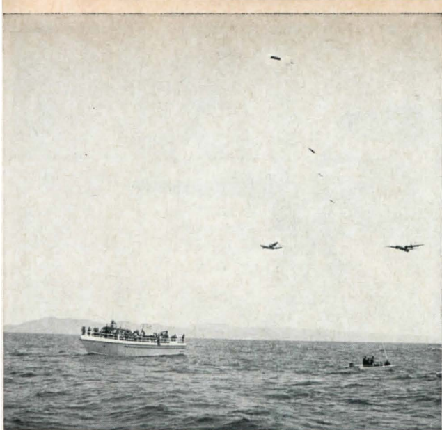
UNITING the Robert Fulton system (originally developed under a contract with Navy's Office of Naval Research) and an HC-130H, the U.S. Air Force demonstrates its new air/sea rescue method. The "victim" in the lifeboat, LCol. T. R. Harris, has donned a suit with a built-in harness and inflated a balloon which lifts the nylon cable.
