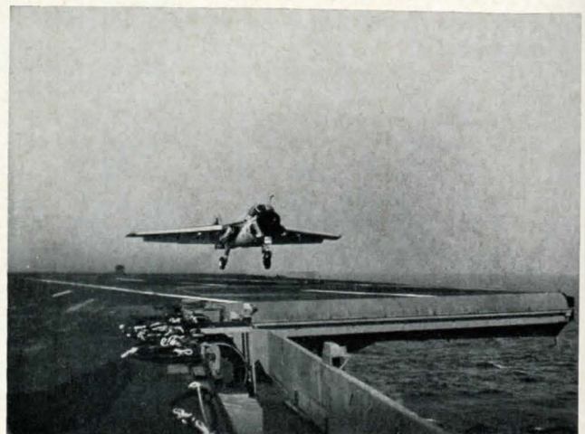
NAEL (SI) is responsible for developing launching and arresting gear. Above, an A-6 Intruder is launched by a waist steam catapult.
