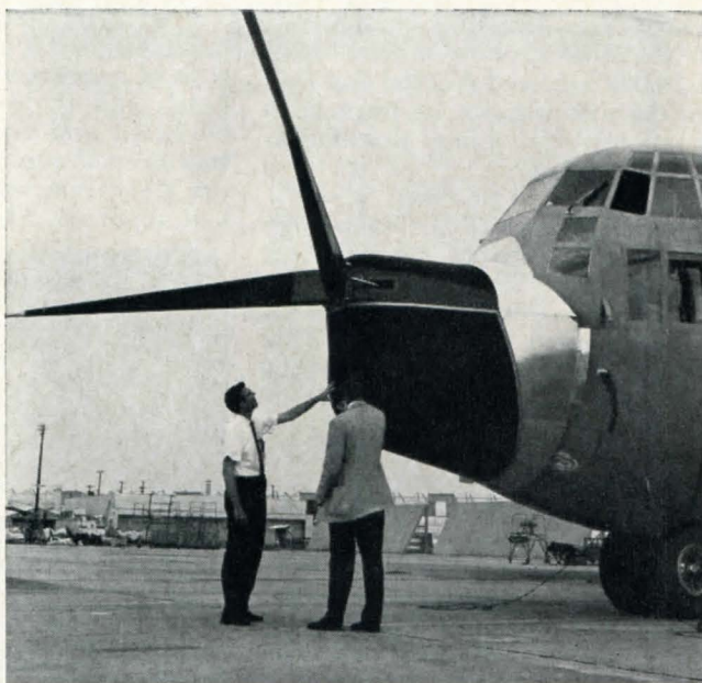
THE BEETLE-LIKE protuberances (which can be folded back along the nose) are the "yoke" of the apparatus. The yoke is part of the Fulton recovery system which retrieves objects or persons weighing as much as 500 pounds. The rescue package with nylon cord is dropped to the astronaut or survivor who dons harness and sends up balloon.
