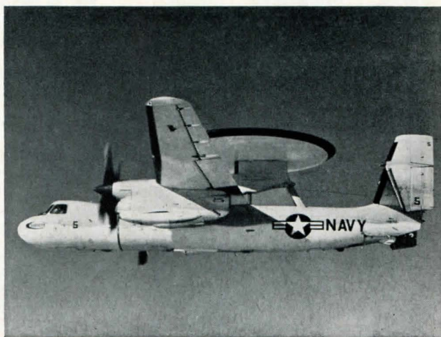
COMPLETELY pressurized, the Hawkeye offers full air conditioning while operating from the deck to service ceiling of 30,000 feet.
