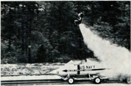
ACEL TESTS experimental rocket escape system by firing it from jet-propelled sled.
