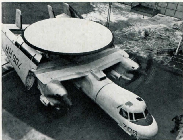
BIG BUT compact, the 24-foot rotodome lowers almost flush to the fuselage and the 80-foot wing spread folds to 30 feet for stowage.
