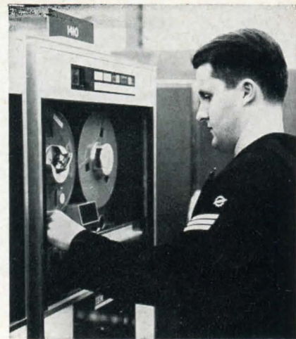
DATA received from four tracking stations are recorded on tape and fed into computer.
