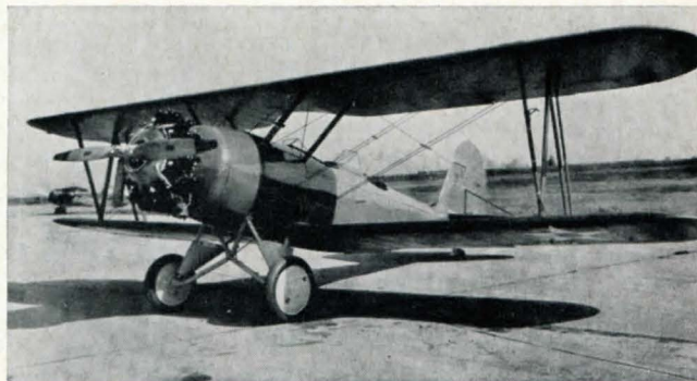
FAMED 'YELLOW PERIL' , designated the N3N-1 landplane trainer, built during the 1930's, was also product of Naval Aircraft Factory.
