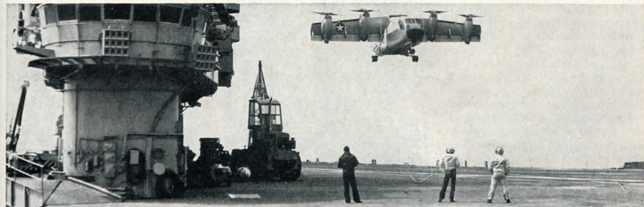
XC-142A HOVERS JUST BEFORE RADICALLY CHANGING ITS WING ANGLE AND TURNING SHARPLY FOR FLIGHT
