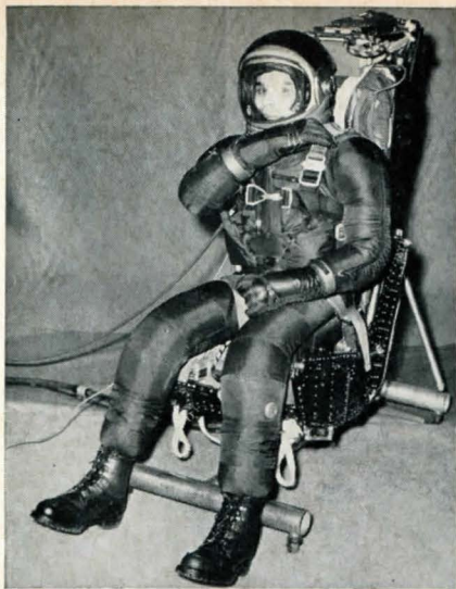
FULL PRESSURE suit is tested for mobility at Aerospace Crew Equipment Laboratory.
