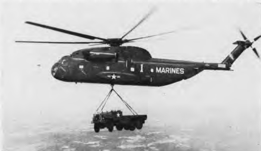
COMBINING SPEED with heavy lift, a Sikorsky CH-53A assault transport lifts a 6½-ton truck and, at an altitude of 5,000 feet, carries it through the air at 138 miles an hour. In its normal military mission, the CH-53A carries 38 fully equipped troops or four tons of cargo at a cruising speed of 172 miles per hour. BIS trials begin this month at NATC, Patuxent River, Maryland, with delivery to Marine Corps operating units later this summer.
