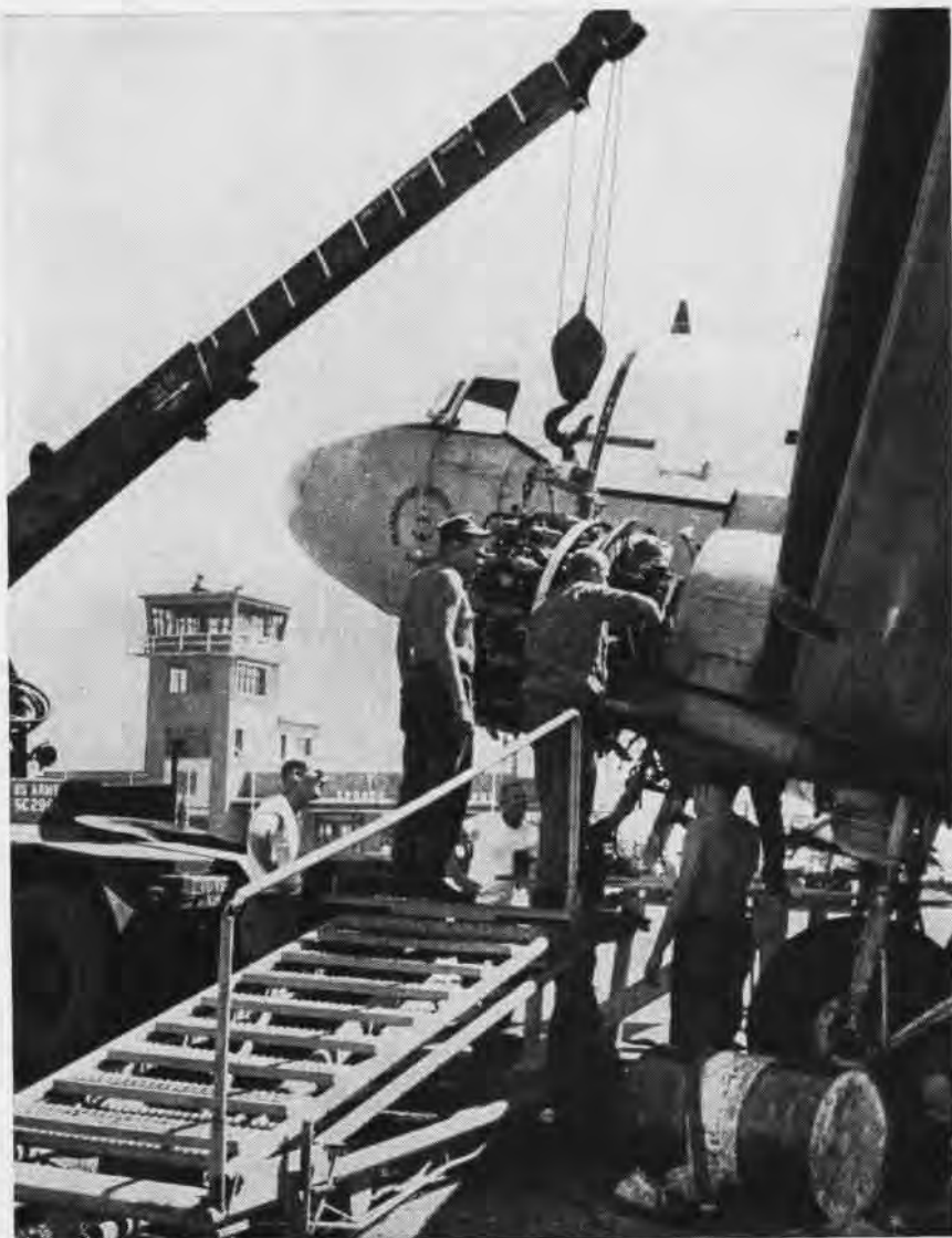
PILOTS AND CREW members of an Air Cofat C-47 Skytrain install a new engine in their plane. The transport limped into a Vietnam air strip, just missed jungle crash.
