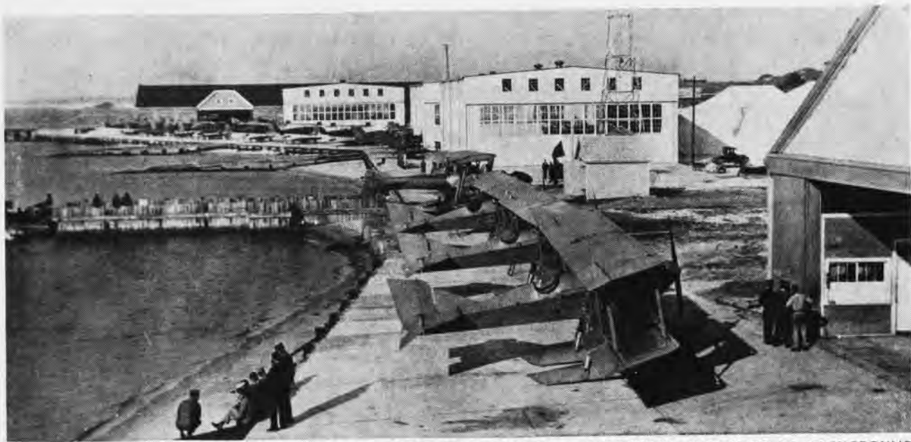
IN JANUARY 1917 SCENE AT PENSACOLA ARE THREE STURTEVANTS, A GALLAUDET AND N-9'S IN BACKGROUND
