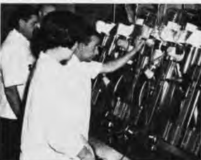
TECHNICIANS keep close watch on machine which clumps the red cells prior to freezing.
