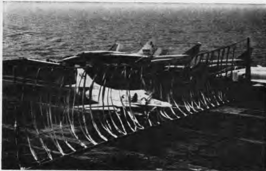
A-4C SKYHAWK , piloted by Ens. John A. Lockhard of VA-112, is pulled to a safe stop by an arresting barrier rigged aboard Kitty Hawk . The A-4 was hit by enemy AA fire.
