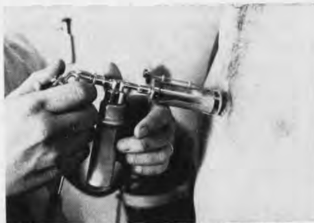
A TINY electrode is attached to skin with fast drying cement by a NASA technician. Three electrodes were fastened to pilots' chests.
