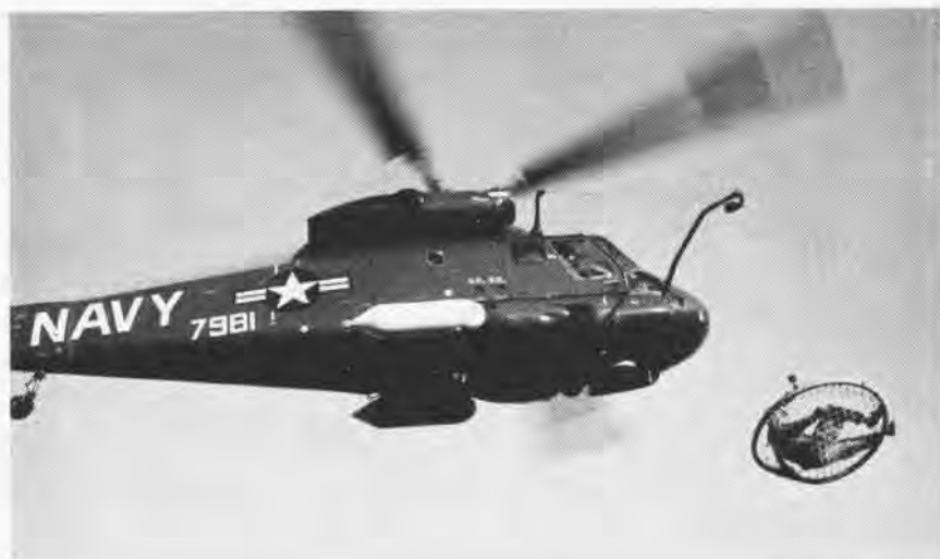
UH-2C Seasprite demonstrates the new fishpole boom used to rescue personnel (above). Photo at right illustrates the accessibility of the power plant. Poised bug (below) shows twin-engine configuration.
