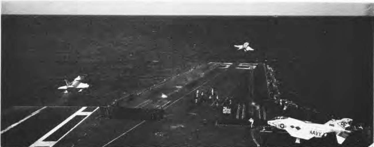
AIRCRAFT are launched simultaneously from waist and bow catapults of the nuclear-powered Enterprise . The widely varied missions of attack air wings mean that radically different aircraft, such as the Phantom and the Skyhawk, will be included in CVW composition.
