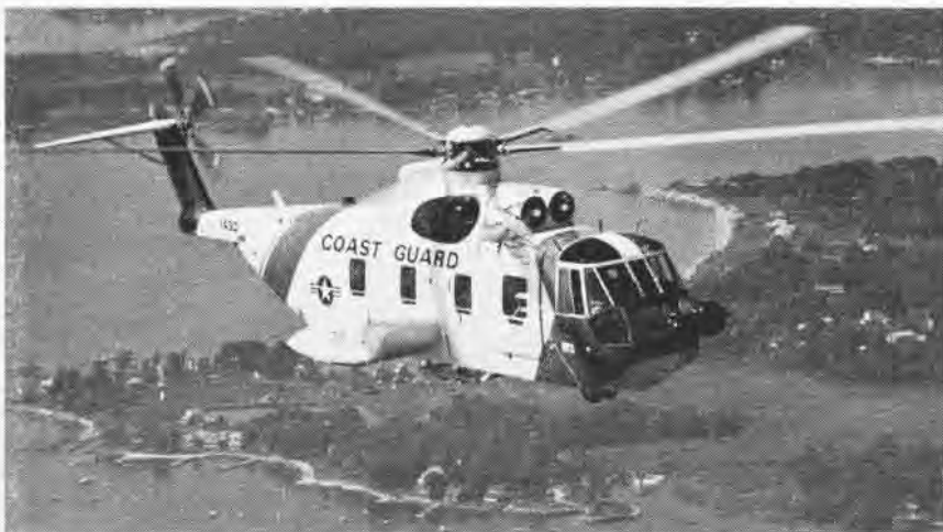
A U.S. COAST GUARD helicopter with the most sophisticated electronics, navigation and instrument systems ever carried by an SAR rotary-wing aircraft made its debut at Sikorsky Aircraft, Stratford, Conn., October 11. Powered by two GE T-58-5 gas turbine engines, each with 1,500 hp. rating at takeoff, the HH-3E has a top speed under normal power of 157 mph, a cruising speed of 150 mph. The helicopter carries external rescue hoist with 240 feet of usable cable. Spanson and pop-out flotation bags allow landings and pickups in rough water. The helo can fly 345 miles out to sea, hover 20 minutes, pick up six survivors and return to land.
