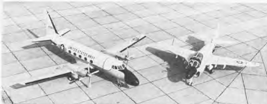
THE FEDERAL Aviation Administration has issued R-4b type certification for the Grumman TC-4C, a systems training aircraft to be used by the Navy for training crews of the A-6A Intruder (NAnews, February 1967, p. 17). The TC-4C's operational envelope—airspeed, gross weight, center of gravity and altitude limitations—is the same as that of Gulfstream I. Navy Preliminary Evaluation began in November. Grumman is under contract to build nine TC-4C's.
