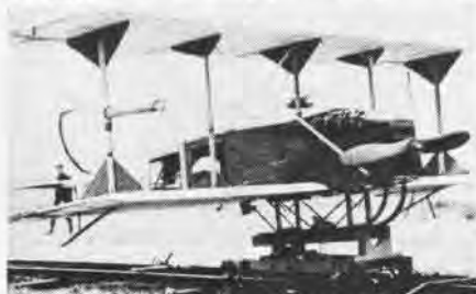
CURTISS HA initiated the Navy's development of fighter aircraft. The Flying Bomb was an early attempt to develop a guided missile. NAS
