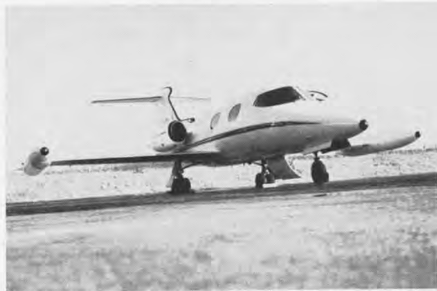
THE U.S. NAVAL Test Pilot School at NATC Patuxent River recently conducted a limited evaluation (nine flights) of the Lear Jet Model 24. NATC representatives also participated. Empty weight of the aircraft is 7,200 pounds and maximum takeoff weight is 13,000 pounds. It has a high-speed cruising capability of approximately Mach .8 and lands at between 115 and 125 knots. In ten minutes from brake release, it climbs to 40,000 feet.
