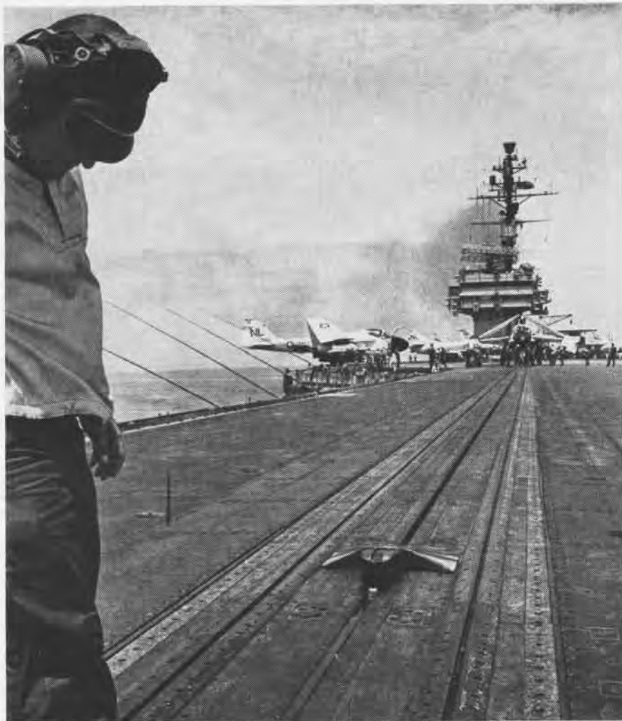
LT. R. D. PFEIFER CHECKS CAT TRACK ABOARD CONNIE BEFORE A LAUNCH
