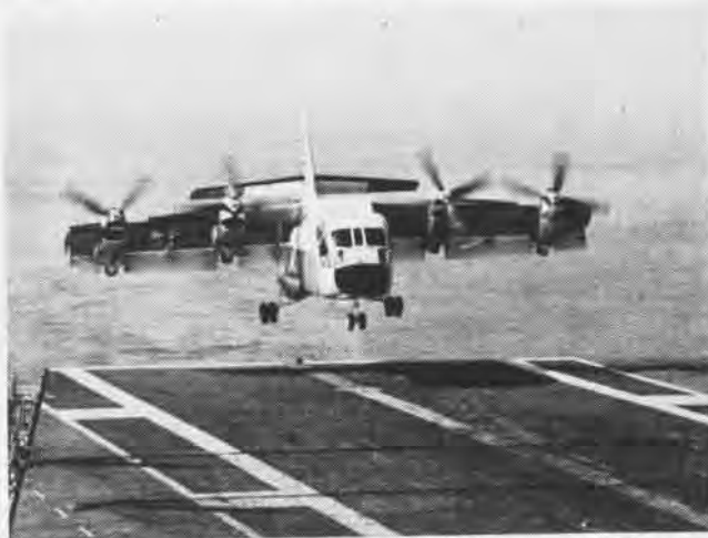
THE TRI-SERVICE XC-142A V/STOL landing aboard USS Bennington during carrier suitability trials at sea off San Diego in May.
