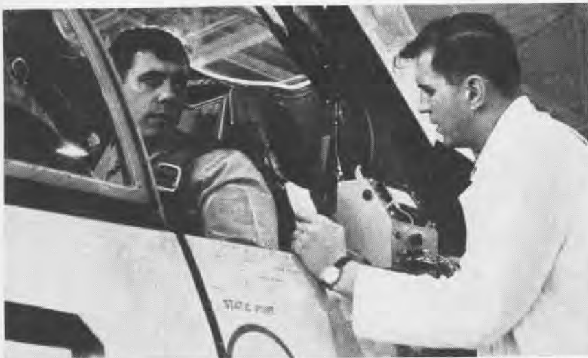
PR1 GILMORE asks Lt. Polski about his Mk 5 anti-exposure suit. The box near Gilmore's hand is a battery-powered tele-thermometer used to take the pilot's skin temperature.
