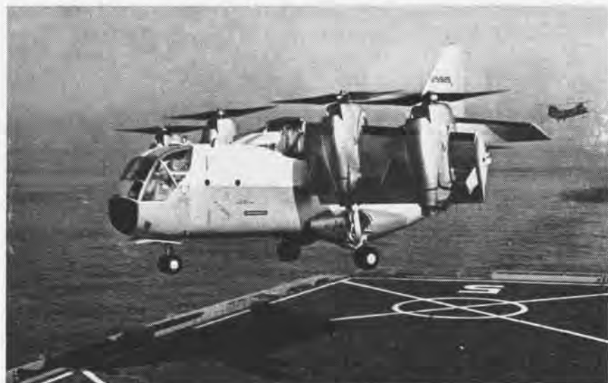
USS OGDEN, an amphibious transport dock, made aviation history when, on November 28, 1966, she became the smallest ship thus far to land the XC-142A on her helicopter flight deck. The aircraft, which looks like a flying boxcar, made seven landings as Ogden steamed off Coronado's Silver Strand. The tilt-wing aircraft, the largest U.S. V/STOL ever built, takes off and lands vertically like a helicopter, but flies forward like a conventional transport.
