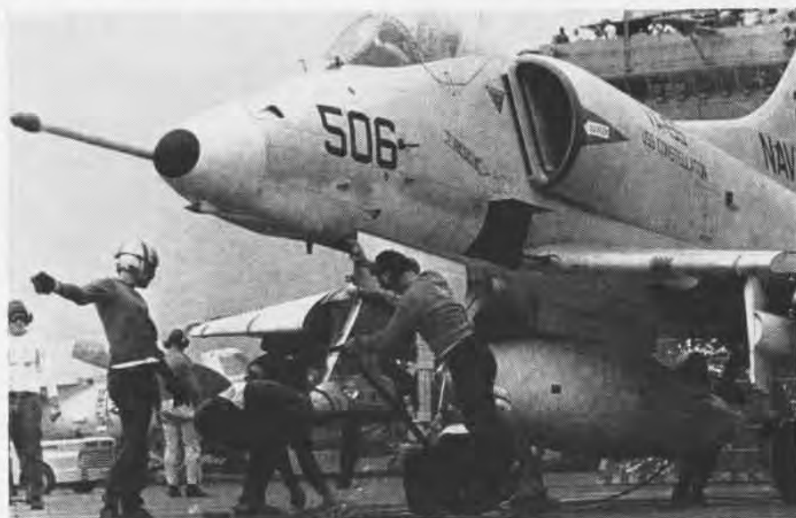
BRIDLE IS ATTACHED TO A-4 AS THE PLANE IS POSITIONED OVER CATAPULT
