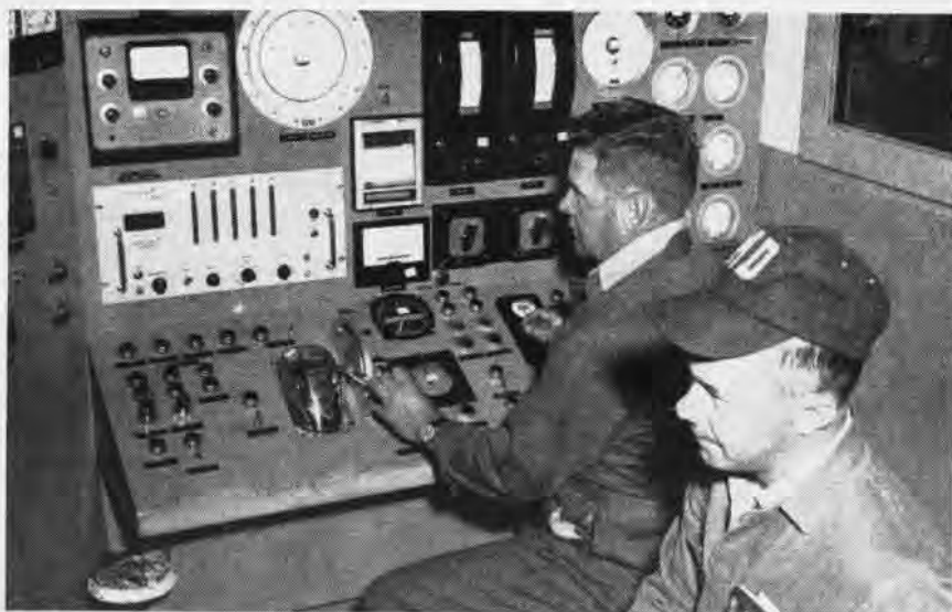
TWO MEMBERS of the jet engine test cell crew check the controls to uncover defects as the engine is put through its paces after it has undergone a thorough overhaul at Oceana.
