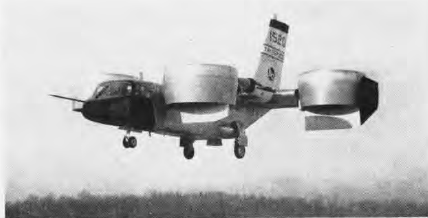
THE FIRST public flight test of Bell's Tri-Service X-22A V/STOL aircraft took place May 9 at Niagara Falls International Airport before more than 300 military observers and news media representatives. Buffeted by winds up to 24 mph, the research aircraft was put through its paces in an 18-minute show. To display the X-22A's STOL capabilities, the pilots took off after using only 330 feet of runway and landed in about 600 feet of runway. Piloting the X-22A on the flight was Chief Test Pilot S. J. Kakol. The copilot for the flight was Paul Miller, Jr., manager of test operations for Bell Aerosystems Company.
