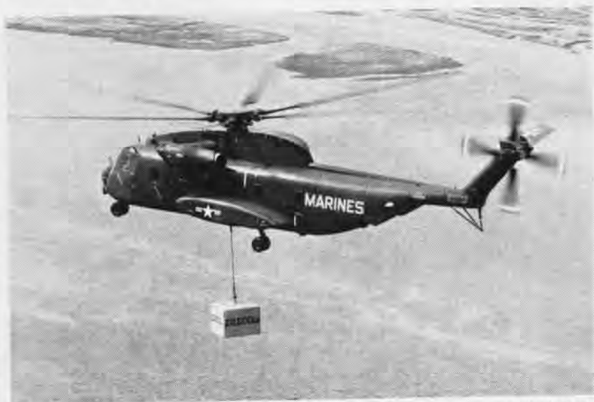
AT STRATFORD, Conn., in May, a Sikorsky CH-53A was flown at a gross weight of 46,000 lbs., highest ever recorded by a Free World production helicopter—previous record was 44,000 lbs., flown by a U.S. Army CH-54A—and 11,000 lbs. over the helo's gross weight. The standard CH-53A was powered by T-64-6 engines. Speed with the external load was 127 mph; with internal load, 150 mph. Test pilots were Richard Wright and John Peterson.
