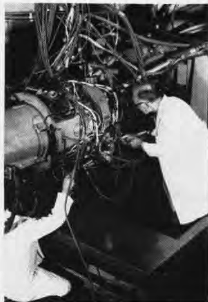
ALLISON T56-A-7 engine is being prepared for dynamometer stand at AEL Philadelphia.
