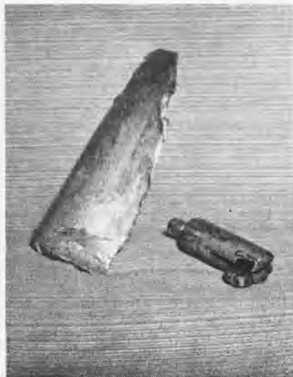
SMALL piece of material, sucked through a jet engine, damaged titanium blade (left).
