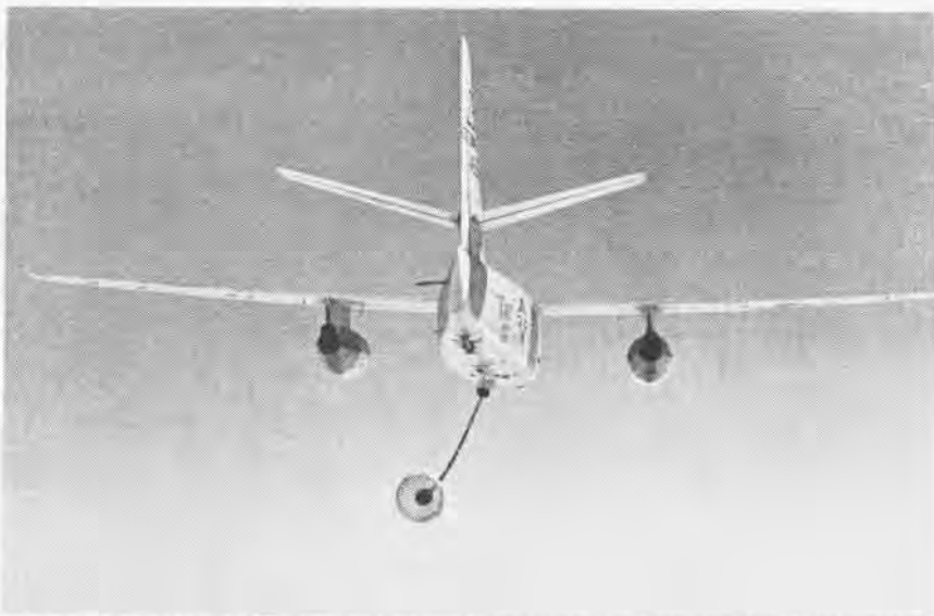
CUSTOMER AIRCRAFT APPROACHES AS TANKER EXTENDS REFUELING HOSE
