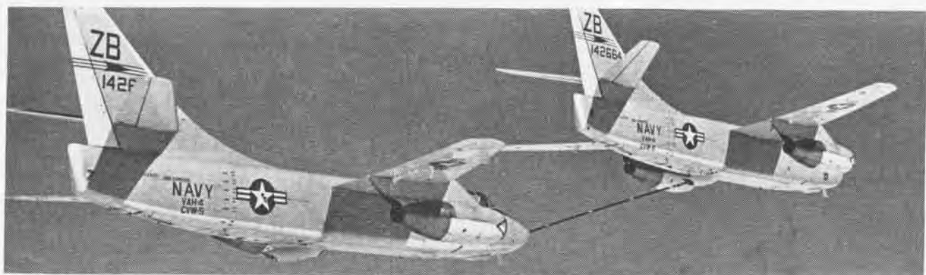
AT MORE THAN 400 GALLONS PER MINUTE, AN A-3B TANKER FROM USS HANCOCK REFUELS ANOTHER SKYWARRIOR
