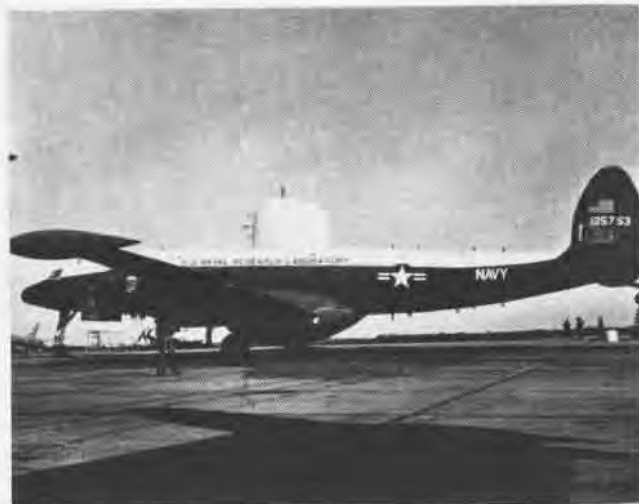
NRL specially-instrumented plane is used for atmospheric electricity studies. Cannon-like projections from the dome take in air samples.
