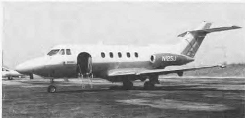
A U.S. NAVAL Test Pilot School evaluation team has completed a limited evaluation of the British Hawker Siddeley DH-125 at NATC Patuxent River. The DH-125 is an eight to ten-passenger executive jet transport powered by two Viper turbojet engines. Empty weight is approximately 11,000 lbs.; maximum gross weight for takeoff, about 21,000 lbs. Team members were Cdr. D. Z. Skalla, LCdr. D. Rice, LCdr. G. A. Aitchison and Lt. G. F. Wheatley.
