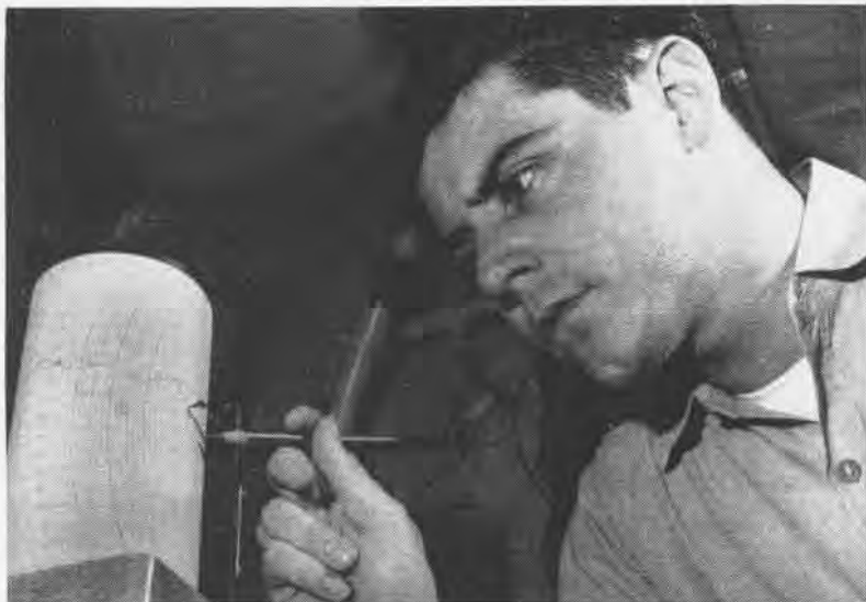
A HANCOCK third class aerographer's mate, Ken Blair, checks the atmospheric pressure with a micro-barograph as his CVA operates in the Gulf of Tonkin off Vietnam.
