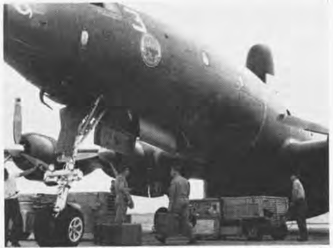
CREWMEN give final preflight check to one of the squadron's EC-121K Super Connies. Aircraft will fly a 15-hour weather recon mission.
