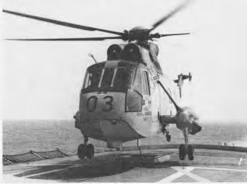
HELO LANDING ABOARD SHIP IS ASSISTED BY RAPID HAULDOWN SYSTEM
