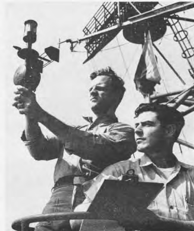
ANEMOMETER "reads the wind" for AG3's James Sanders and Kenneth Blair as they obtain data on true wind as well as its velocity.
