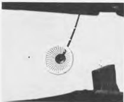
FUEL HOSE BASKET IS NOW READY
