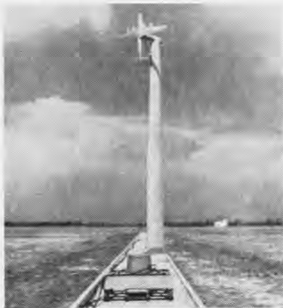
ANTENNA with model on top is used for testing sonobuoys at NATC Patuxent.
