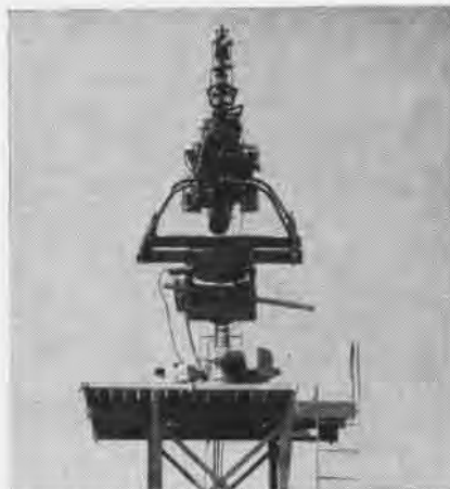
SUPPORT tower is used to position large models or full scale antennas for tests.
