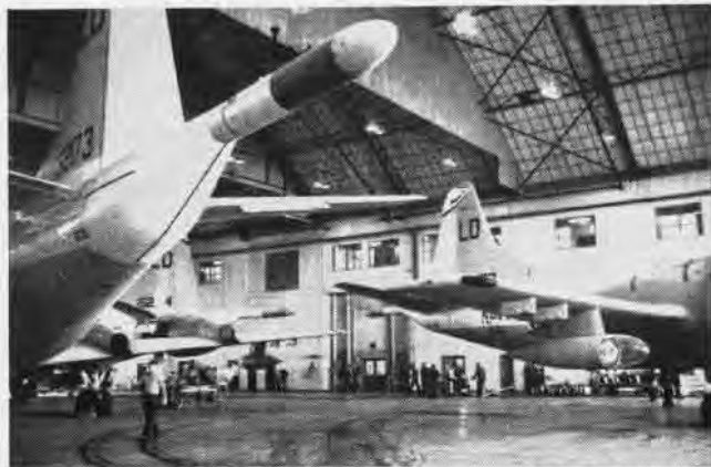
THREE ORION 'MAD' BOOMS JUT INTO VP-10'S HANGAR
