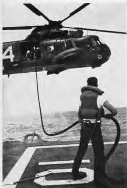
REFUELING without having to land gives the helicopters added time for operations.
