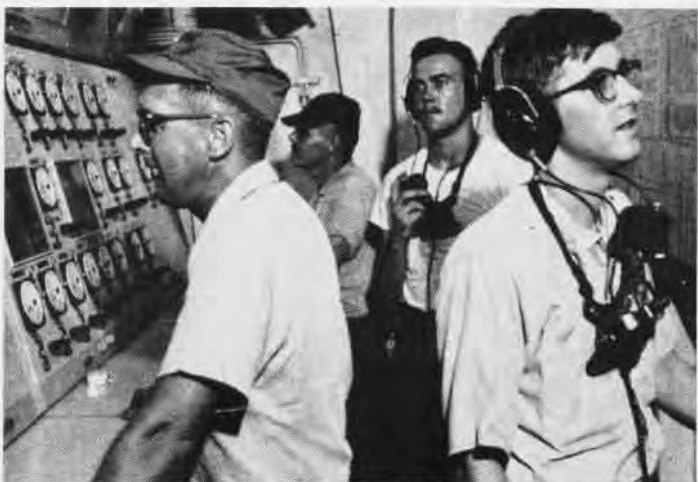
CREWMEN CHECK BALLAST CONTROL VALVES ABOARD LPD
