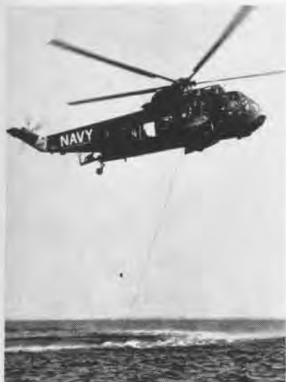
AN RH-3A dunks its mine countermeasures gear in the sea to determine effectiveness.
