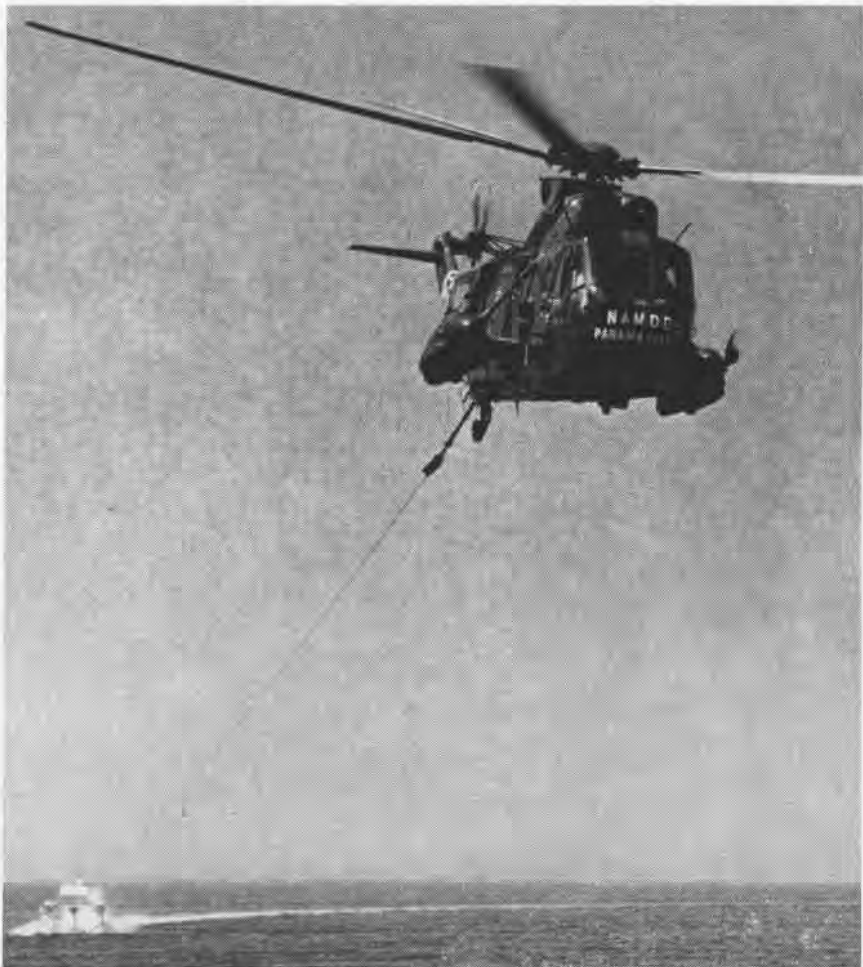
ONE OF THE WAYS an RH-3A helicopter enacts its minesweeping role is to pull a mine countermeasures sled in a wide sweep, thus making the sea-lane safe for oncoming vessels.
