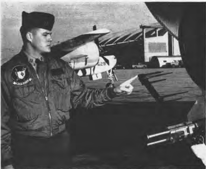
PILOT POINTS TO TRAVERSING RAKE SYSTEM MOUNTED ON AFT FUSELAGE
