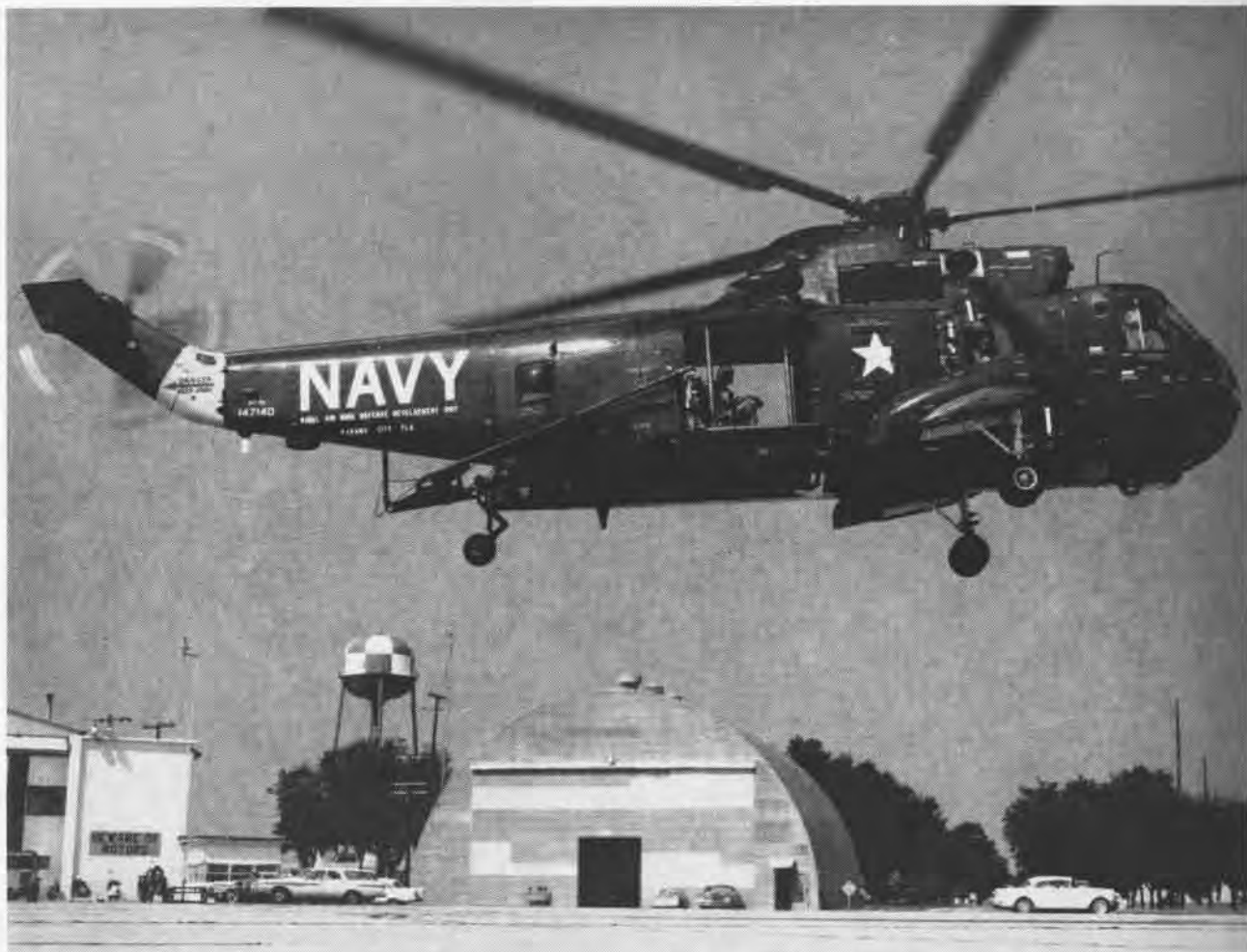
AGAINST THE BACKGROUND of the hangars of the Naval Air Mine Defense Development Unit, an RH-3A takes off from the flight section at the Panama City facility. Equipped for mine countermeasures, Sikorsky helo demonstrates virtues of whirlybird as minesweeper.
