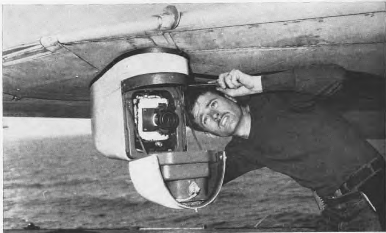
PH1 G. R. JOHNSON ADJUSTS A CAMERA POD MOUNTED ON THE WING OF AN A-4 SKYHAWK ABOARD CORAL SEA
