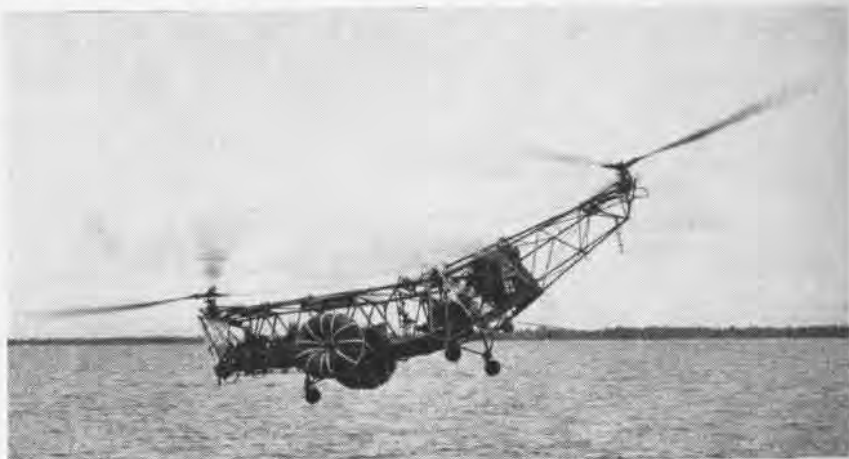
WHEN THE NAVY first considered using the helicopter as a minesweeper, it used an HRP type as a starter. The technique has come a long way since its initial trials and tests.
