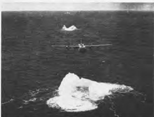
USCG HC-130B ice patrol plane, hedge-hopping a row of icebergs off the coast of Labrador, has selected the berg in foreground for marking by an aerielly dropped chloride-rhodamine "B" dye bomb. The Coast Guard is engaged in an intensive assault on huge floating icebergs, locating them and notifying ships of their location.
