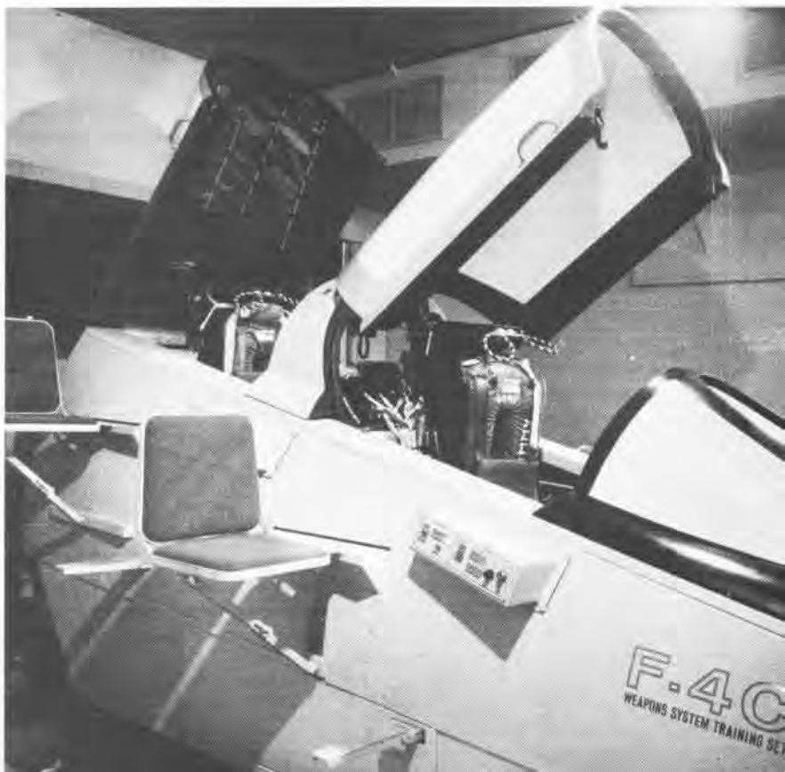
The weapon system trainer shown above and below is for the USAF version of Navy's famed Phantom II. As one of today's Link products, it trains pilots and RIO's for their missions in the two-seat, all-weather fighter.
