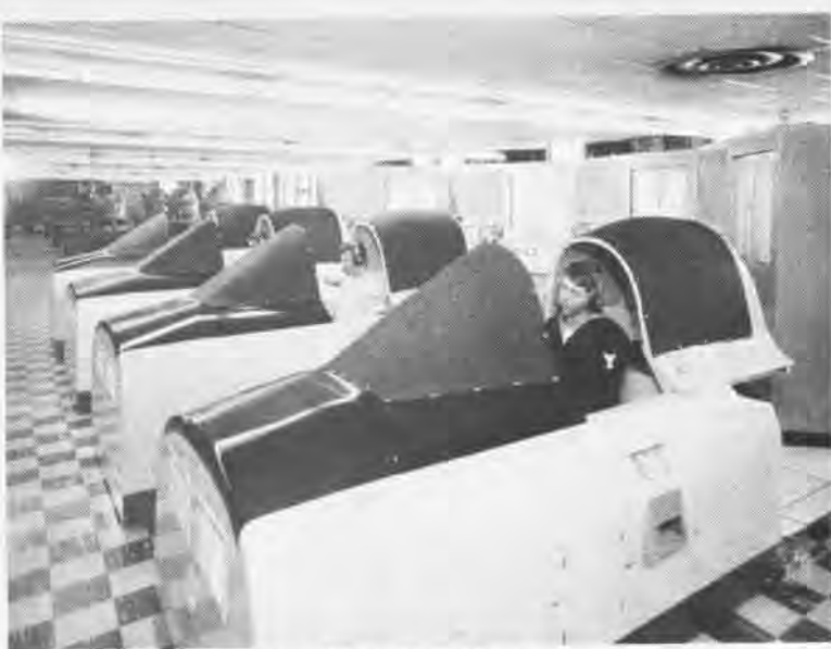
Learning at Naval Air Station, Whiting Field, Fla., is speeded by the use of a new four-cockpit instrument training system, built by the Link Group of General Precision Systems, Inc.
