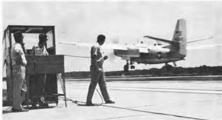
LT. PETE Percou operates the landing lens and lights to notify the pilot of a C-1A aircraft from the carrier USS Forrestal when he is to cut his power and land.
