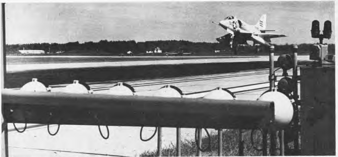
AT NALF FENTRESS FIELD, A PILOT OF AN A-4 SKYHAWK USES THE FRESNEL LENS SYSTEM AS HE PRACTICES HIS FIELD CARRIER LANDINGS
