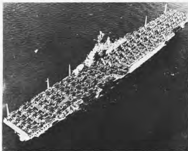
A QUARTER-CENTURY of service by the ASW carrier Essex is typified by these two photos. Shot at left, taken in May 1944, shows the ship's straight flight deck crowded with aircraft and with gun mounts for-
