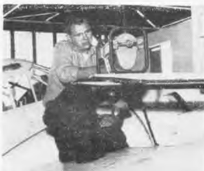
AT NAS ALAMEDA'S Aircraft Maintenance Department, the "bones" of aging Beechcrafts are examined and X-rayed for structural damage. AMI's C. T. Packer and H. V. Parks, specially-trained X-ray technicians, are the only personnel allowed to operate the equipment. They rope off a 100-foot X-ray area and position the camera over the wing
