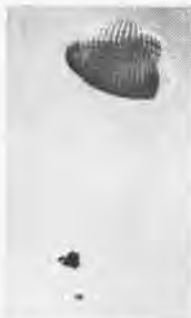
After ejection, pressurized module is stabilized by its glove section until recovery chute is deployed. Pitch flaps help achieve horizontal stability. The recovery chute controls rate of descent at 31 feet per second. F-111's chute deployed after drop to 15,000 feet.
