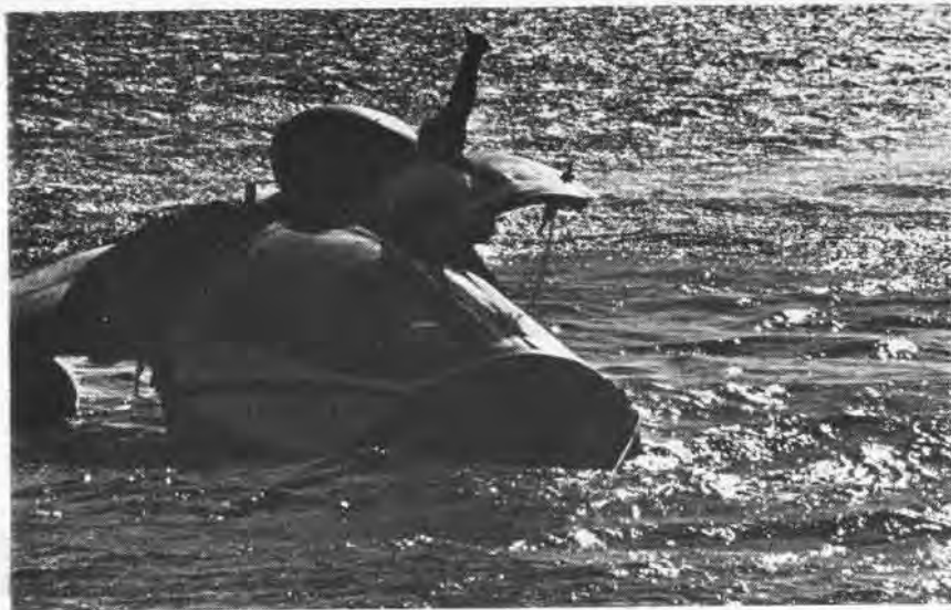
Extensive testing (left) and first emergency use of module (above after recovery) has proven survival capabilities. Automatic underwater escape is provided. If aircraft enters water, cockpit is severed, rises to surface, floats upright, insures safety from sharks.
