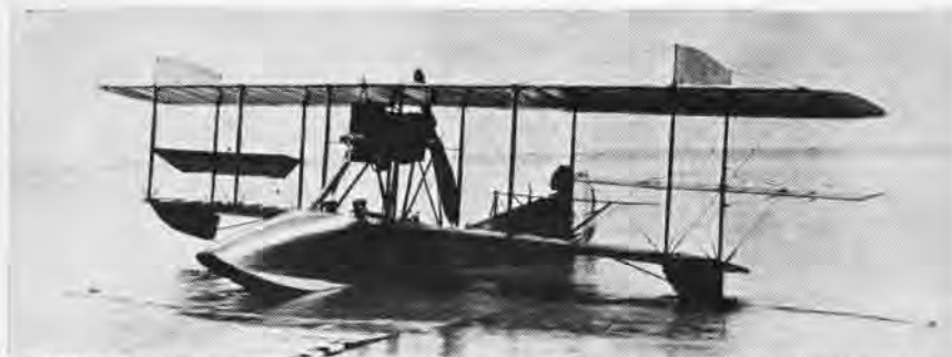
CURTISS F BOAT, THE TYPE IN WHICH THE UNIT WAS TRAINED AT BUFFALO, N. Y.
