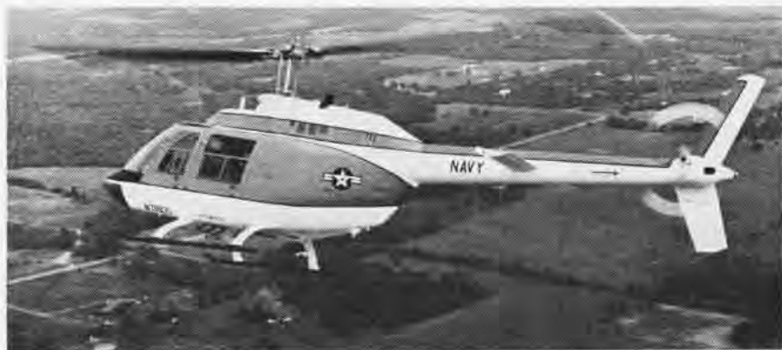
THE FIRST U.S. Navy TH-57A makes its maiden flight at Textron's Bell Helicopter Company facilities in Fort Worth, Texas. The Bell 206A JetRanger was selected as the Navy's primary light turbine training helicopter. Forty of the trainers are to be used by the Naval Air Training Command at Pensacola, Fla., succeeding a fleet of 36 Bell TH-13M's. The TH-57A is powered by an Allison 250-C18 turbine engine. Deliveries are scheduled to be made later this year.
