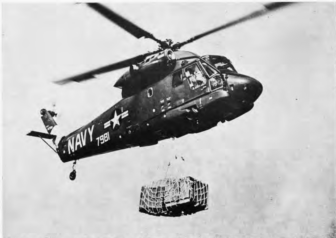
KAMAN'S UH-2C Seasprite utility and rescue helicopter has been delivered to the U.S. Navy and deployed to Southeast Asia aboard Kitty Hawk. A retrofit of the Navy's single-engine UH-2A and B models, the new twin-engine design provides for greater performance by the helo.
