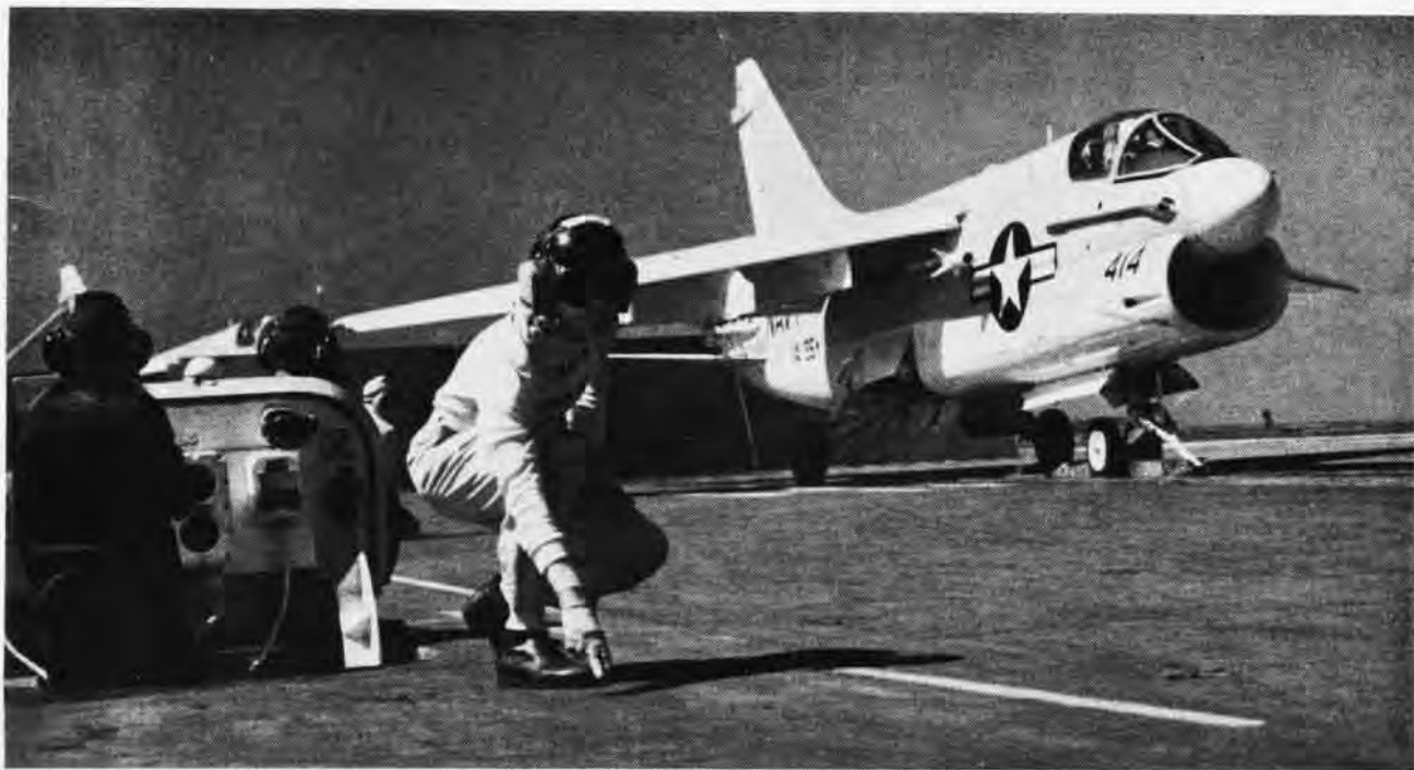
The very picture of action, Lt. Robert C. Leslie, bow catapult officer, signals launch of an A-7A from USS America. Below, with CVW-6 aircraft spotted on the catapult, USS America turns into the wind to launch her aircraft during a period of refresher training in the Caribbean.
