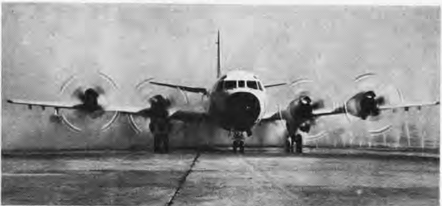
ORION TRIPS the shower mechanism, taxis through spray-down unit and comes out clean. There are 60 nozzles spraying 1,000 gallons of fresh water a minute; the operation is fully automatic. The new $25,000, aircraft rinse-down facility has been installed at Jacksonville.
