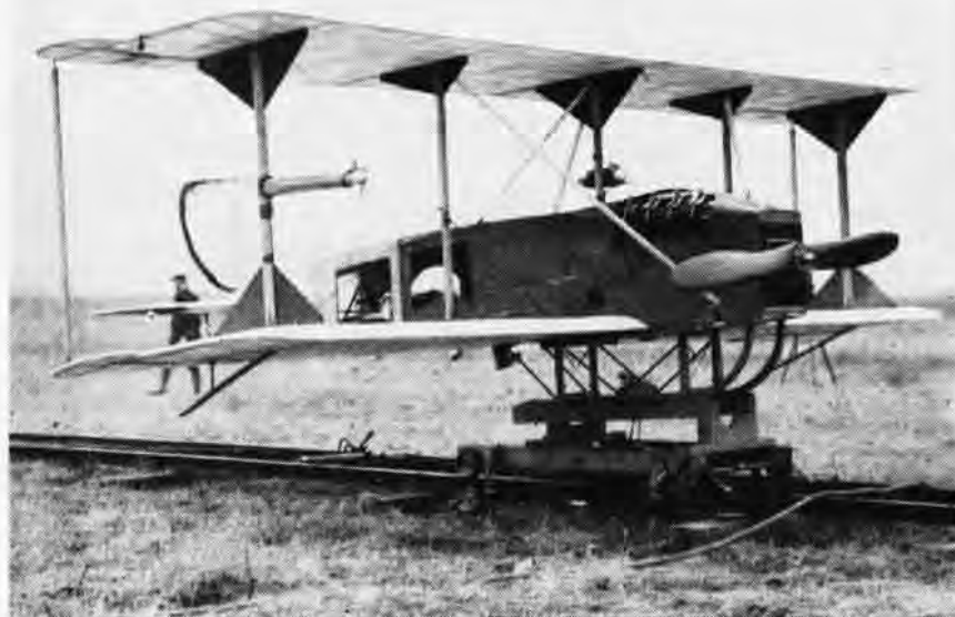
A CURTISS-SPERRY FLYING BOMB IS SHOWN HERE MOUNTED FOR A CATAPULT LAUNCH
