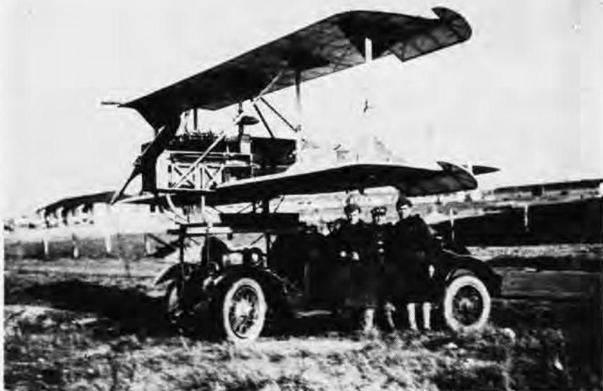
AN AUTOMOBILE IS SUBSTITUTED FOR A WIND TUNNEL IN A TEST OF A FLYING BOMB
