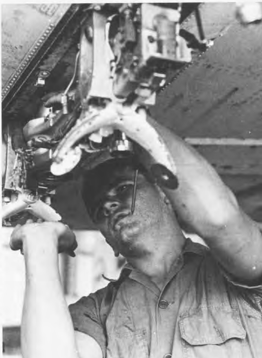
ORDNANCEMAN Cpl. Bryan Roache checks a bomb release electrical circuit.
