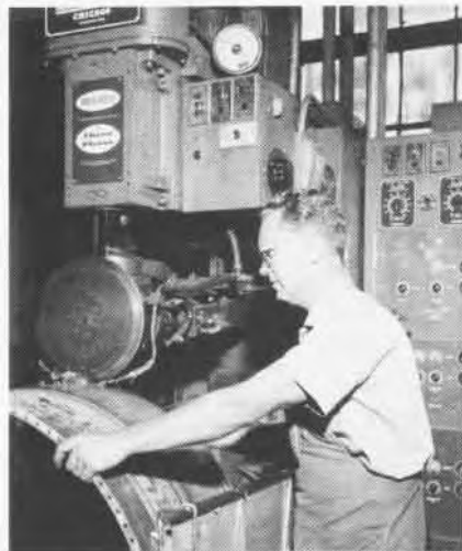
AT NORTH ISLAND'S Naval Air Rework Facility, F. W. West (left) operates a plasma needle arc welder to repair eroded areas of J-57 vanes. Above left, W. W. Kissell uses an automatic TIG welder to work on front duct assembly of a J-57 afterburner combustion chamber. Above right, Gordon Hayes operates a resistance seam welder to attach a reinforcing band to an afterburner duct, just before a new end is spliced on the afterburner.
