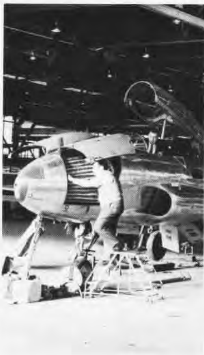
ONE OF the technicians at NADC evaluates sonar components (left). The nose cone of a QT-33 pilotless drone is replaced (center). Above, a systems analyst programs a patchboard to install in an analog computer.
