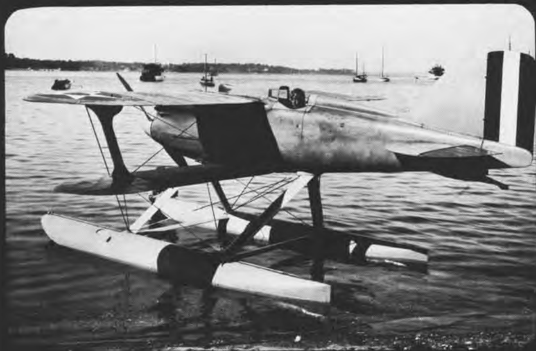
Curtiss R3C-2 flown by Lt. Ralph Ofstie, above, was one of two Navy entries in 1925 Schneider at Bay Shore Park, Md. The R3C-2's were powered by 565 hp. Curtiss V-1400 engines. Both Navy planes dropped out of the race prior to the finish, but Army Lt. Jimmy Doolittle went on to win (setting four new records in his R3C 2). It was the last American victory in international speed competition. England eventually won the trophy outright.
