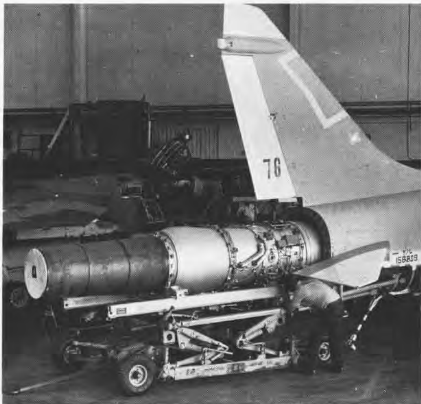
PRODUCTION models of the Navy's A-7E Corsair II's are coming off the assembly line at LTV equipped with the new Allison TF-41-A-2 turbofan engine which delivers 15,000 lbs. of thrust.
