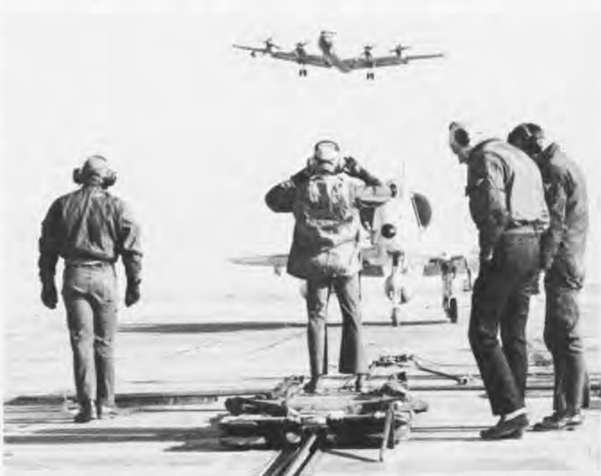
IGNORING THE ILLS commonly associated with the day, the Naval Air Test Center, Patuxent River, Md., put its SATS (Short Airfield for Tactical Support) into operation on Friday, December 13. An A-4, piloted by LCDR. Don Gerrish, was the first to be launched by the ground catapult which is part of the portable launch and recovery setup. SATS is a complete airfield that can be transported by airplane, ship or truck and set up in 72 hours.
