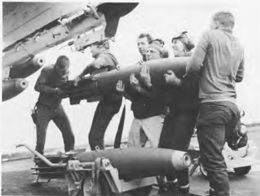
IT'S HARD WORK to arm an A-6 Intruder with a 500-pound bomb and this fact is reflected in the faces of these ordnancemen, members of Attack Squadron 165 aboard the Ranger .
