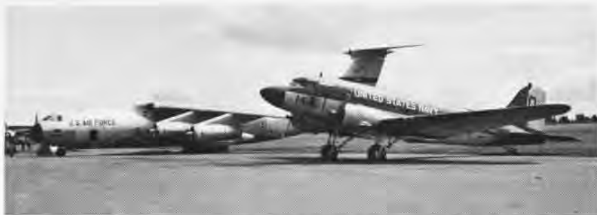
THE NEWEST , fastest transport and the oldest, slowest one used for New Zealand to Antarctic runs are shown side by side at Christchurch. The USAF C-141 Starlifter carries an average load of 40,000 pounds while the Navy's LC-47 "Gooney" carries only 3,000 pounds of cargo. Whereas the Starlifter can make the trip in five hours, it takes the Gooney 15 hours. This February the Antarctic pioneer LC-47 will leave VX-6 after 13-1/2 years of service.
