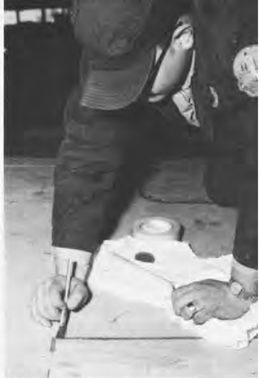
A MEMBER of VP-8, AN Eugene S. Biswick, applies sealant to the wing leading edges to keep out deterioration effects of corrosion.
