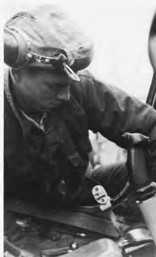
The plane captain and his crew thoroughly check out the A-6A after a flight. Here plane captain places pins in ejection seat for safety.
