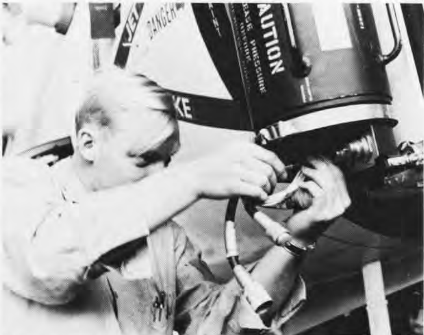
The multiple radar and related systems are the heart of the sophisticated A-6A, Intruder. Here, an AQB is removing the search radar modulator from the electronics-packed nose.
