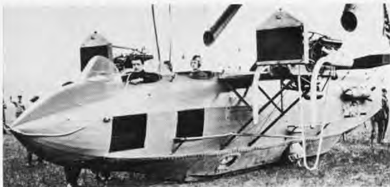
THE FOUR-MAN C-5 was a 192-foot non-rigid airship with a 40-foot control car slung beneath her. With two 125-hp engines, she had the range to fly the Atlantic.
