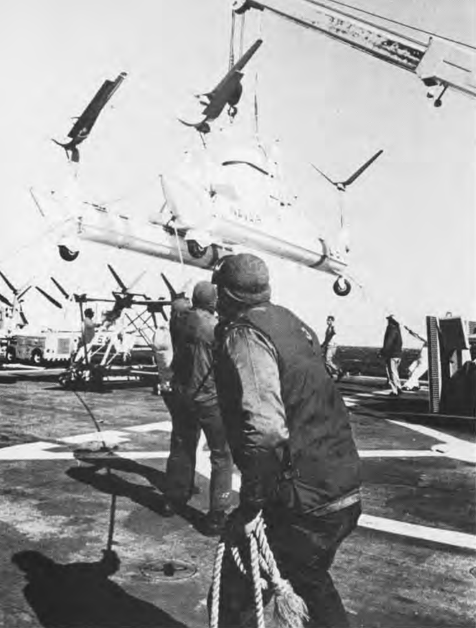
Flight deck crewmen aboard USS Raleigh hoist the Mk 105 sweep onto a cradle for preflight. When in the water, the 105's hydrofoils are lowered for greater speed.
