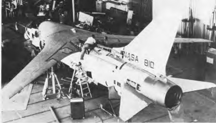
As viewed from below, the supercritical wing in flight aboard a modified F-8, opposite. Left, the thin wing is installed aboard the Crusader. The two aircraft below are Navy T-2C's. The Buckeye on the right is equipped with a thick supercritical wing.
