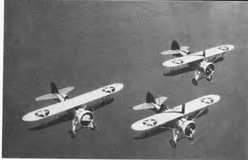
Langley-based F4B-4's of VF-3B carried two fixed, forward-firing .30 caliber guns, had a service ceiling of 27,000 feet and a maximum speed of 188 mph. The F4B's remained in fleet service from 1929 to 1938 and were assigned to shore stations as late as 1941.
