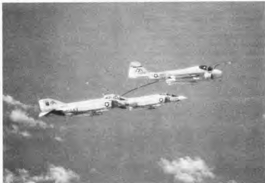
High above the Mediterranean, a KA-6D refuels two Phantoms. Navy's newest aerial gas station is deployed with VA-85 aboard Forrestal and VA-176 aboard Roosevelt . The tanker Intruder , scheduled to replace the KA-3 Skywarrior , retains all the flight characteristics of the A-6 and can transfer about 350 gallons per minute at speeds ranging from 220 to 320 knots.
