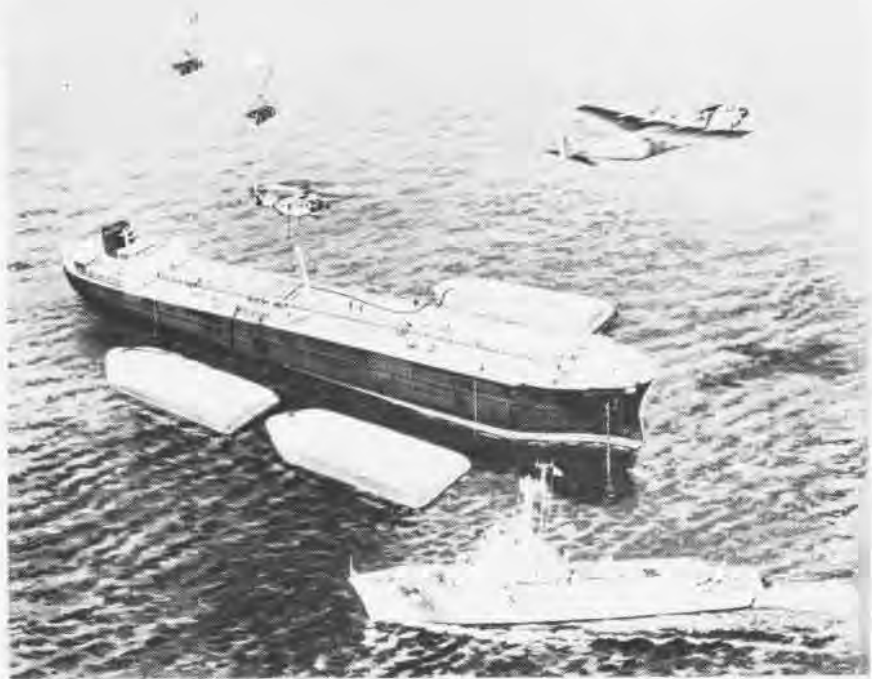
This drawing depicts the Coast Guard's air deliverable anti-pollution transfer system (ADAPTS) at the start of a mission. If a tanker goes aground, ADAPTS will eliminate the need to deliberately pump oil to lighten ship. Instead, the oil will be pumped into the large rubber containers by diesel/hydraulic submersible pumps parachuted from a Coast Guard HC-130B. A specially trained crew will be delivered to the scene by helicopter to operate the equipment.
