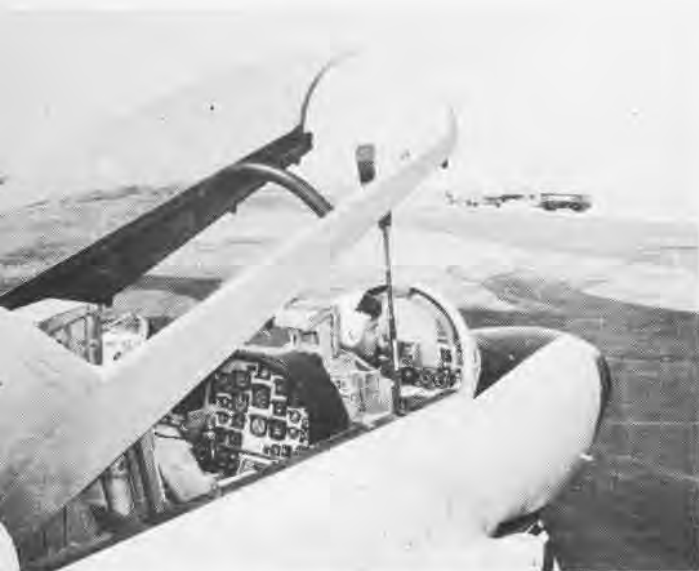
Above, Lockheed T2V modified by Douglas for flight testing the ANIP cockpit, in 1957. Rear console is standard, front is integrated panel featuring contact analog. The thin, transparent TV tube was developed by Kaiser Aircraft and Electronics Corporation. On opposite page is long-range configuration and early example of "pathway." Modern systems display considerably more information.
