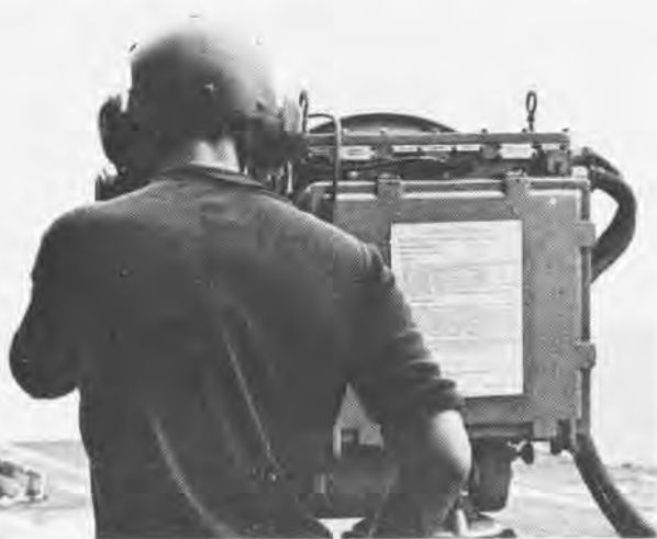
Midway Pilot Landing Aid TV (PLAT) is broadcast continuously over the PLAT control system during the daily launch and recovery period. Above, PLAT radar unit measures the speed of an incoming A-6. Information is recorded on PLAT tape and used by the LSO to guide the aircraft in.
