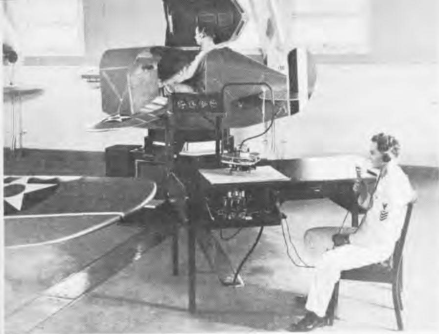
Early Link Trainer, a device regarded with mixed emotions by thousands of aviators, is shown in rare 1942 photograph. Instructor is Aviation Pilot Hoover.
