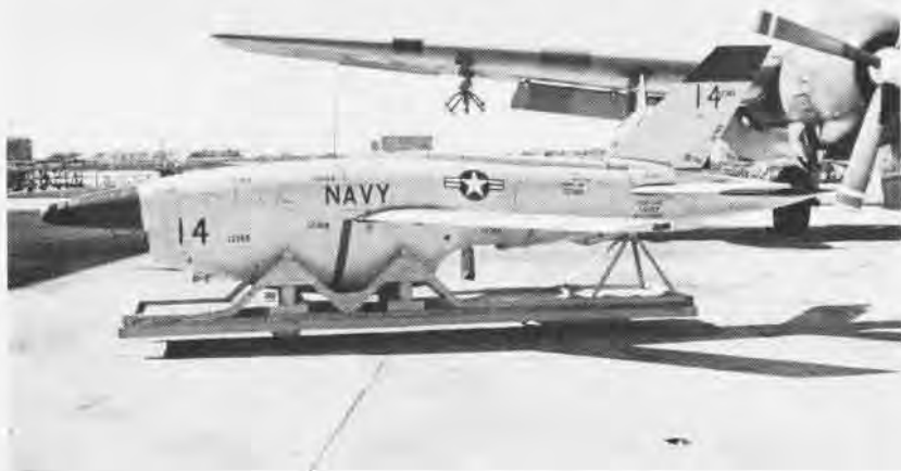
The BQM-34A Firebee provides a remotely controlled subsonic target for training and evaluation, above. An air controller gives landing instructions atop station tower, right.
