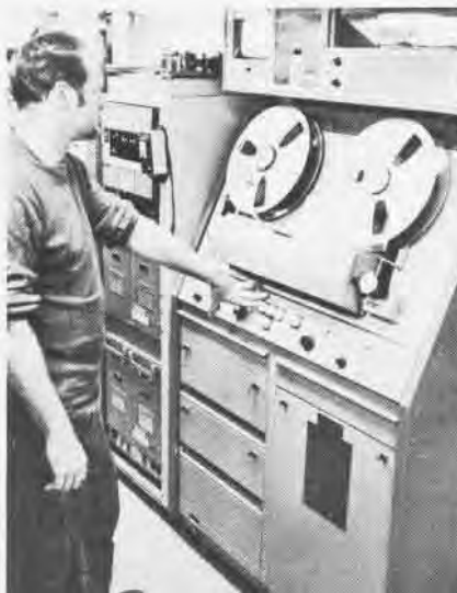
PLAT tape, left, records information from cameras, radar units, voice communications from LSO, primary flight control and carrier air traffic control. Tapes are used during debriefings and act as instant training devices. System helps to avoid/correct human mistakes and provide safer landings aboard all carriers.
