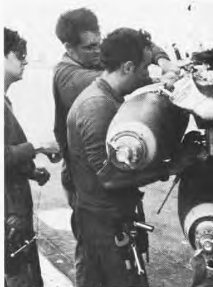
A-7E's first combat deployment proved capability of sophisticated plane. AO3 Larry Axtell, left, installs safety pin in Sidewinder launcher to prevent premature firing. AO3's Tom Valentin and Dick Osborne and AO2 Jim Bechtold, above, install arming wires on bombs. Below, AO1 Dan Miller feeds ammo into cannon as crew loads 830-lb. bomb.
