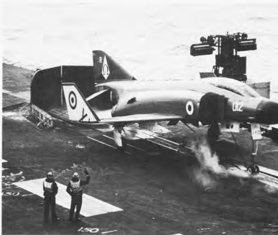
Third Ark Royal, above, saw service in many battles during World War II. Below, an F-4K Phantom, in afterburner, on waist catapult for trials of water-cooled jet blast deflector and deck cooling panels.
