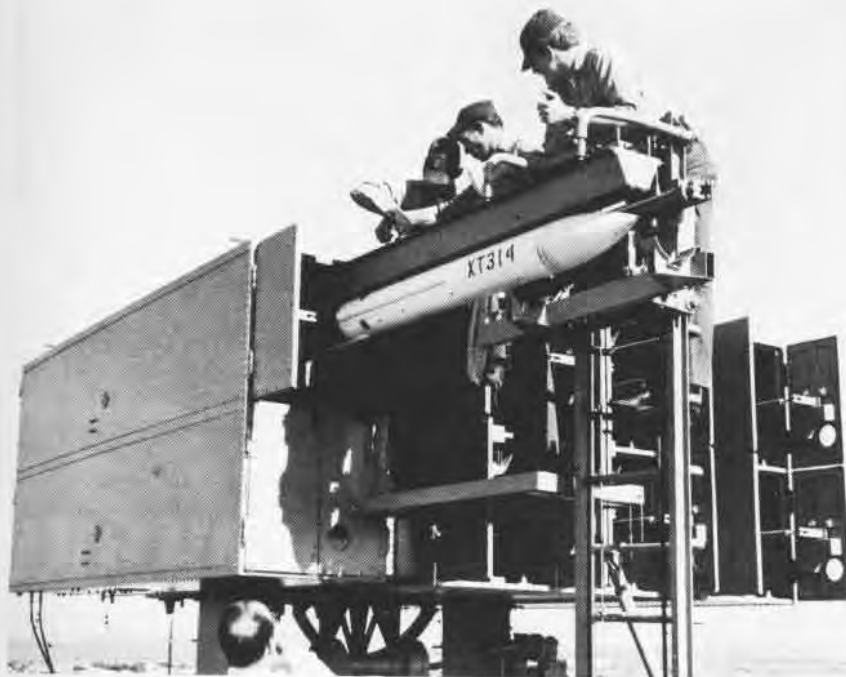
Gunner's mates install test missiles in USS Okinawa's missile launcher, left and above. Below, fire control technician operates the director illuminator during tests.
