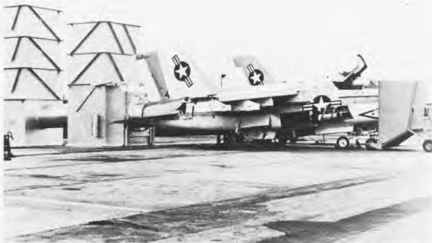
A jet engine sound suppressor, recently installed at the Naval Air Rework Facility at Alameda, "keeps down the noise" aboard the base during a ground run-up of a Corsair.
