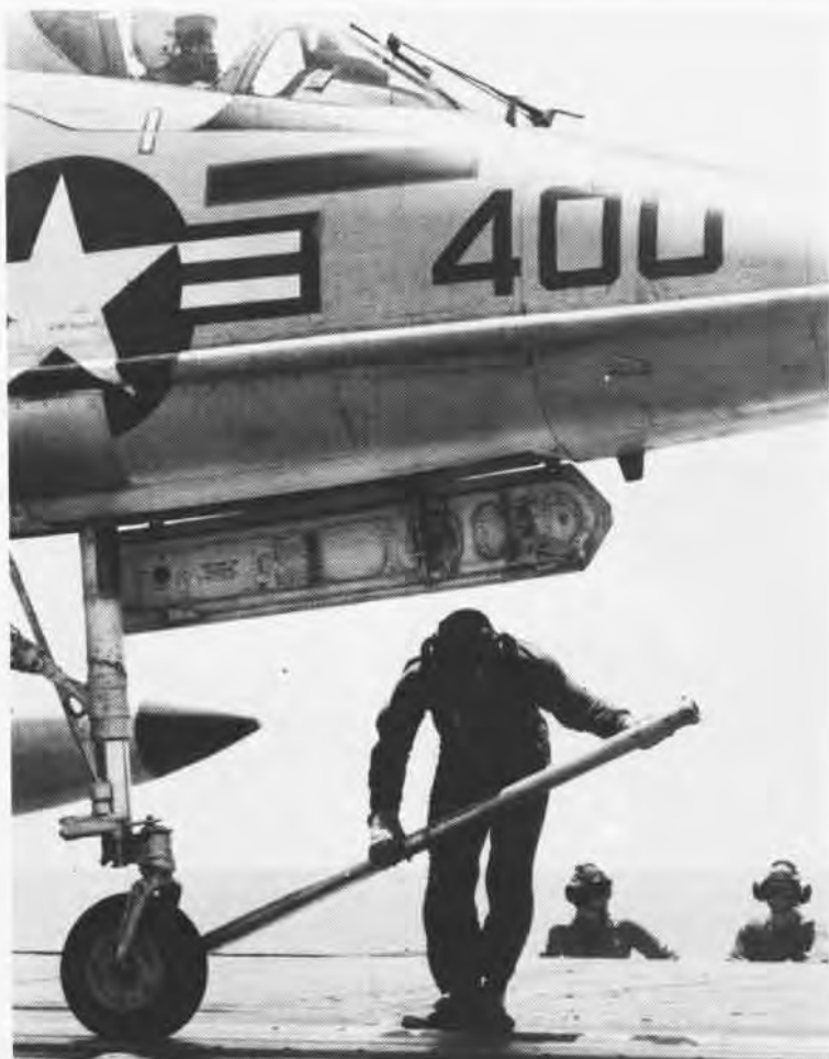
Field landing mirror systems for touch and go landings, left; rockets and pods for Huey gunships in Vietnam, top; and tiller bars to maneuver planes on a carrier bottom; are all items developed by NavAirSysCom.
