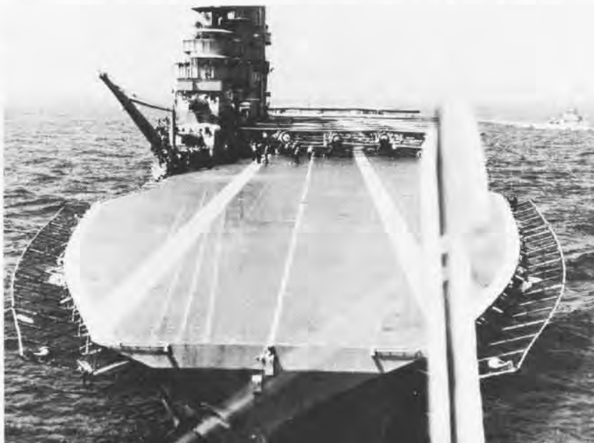
Two O3U-1 's of California 's scouting detachment are in fair-weather stowage position, above. The P-6 turntable-type powder catapult and aircraft handling equipment are well illustrated in this view. Saratoga 's forward catapult, right, was capable of speeding a 5,500-pound plane to 65 knots in a 55-foot run.
