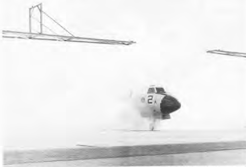
An Orion gets washed down in the new NAS Barbers Point "birdbath." The bath washes off salt spray that accumulates. An estimated $8,000 is saved in progressive aircraft rework cycle when the bath is used. It cuts down on corrosion and the necessity for repainting.
