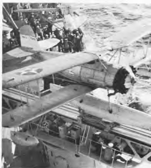
The Navy's first successful catapult launching was made at the Washington Navy Yard in November 1912. Powered by compressed air, the device launched Lt. Ellyson in a Curtiss A-3. Later models of the compressed air catapult were installed in Langley and aboard battleships and cruisers, as on Arizona, opposite. At right, O2U-3 is launched by powder catapult from Pensacola. F4B-3, below, was used for first flush deck catapult tests at Philadelphia Navy Yard using hydro-pneumatic design.
