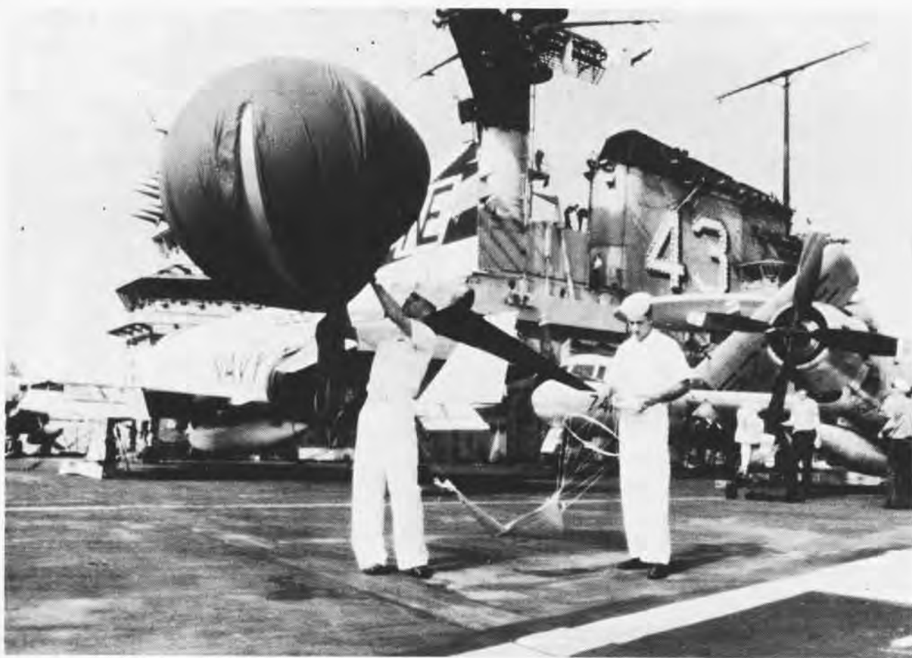
An aerographer's mate takes temperature readings in an instrument shelter for a local weather forecast at NAS Glenview, above. Below, aerographer's mates launch radiosonde from USS Coral Sea to gather upper air soundings.
