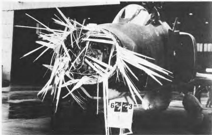
Under lab conditions, left opposite, a corona effect is achieved. Above left, time lapse photo of a lightning strike on an F-4; a simulated wing tip strike, above; left, the remains of an F-4's radome, lost to a strike.
