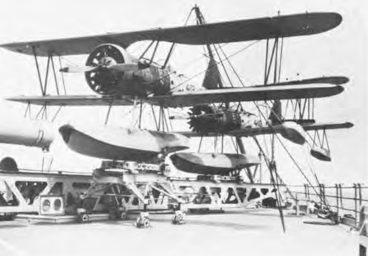
Two O3U-1 's of California 's scouting detachment are in fair-weather stowage position, above. The P-6 turntable-type powder catapult and aircraft handling equipment are well illustrated in this view. Saratoga 's forward catapult, right, was capable of speeding a 5,500-pound plane to 65 knots in a 55-foot run.
