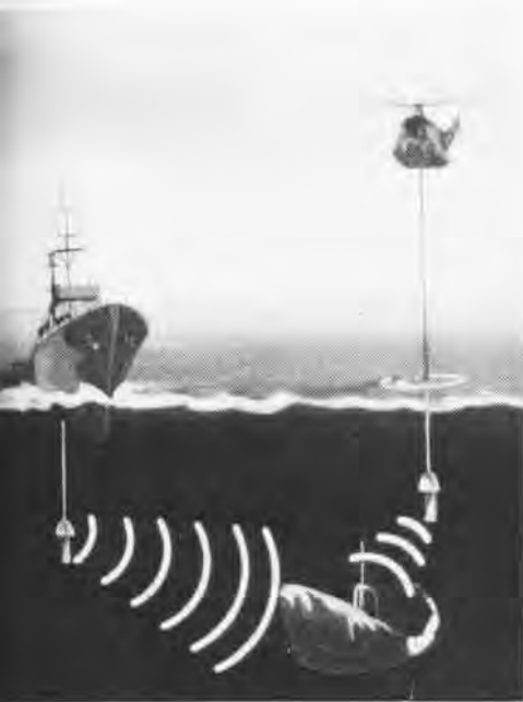
A destroyer and a helicopter use dipping sonars to hold contact on a submarine in the artist's drawing at left. The warship and the helo get valuable sonar information via the ship, helicopter acoustic range prediction. The drawing at right depicts a P-3 Orion gaining sonobuoy contact with a submarine with the help of acoustic sensor range prediction for fixed wing aircraft.
