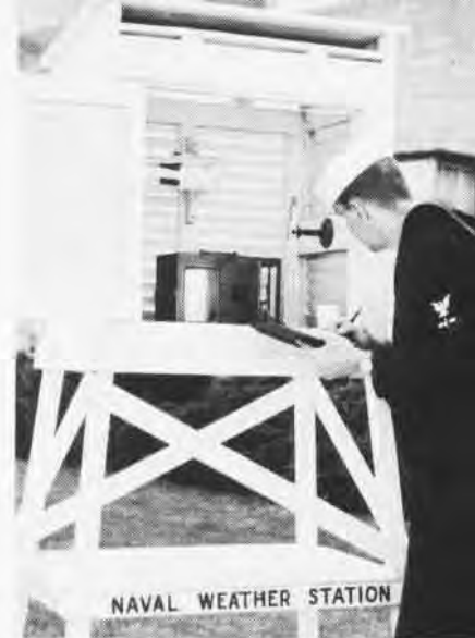
An aerographer's mate takes temperature readings in an instrument shelter for a local weather forecast at NAS Glenview, above. Below, aerographer's mates launch radiosonde from USS Coral Sea to gather upper air soundings.
