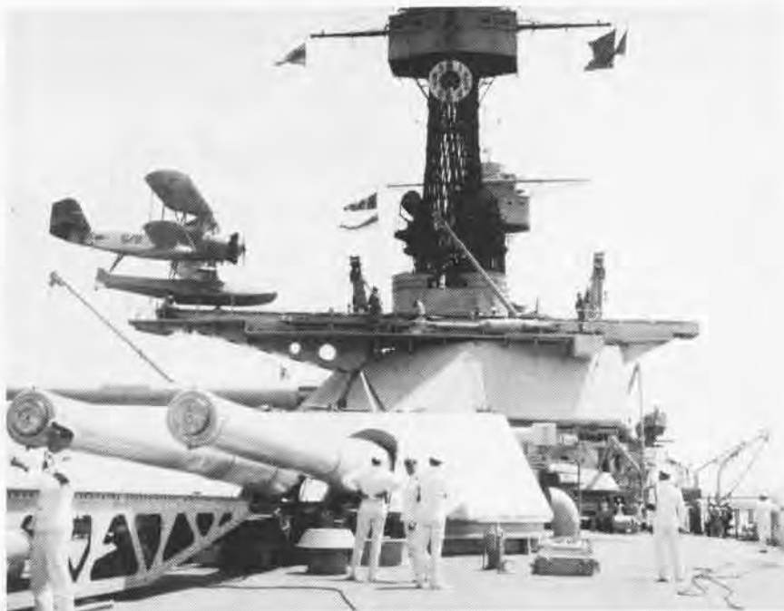
O2U prepares to launch from West Virginia in 1930, using turret-top P-4 powder catapult. An SOC , below, during a CAST recovery.
