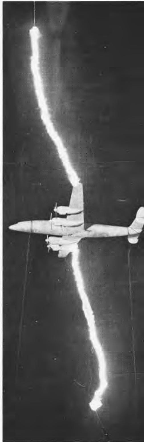
Under lab conditions, left opposite, a corona effect is achieved. Above left, time lapse photo of a lightning strike on an F-4; a simulated wing tip strike, above; left, the remains of an F-4's radome, lost to a strike.
