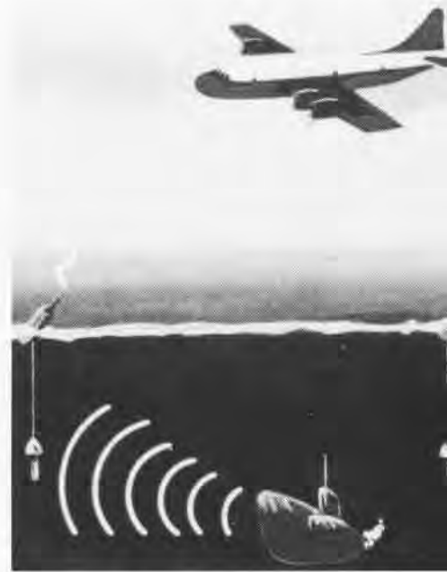
A destroyer and a helicopter use dipping sonars to hold contact on a submarine in the artist's drawing at left. The warship and the helo get valuable sonar information via the ship, helicopter acoustic range prediction. The drawing at right depicts a P-3 Orion gaining sonobuoy contact with a submarine with the help of acoustic sensor range prediction for fixed wing aircraft.
