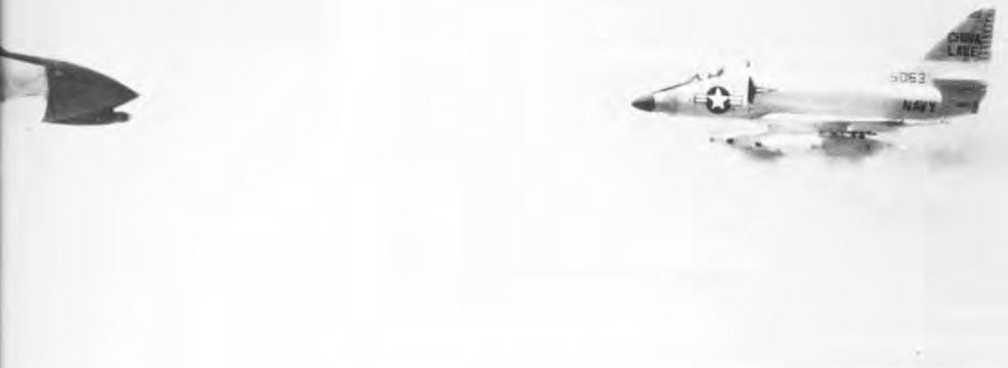
The F-48 at left launches a Sparrow missile toward an airborne target while the Skyhawk, above, demonstrates another form of air-to-air weapon, the projectile firing Mk 11 gun. Below, 900 high-explosive armor-piercing rounds can be fired from the A-4's three Mk 4 gun pods in a little over 4 seconds.
