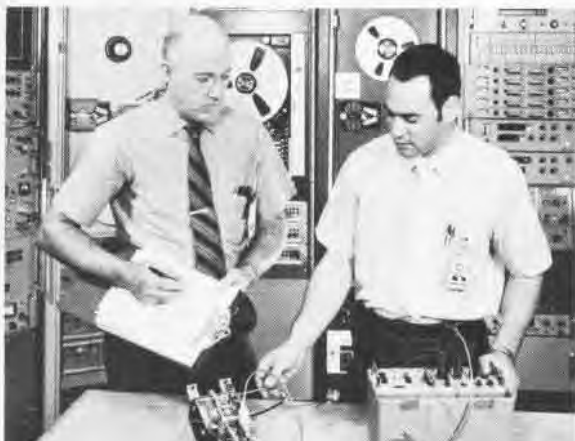
Inside of the mobile telemetry ground station during operations, left. Above, flight line test of missile is made prior to aircraft takeoff. The mobile van houses a telemetry ground station. Telemetry pack is tested before flight.
