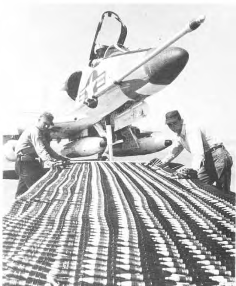
The F-48 at left launches a Sparrow missile toward an airborne target while the Skyhawk, above, demonstrates another form of air-to-air weapon, the projectile firing Mk 11 gun. Below, 900 high-explosive armor-piercing rounds can be fired from the A-4's three Mk 4 gun pods in a little over 4 seconds.
