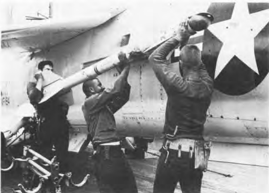
Missiles of the Sidewinder family are displayed at top, top to bottom: AIM-9B, AIM-9D and AIM-9C. Crusader of VF-194, center, sends a Sidewinder streaking toward its target. Ordnancemen aboard Ticonderoga load a Sidewinder on an F-8.
