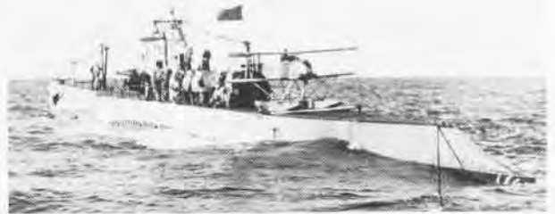
Tiny MS-1, tested as a submarine-borne scout plane, had eighteen-foot wing span and was stowed in sealed chamber on the deck.
