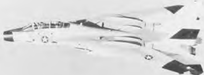
The F-14 Tomcat, Navy's newest fighter, fully "tucked" its wings for the first time in a test flight at Grumman on September 2. Its ability to sweep its wings extends its range and permits it to operate at peak efficiency at all altitudes and at all speeds.
