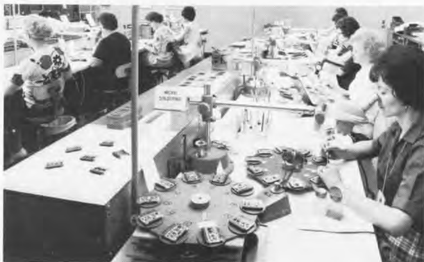
The outside diameter of an 18-foot ram, a component of the Mark 7 arresting engine, is ground at NAEC Philadelphia, right. NAFI workers solder micro standard hardware modules used in the standard hardware program, below. The modules are used in missile, ASW and telemetry systems. Jumpers at the Naval Aerospace Recovery Facility, El Centro, test parachutes, bottom.
