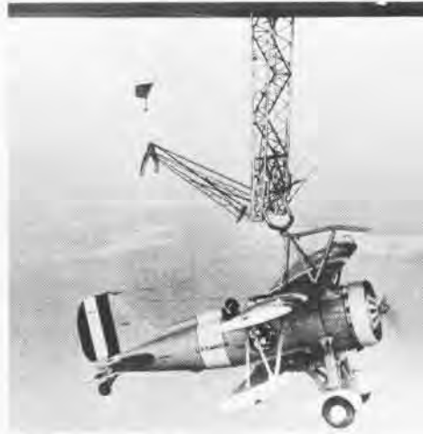
HTA detachment's acrobat insignia is visible on F9C hanging from Macon's trapeze.
