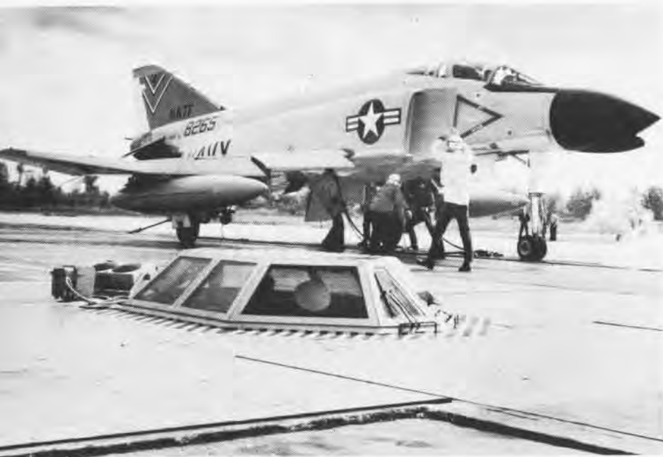
Personnel at NATF Lakehurst hook a bridle to an F-4 in preparation for a catapult test, above. Note the integrated catapult control station in the foreground. A similar station, with the monitor control console, below, will be installed in the carrier Nimitz.
