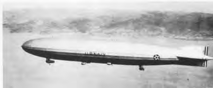
ZR-1 pioneered at-sea airship operations from Patoka , a tanker converted to an airship tender. Her design was essentially that of the early German naval airships downed in England during WW I.
