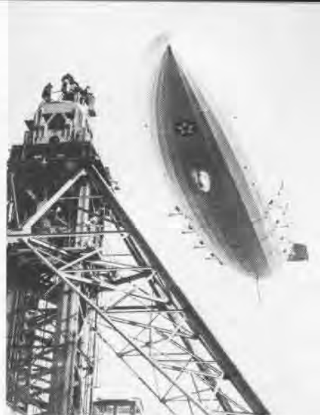
ZR-5 approaches NAS Moffett Field's mooring mast, as mooring crew handles a line dropped from the airship's bow hatch.
