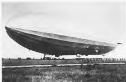
Ill-fated R-38, scheduled to enter the U.S. naval service as ZR-2, broke in half on its final test flight and plunged burning into the Humber River at Hull, England.
