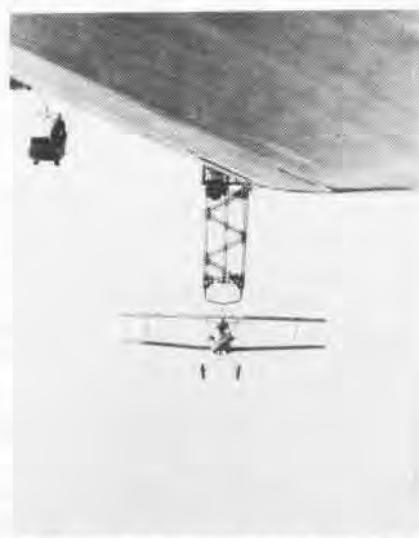
Flying an N2Y, Navy pilots work out hook-on techniques and refine equipment, using Los Angeles's experimental trapeze device.
