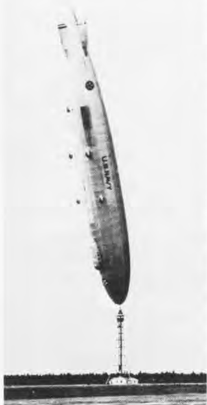
Caught in a sudden but gentle wind, USS Los Angeles stood on her nose in 1926, rotating 180 degrees around her mooring mast.
