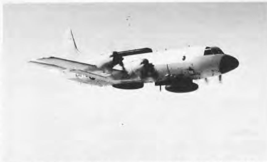
Prototype of Navy's newest Orion features a large canoe radar on top and bottom of the aircraft and a ventral radome. Lockheed is converting ten P-3A's and two EP-3B's to the ECM EP-3E configuration. Total delivery of the new aircraft to VQ's 1 and 2 is scheduled for July 1972.
