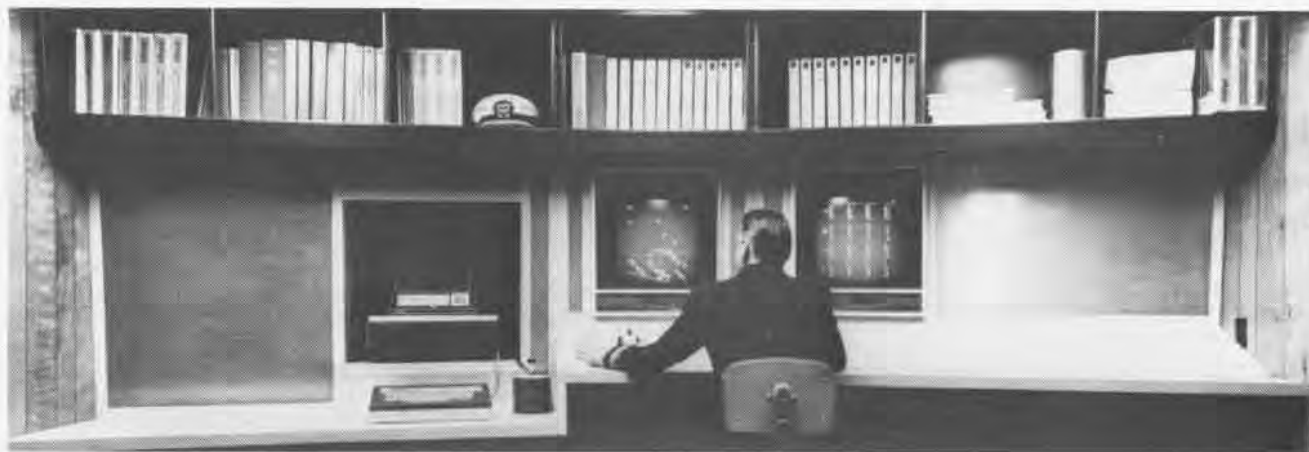
The display console, below, includes these three panels. Panel at left provides the data on simulated firings. Triangles on 3D real-time screen are mountain tops. At right is safety data.
