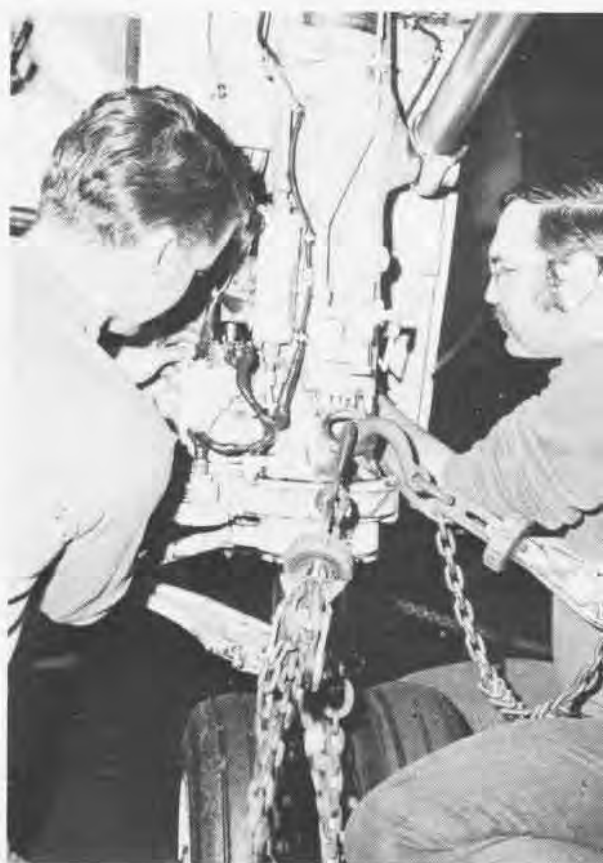
VF-96 Project SAMIE coordinator, AMST O. J. Jordan, completes the phase two maintenance sequence chart for the squadron F-4J's, opposite top. ADCS D.C. Black guides a J79-GE-10 engine toward an F-4J for installation after a 600-hour inspection, left. AE3's K.S. Beck (L) and S.R. Harrison work on an F-4's approach lights.
