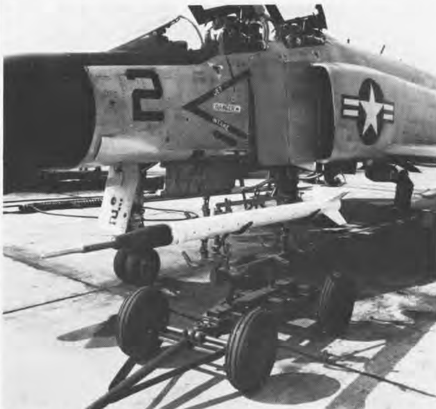
Airborne pod subsystem resembles a Sidewinder and is mounted on the aircraft in same manner.
