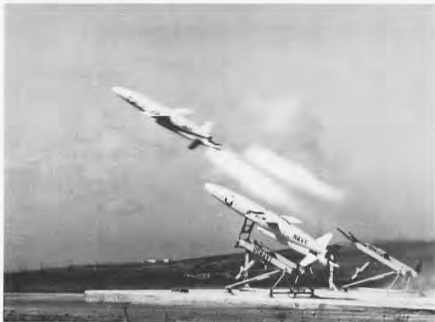
Trailing JATO tails, MQM-74A Chukar drone leaves the stand for a flight, above. At right, Air Force F-100 paces a Firebee I .
