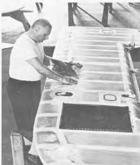
Painstaking effort goes into each restoration at Silver Hill. Here, wing of F9C has doped finish on fabric covering sanded down during repairs.
