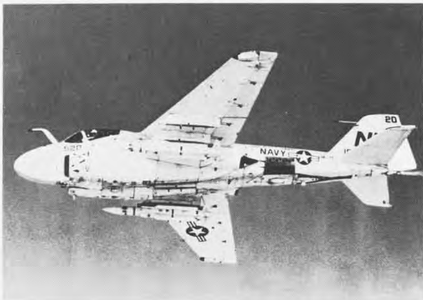
Condor missile is tested against trailer-mounted radar at desert test site, above, with dramatic results. VA-75 Intruder from Kitty Hawk , below, carries two Standard ARM missiles while on a tactical flight over SEAsia.
