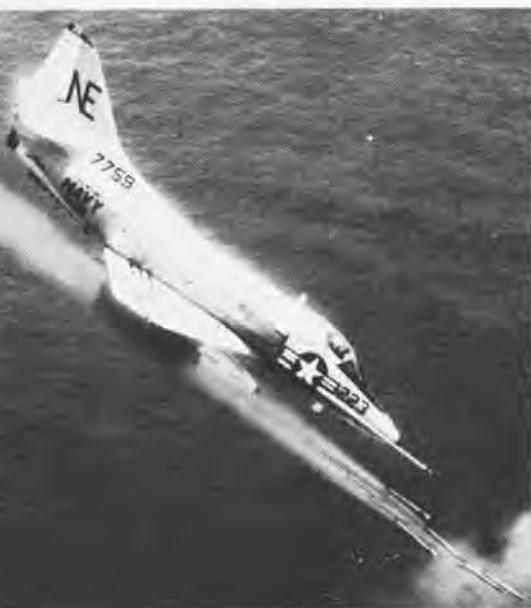
Close-up of the 2.75" FFAR 19-place rocket launcher illustrates striking power available to attack aircraft. A-4, below, launches FFAR's during WestPac deployment.
