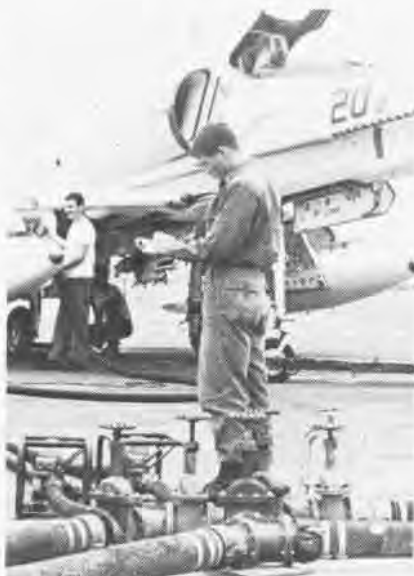
The fuel level in a 10,000-gallon holding tank is checked, top right. Marine monitors fuel quantity gauge as a VMA-211 Skyhawk refuels at the pits, above. Right, TAFDS OinC checks out fuel filter for the system.
