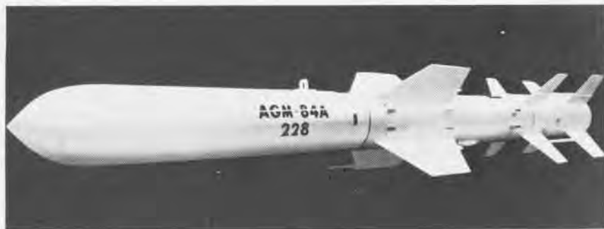
Condor is designed to attack high value targets that lie in heavily defended areas, homing automatically or under remote guidance.
