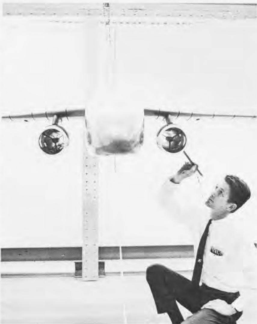
Vought engineers work on S-3A Viking's aft body and tail, opposite left. Photo at opposite right top shows fuselage assembled in half shells to provide extra work space for installing wiring and plumbing. First S-3A nears completion, opposite right bottom. Model of S-3A is prepared for wind-tunnel flutter testing, above. Cutaway at left shows interior arrangement.
