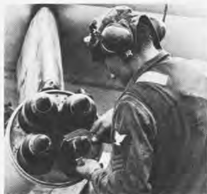
VA-25 ordnanceman checks Zuni rockets in wing-mounted pod aboard Coral Sea prior to tactical mission assigned by Seventh Fleet.
