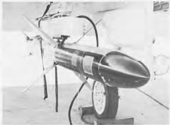
Shrike anti-electronic-radiation missile homes on a wide variety of frequencies to carry out its mission against enemy air defenses.
