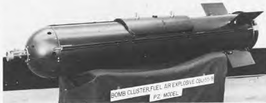
CBU-55 releases fuel containers which disburse explosive clouds, clearing hazards to helicopter landings. Walleye , right, homes, directed by self-contained TV guidance, on its objective.
