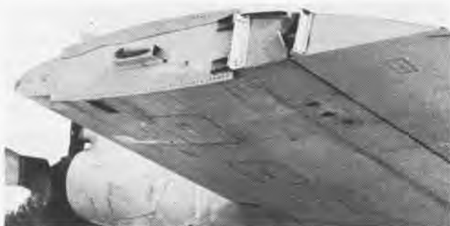
These photographs are before and after shots of the same P-3B. The Orion lost eight feet of wing and damaged a vertical stabilizer in a midair collision. Wing was capped for the flight home.
