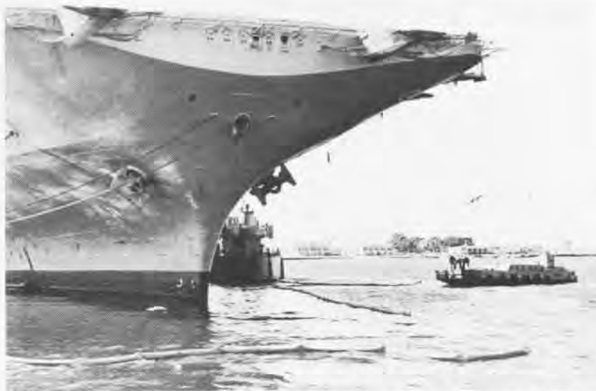
A floating device of plastic-coated nylon, eight inches in diameter, is maneuvered into place around USS Oriskany (CVA-34) during tests at NAS North Island. Manufactured in sections that can be joined to surround any size ship, an 18-inch curtain, counterweighted by 1/4-inch chain, extends below the surface to keep spilled oil from sliding underneath. In choppy water, additional rings can be placed outside of the original ring to catch any oil overflow.
