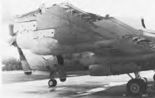
These photographs are before and after shots of the same P-3B. The Orion lost eight feet of wing and damaged a vertical stabilizer in a midair collision. Wing was capped for the flight home.
