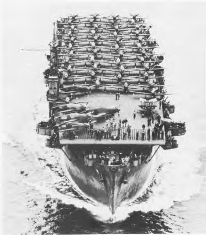
Altamaha heads for India with badly needed P-51's stacked on her flight and hangar decks. The 450-foot flight deck normally accommodated 12 fighters and 9 torpedo bombers.
