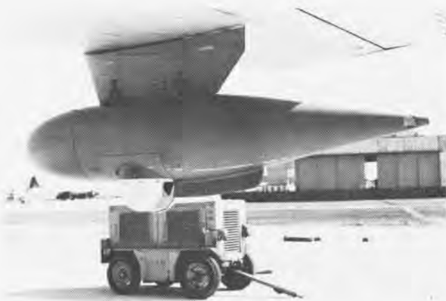
Fairing behind the turret on Hughes' FLIR was later replaced by a fin.
