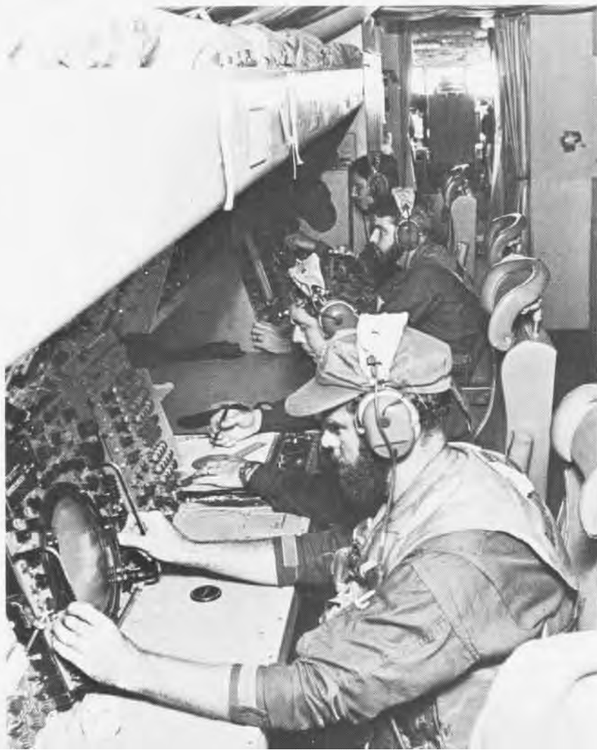
P-3C TACCO, aided by a computer, analyzes sensor data. Below, sensor operators, navigator and TACCO of a P-3A work together to solve an antisubmarine warfare problem.
