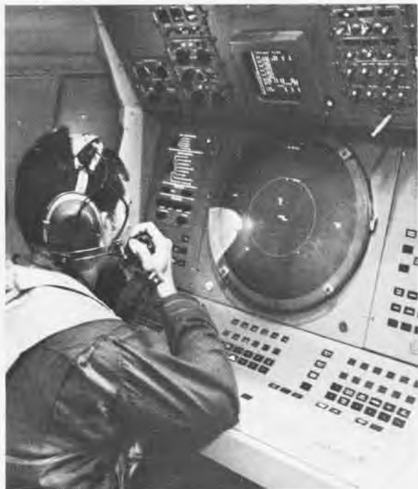
P-3C TACCO, aided by a computer, analyzes sensor data. Below, sensor operators, navigator and TACCO of a P-3A work together to solve an antisubmarine warfare problem.
