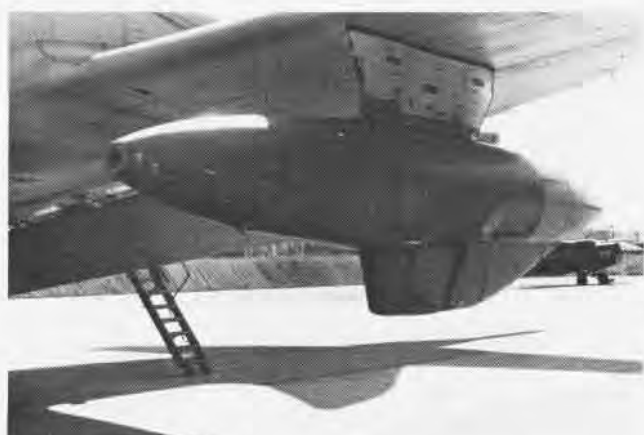
Narrow fin on Texas Instruments' FLIR increased azimuth coverage.
