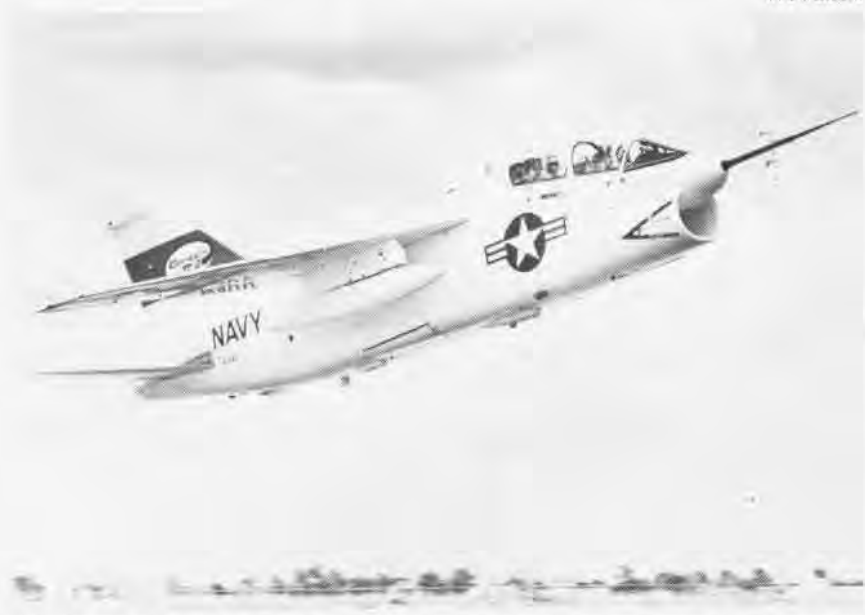
LTV's Corsair II 2 prototype made its maiden flight at NAS Dallas on August 29. The stretched version, which will accommodate two pilots or a pilot and passenger, is designed for combat crew or instrument training, or for use in combat. To make room for the second cockpit, the nose section was re-faired to just forward of the wing and stretched 16 inches. An 18-inch insert was added just aft of the wing section and the aft section was tilted up about 1.2 degrees.
