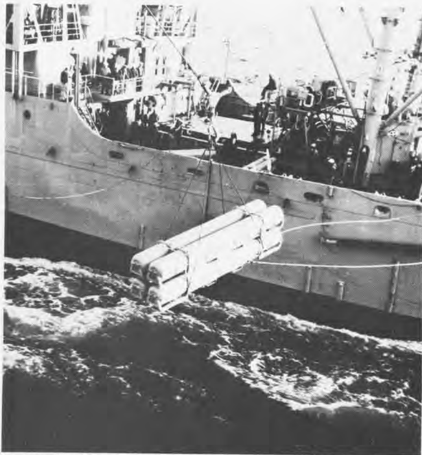
Proper container design and handling ensure safe at-sea transfer of Navy weapons. Here, four Shrike missiles are transferred from an ammunition ship to the attack carrier Midway.
