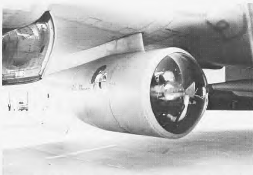
GE ALLTV pod is 46 inches in diameter, allowing increased gimbal angles for the camera.
