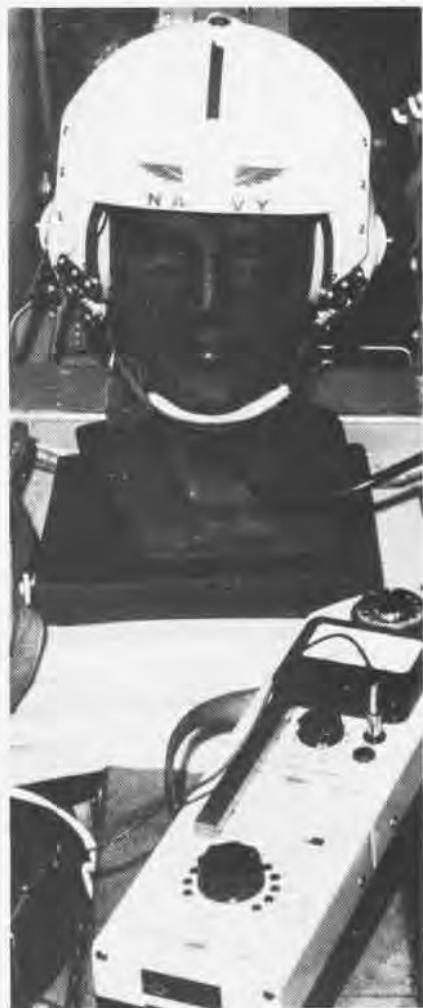
Mike the Manikin, an instrumented, portable head developed by the Acoustical Sciences Division of the Naval Aerospace Medical Research Laboratory, is used to obtain flight helmet performance data in respect to noise attenuation and speech intelligibility during actual aircraft operations.
