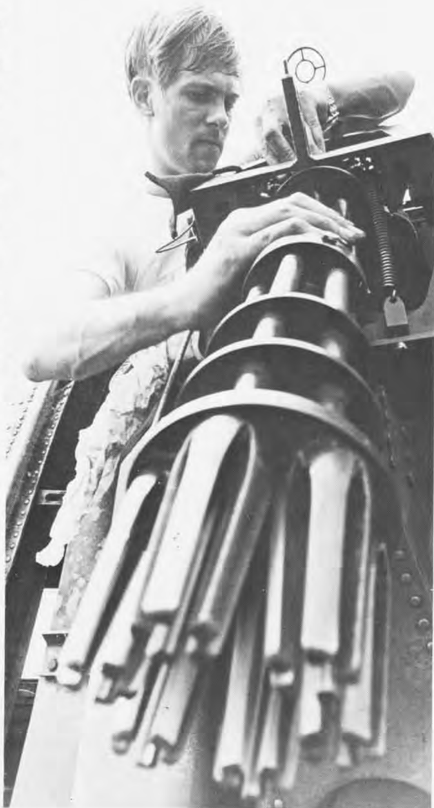
Aircrewman Mark Hoover cleans his helo's Gatling-type machine gun which is capable of firing 4,000 rounds of ammo per minute.
